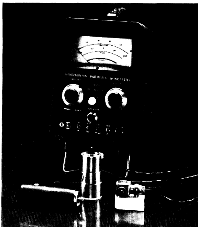
Figure 3-12. Harmonic Bond Tester With the Vibrating Pin Probe- Left Front
