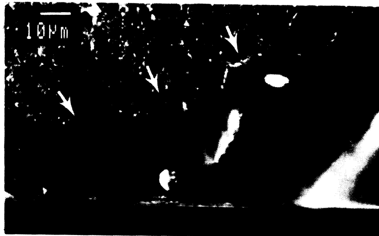
FIGURE 7. Contamination from a smear of masking tape resin (white arrows) near a chamfer. Masking tape is sometimes used to hold pieces of a fractured specimen together, but should be avoided on the fracture and tensile surfaces. The smear blends into the fracture surface and is partially transparent to X-rays as shown. An energy dispersive analysis identified the smear as having potassium, chlorine and sulphur. Trichloroethylene is an effective solvent to remove the resin.
