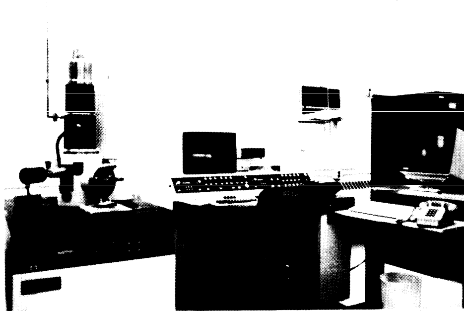
FIGURE 3. Scanning electron microscope with energy dispersive spectroscopic capabilities, low-energy operation and magnification between 20x and 20,000x.
