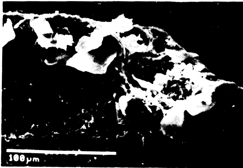
FIGURE 10. Contamination from human skin. (Courtesy of A. Pasto, GTE Laboratory, now with Oak Ridge National Laboratory).
