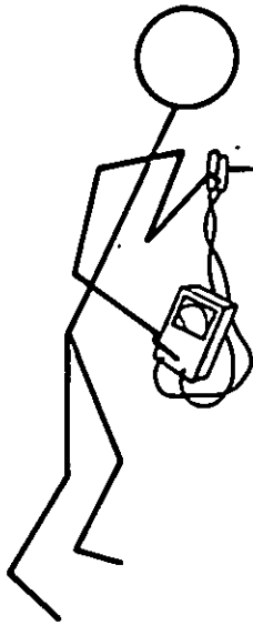
(A) Check Clip Leads for Integrity of Insulation and Compatibility With Terminals
