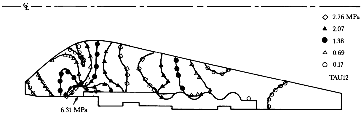
Figure 7-48. Maximum Shear Stress Contours
