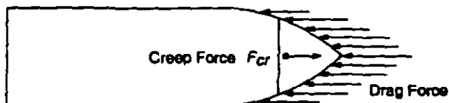
Figure 5-7. Creep Force on a Fuze Part
