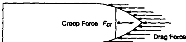
Figure 5-7. Creep Force on a Fuze Part
