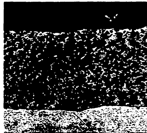
NYE-CARB® Composite Cross Section (600X Magnification)
