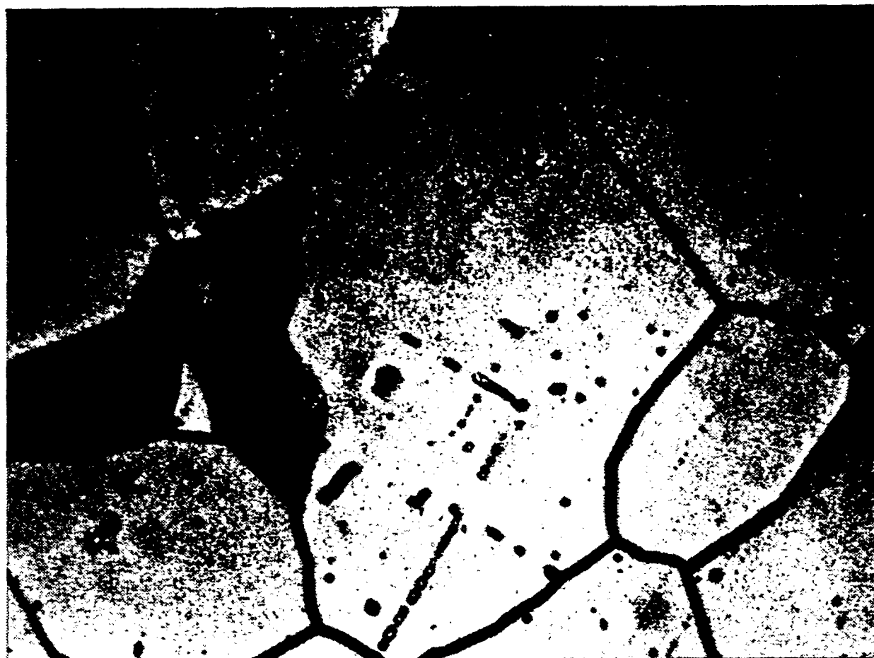
Figure 2-27. Intergranular Corrosion of Sensitized Type 316 Stainless Steel (Ref. 6)
