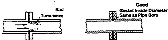
(B) Gaskets That Protrude Into the Flow Channel Cause Turbulence
