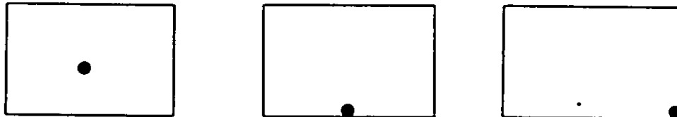
FIGURE 17. Schematic showing how a volume-distributed flaw can be located in the volume, at the surface or at an edge.
