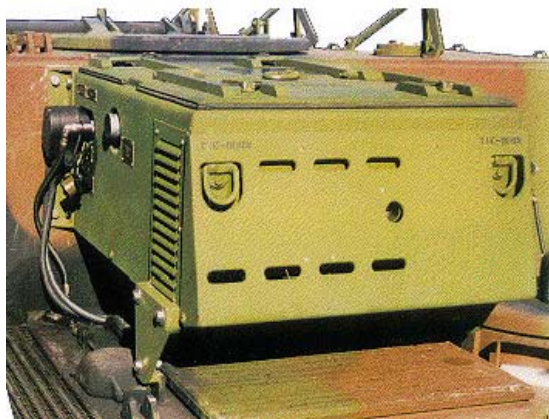
MEP-952A on M557 (Power connector side)
