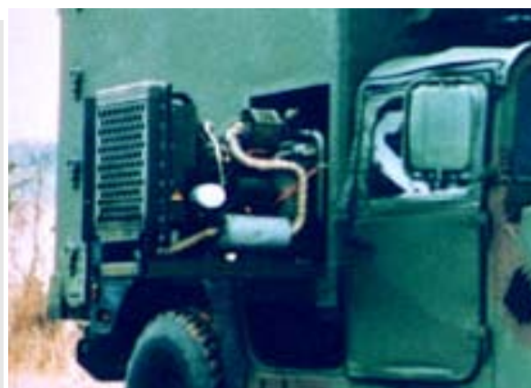
10 kW APU ready to slide into shelter. - front view -
