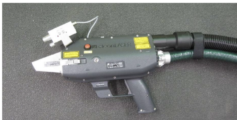
FIGURE 2: Image of a 300W Hand-Held Laser End Effector with sensor package, vacuum hose connection, and fiber optic cable connection
