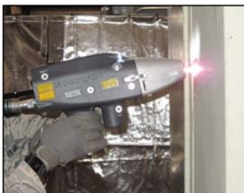
FIGURE 6: Proper end effector angle during HHL operation
