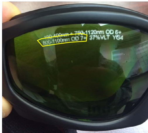
FIGURE 4. Laser eye protection rating with wavelength ranges
