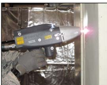
FIGURE 6: Proper end effector angle during HHL operation
