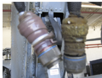
Unacceptable Self-fusing silicone tape not applied and not secured with authorized lacing tape.
