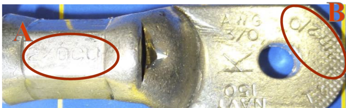
(A) Die index number embossment on completed crimp. (B) AIR Gauge marking.
