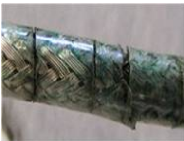
Unacceptable Radial crack in the insulation.
