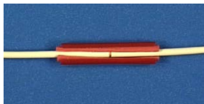
Unacceptable Exposed conductor; under-heated or under-sized.
