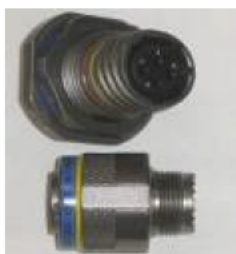
Acceptable Serviceable connector.
