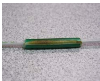
Unacceptable Mismatched adhesive and sleeve as well as over-heated installation.
