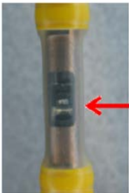
Unacceptable Conductor not visible in inspection window.
