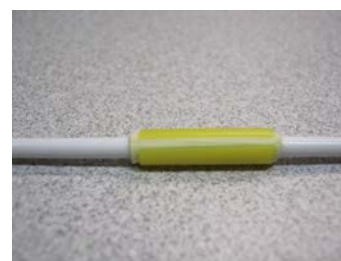
Unacceptable Under-heated/not melted.
