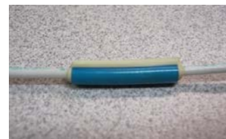
Unacceptable Adhesive/insulation mismatch.
