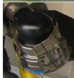
Unacceptable Plastic bag or ESD Grid Tape used to cap and stow connector.
