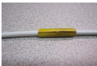
Unacceptable Over-heated installation.
