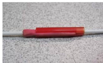
Unacceptable Misalignment adhesive and outer sleeve.
