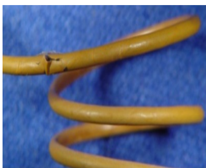
Acceptable Only outer topcoat damage. No inner polyimide insulation (brown) damage; conductor not exposed
