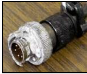
Unacceptable Connector corrosion with connector degraded until broken.
