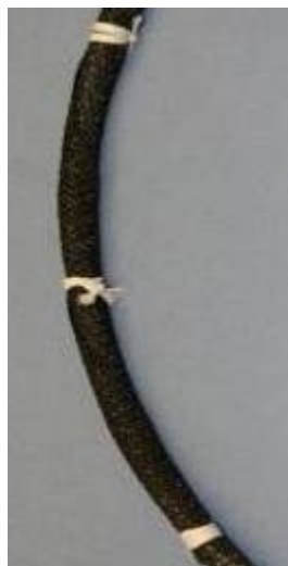
Acceptable Proper installation of harness covering.
