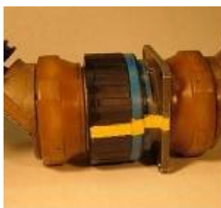
FIGURE 5-1. Example of correctly mated connectors using an indicator line and locking pin with inspection hole.
