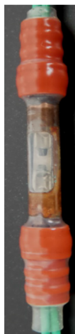
Unacceptable Evidence of corrosion inside sleeve. Multiple wires installed, both ends.
