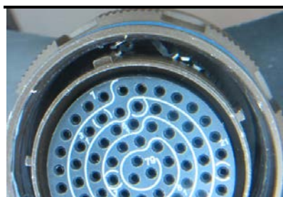
Unacceptable Multiple broken EMI seal fingers
