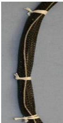
Unacceptable Improper twisting of harness covering.
