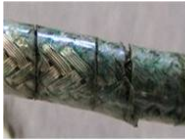
Unacceptable Radial crack in the insulation.
