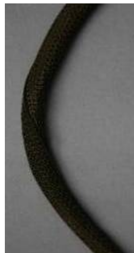
Unacceptable No spot tie on harness covering.
