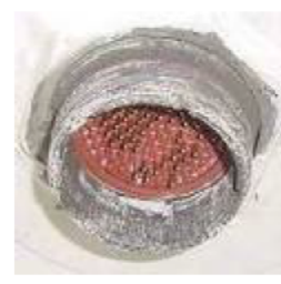
Unacceptable Another example of corrosion on a connector.
