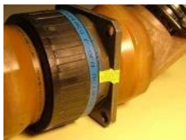
FIGURE 5-1. Example of correctly mated connectors using an indicator line and locking pin with inspection hole.
