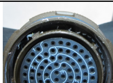
Unacceptable Missing and broken EMI seal fingers
