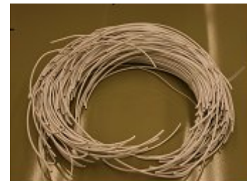
Unacceptable Wire received from supply in an unusable condition. Wire is in several short segments.
