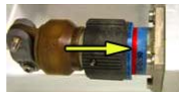
FIGURE 4-1. Example of correctly mated connectors using a red locked indicator band and locking pin with inspection hole.
