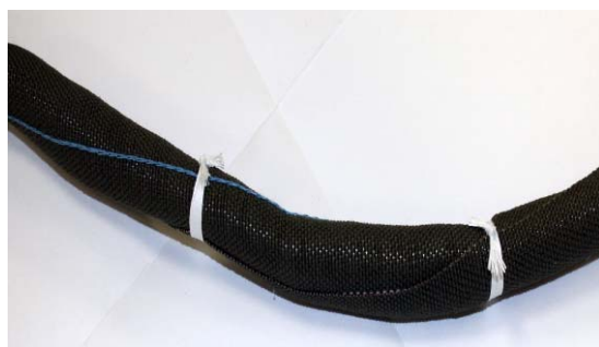
FIGURE 19-1. Illustration of EMI wraparound braid and examples of proper installation.
