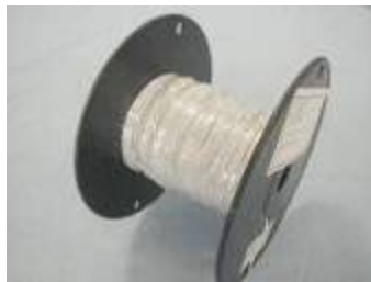
Acceptable Wire is received from supply on a spool with identification label.
