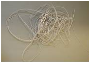
Unacceptable Wire received from supply in an unusable condition. Wire is not on a spool.
