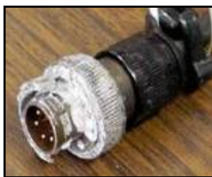
Unacceptable Connector corrosion with connector degraded until broken.
