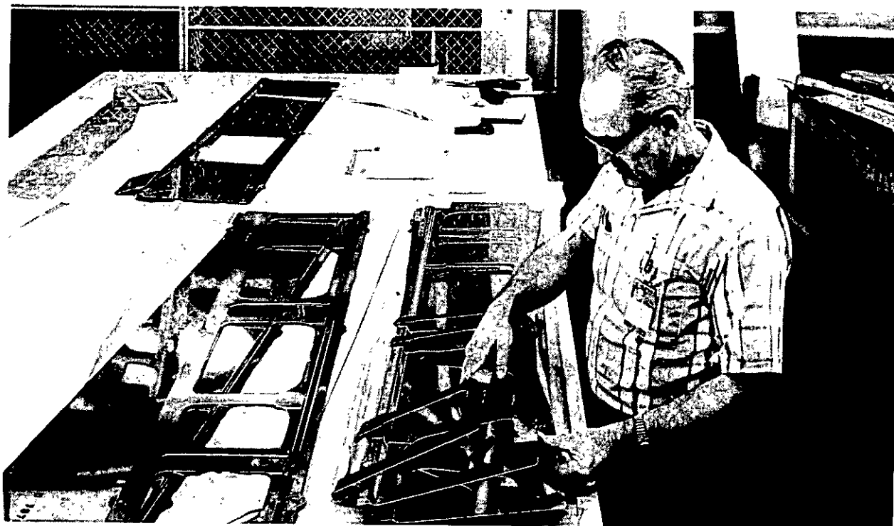
FIGURE 5.3 Prefit inspection prior to bonding.
