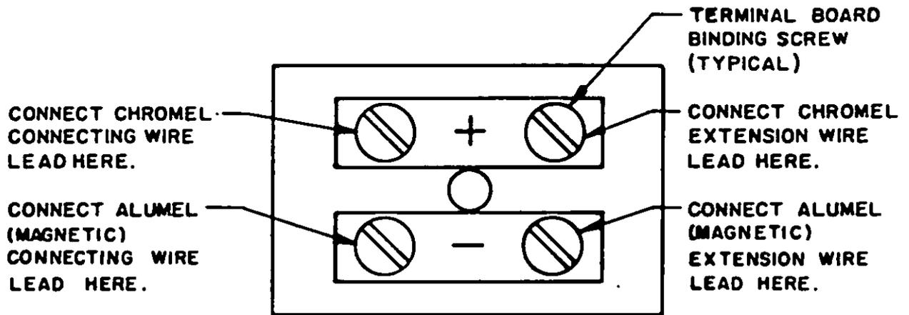
Terminal board for thermocouple sensor.
