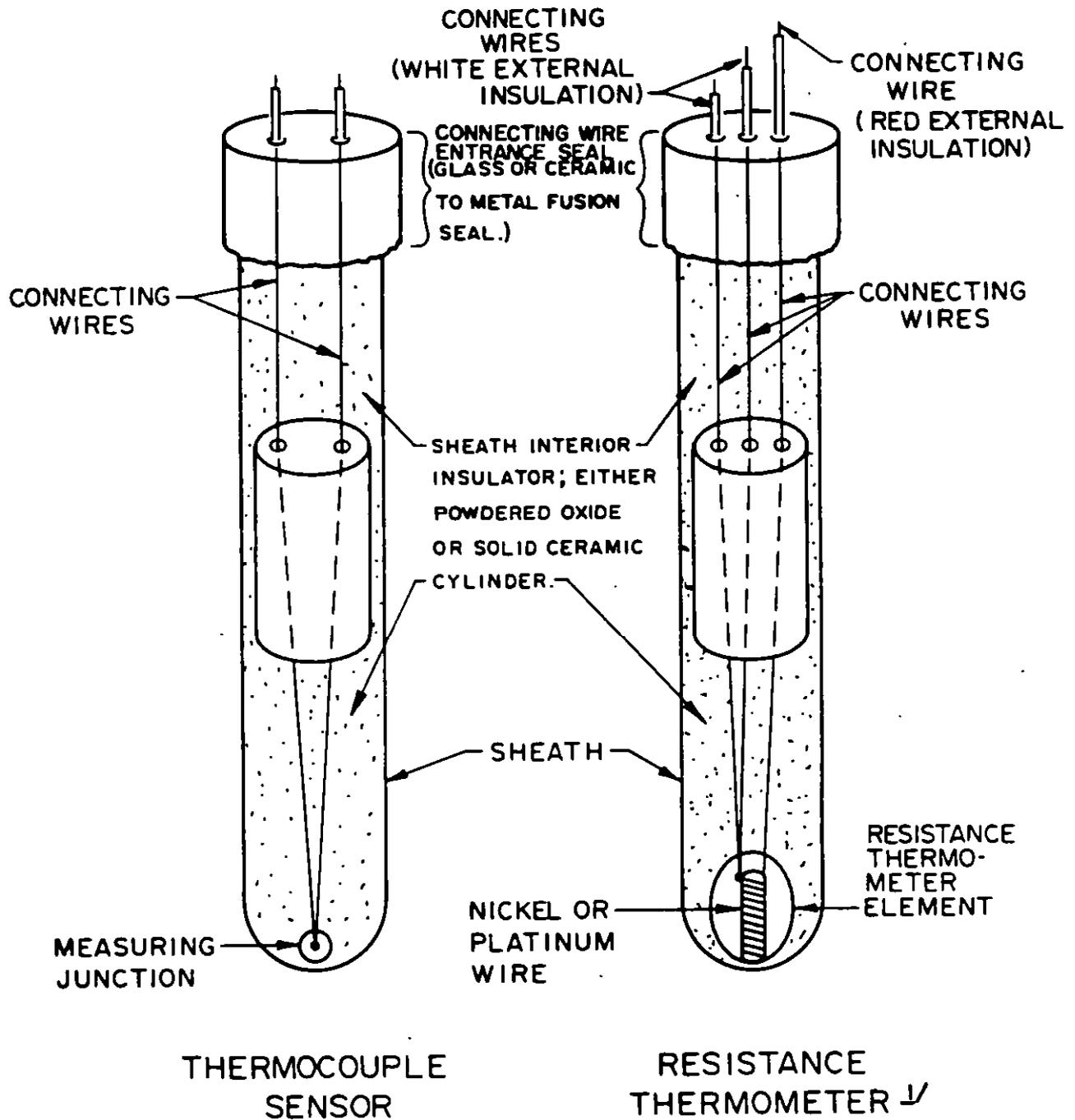
✓ For bare bulb configuration, the resistance thermometer with nickel element will have two connecting wires.
