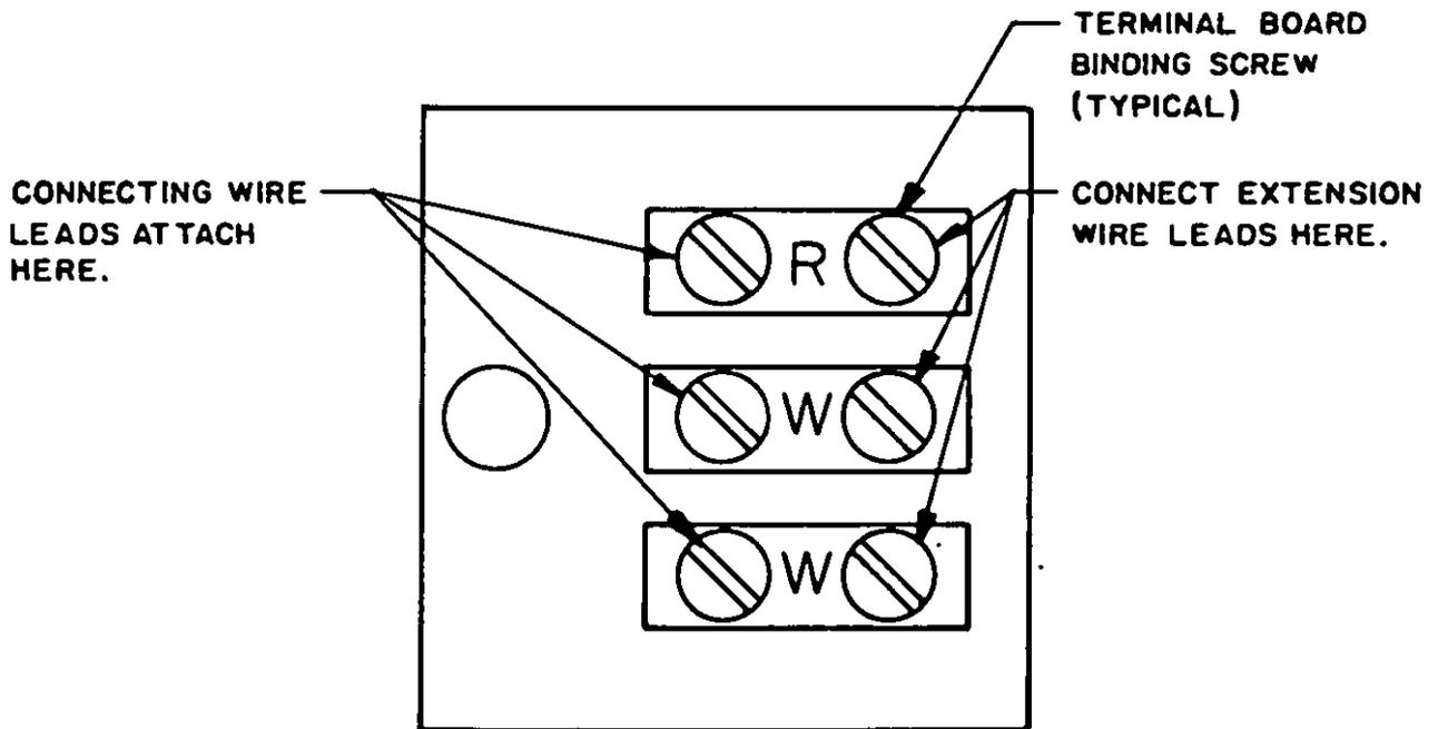
Terminal board for resistance thermometer.
