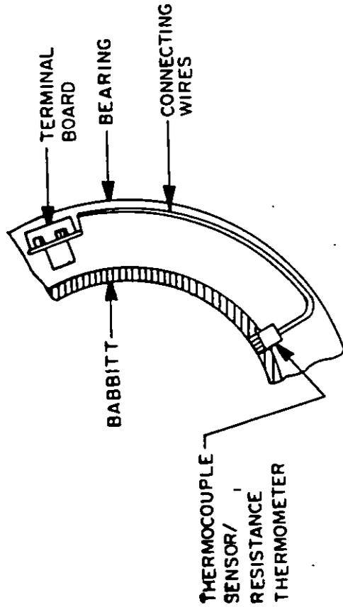
Typical embedded configuration installation.
