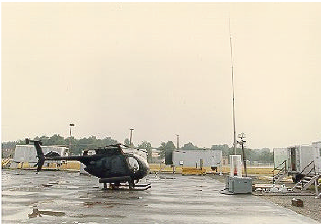
FIGURE 18. Helicopter in Nose-on Orientation From 35-Foot HF Antenna
