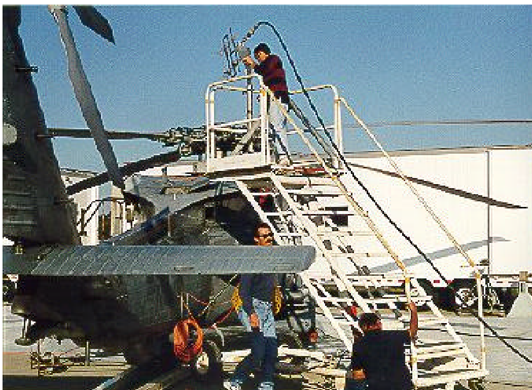
FIGURE 24. Illumination of Test Item at VHF Frequencies
