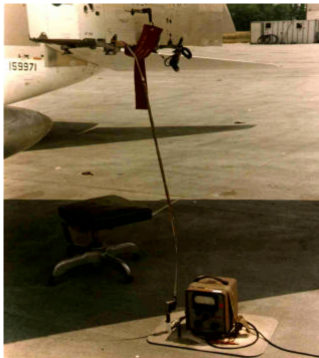
FIGURE 20. Voltage-Ground Measurements Setup
