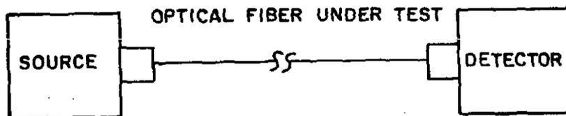
FIGURE 3. Fiber breakage test configuration.
