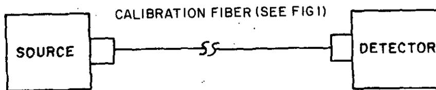
FIGURE 2. Source/optical power meter calibration configuration.
