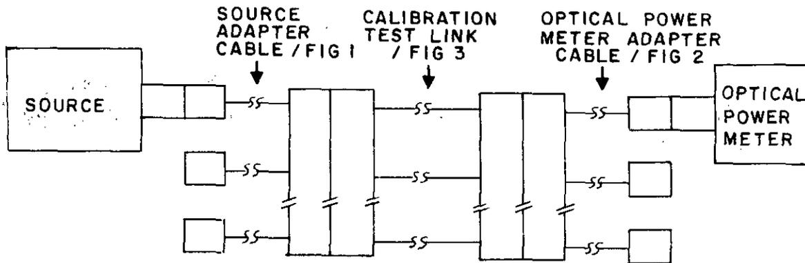
FIGURE 7. Source/optical power meter calibration configuration.
