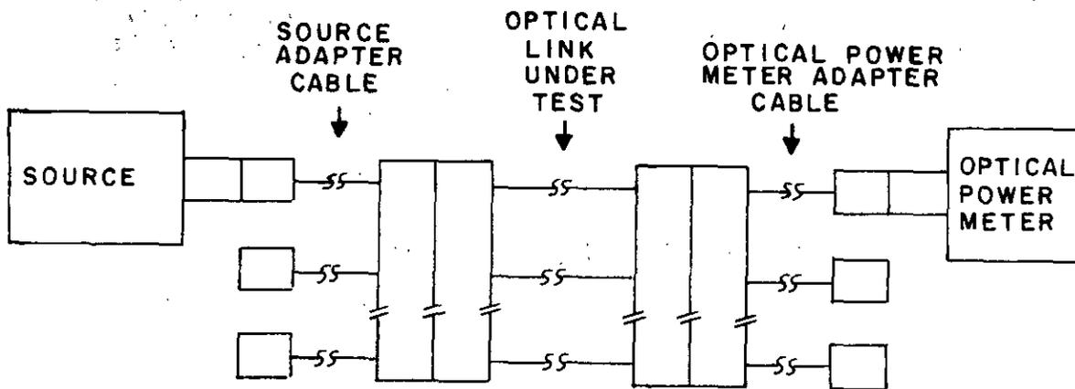
FIGURE 8. Optical link test configuration.
