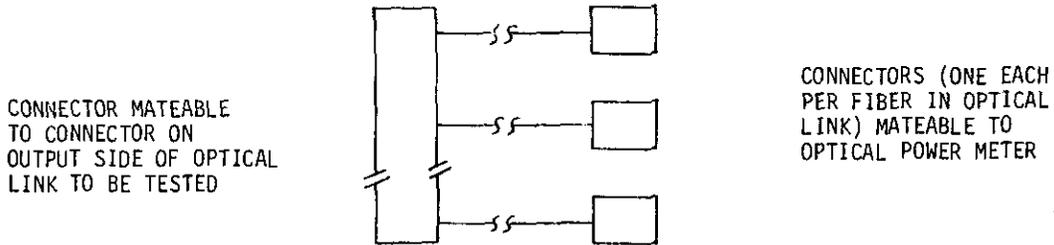
FIGURE 5. Optical power meter adapter cable.
