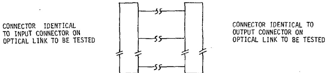
FIGURE 6. Calibration test link.
