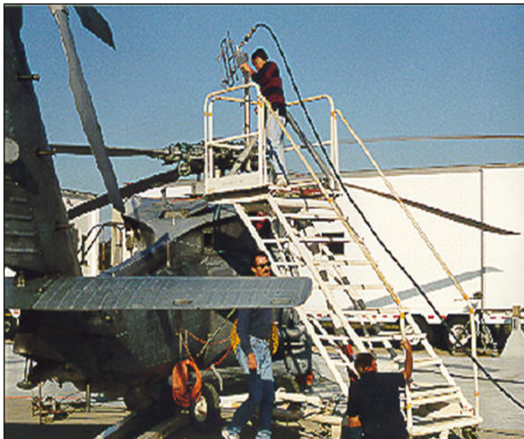
FIGURE 27. Illumination of test item at VHF frequencies
