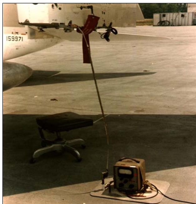
FIGURE 25. Voltage-ground measurement setup
