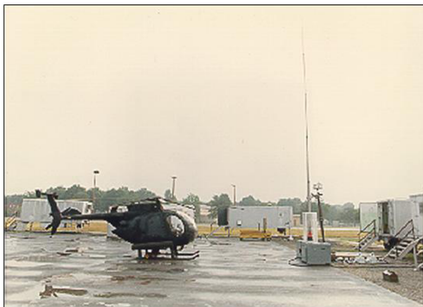
FIGURE 23. Helicopter in nose-on orientation from 35-foot HF antenna
