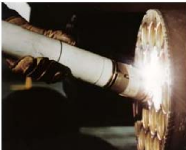
FIGURE 29. RF arc generated during HERO testing
