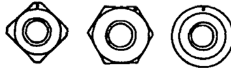
AMERICAN STANDARD SQUARE, HEX, AND ROUND WELD NUT (SMALL RAISED DOR ON CHAMFER)
