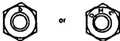
HEX WHEEL NUTS (DEPRESSED "D" or "MDC")
