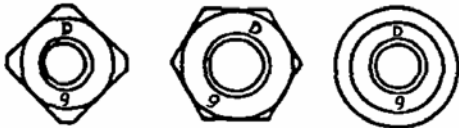
METRIC SQUARE, HEX, AND ROUND WELD NUTS (DEPRESSED LETTER "D" AND CLASS NO.)
