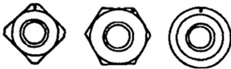
AMERICAN STANDARD SQUARE, HEX, AND ROUND WELD NUT (SMALL RAISED DOT ON CHAMFER)
