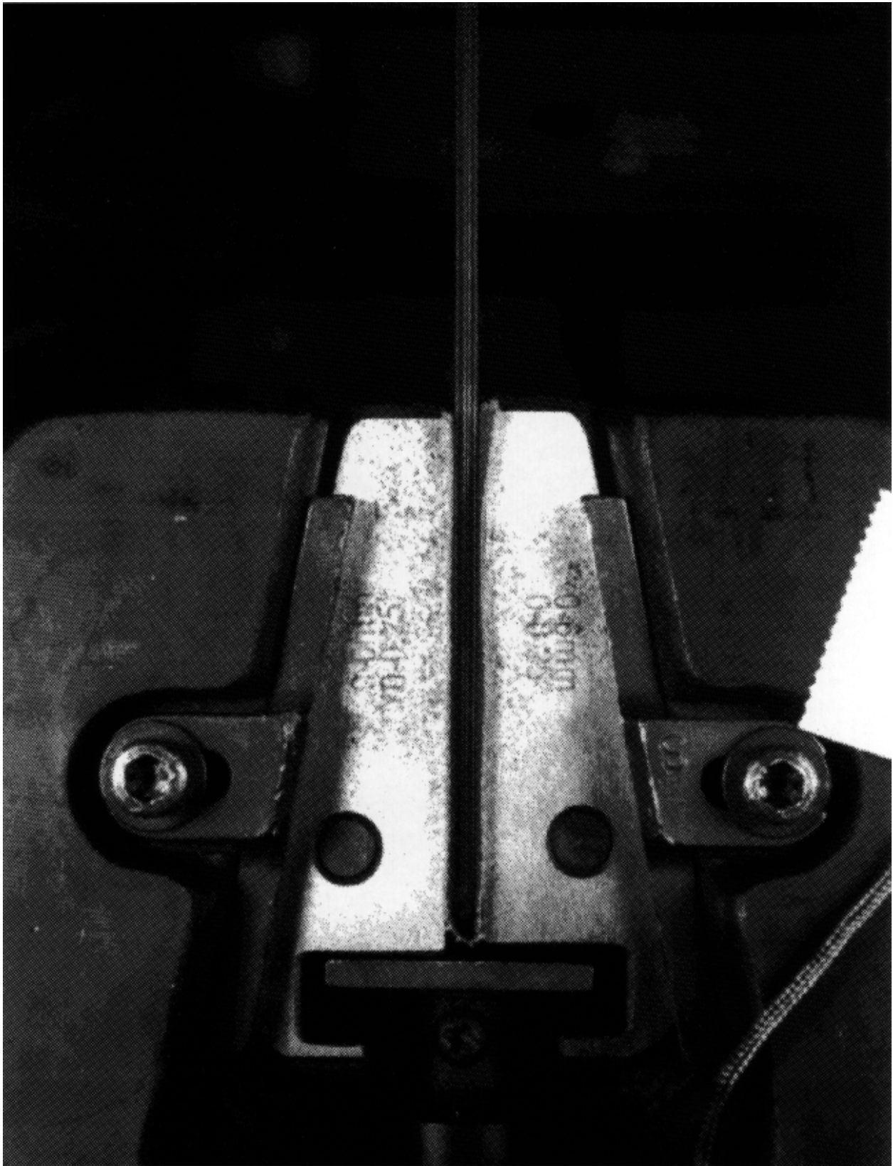
FIGURE 6.7.4.2.1(b) Tension testing of untabbed coupon using an emery-cloth gripping interface.
