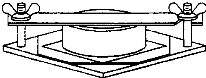
Figure 1.— WATER REPELLENCY TEST APPARATUS
