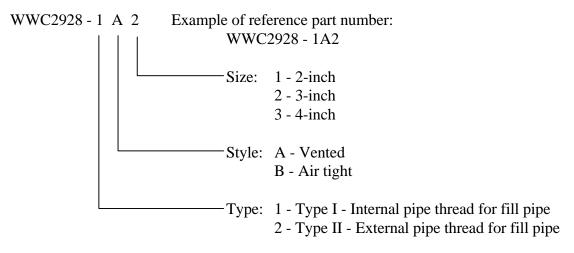
6.6.1 Type, size, and style code. The type and size of the caps are identified by a 3-digit code number and the style is identified by a single alpha character (see table I).
