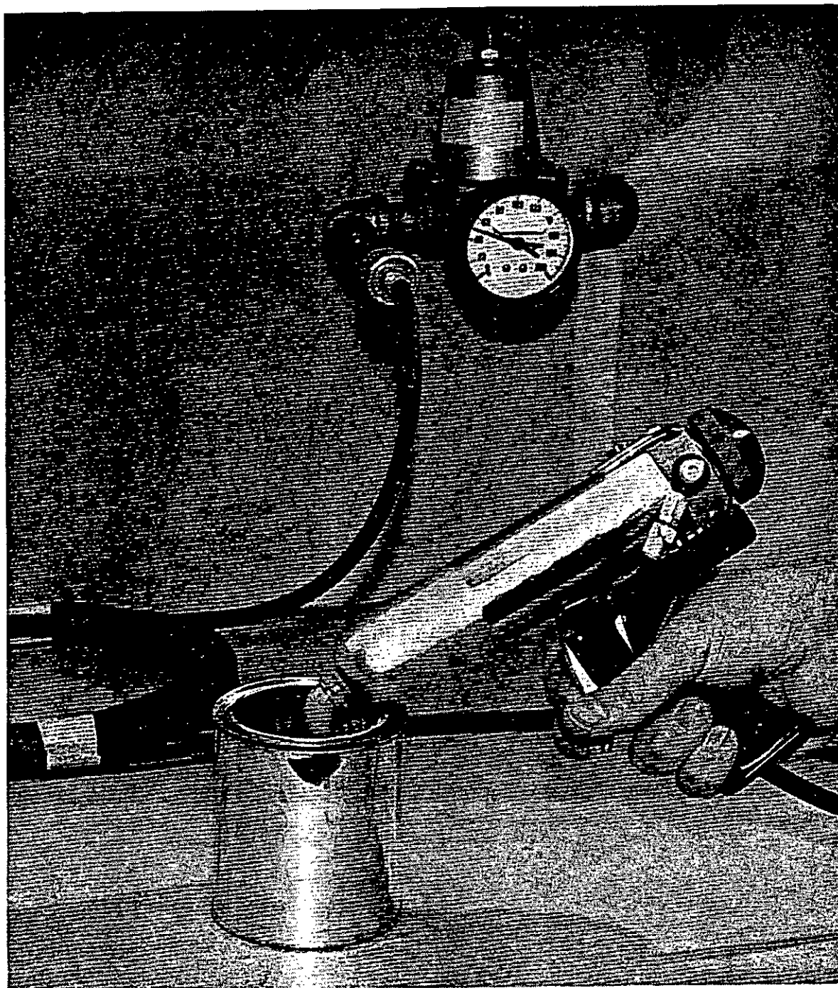
FIGURE 2.—Application life test using a 6 oz power gun containing a 6 oz cartridge without added nozzle, and operated at 50 psi.
