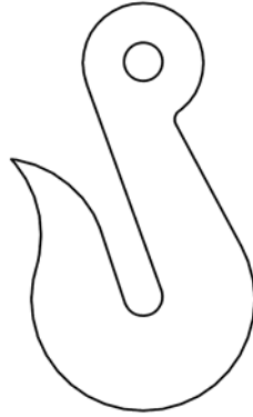
FIGURE 22. Type V, class 2, eye grab hook.
