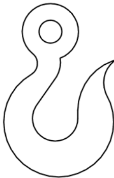
FIGURE 23. Type V, class 3, eye hoist or eye sling hook.
