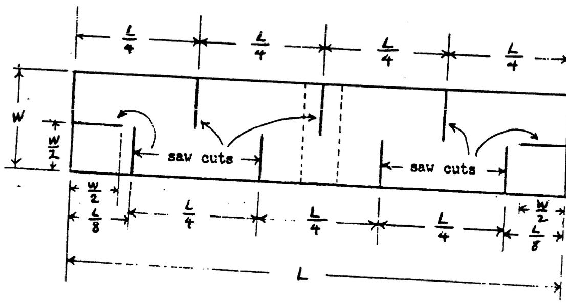
Figure 1. - Locations in ingots from which chemical samples shall be taken.
