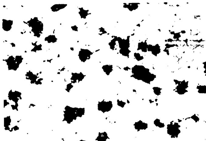
Figure 1. Ferritic malleable iron. Temper carbon in ferrite.
