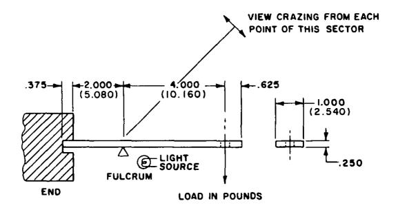
DIMENSIONS IN INCHES, TOLERANCES ON ALL DIMENSIONS SHALL BE ± 0.030 INCH, EXCEPT ON SPECIMEN THICKNESS WHICH SHALL BE IN ACCORDANCE WITH SPECIFICATION MIL-P-5425 (DIMENSIONS IN CENTIMETERS. ± 0.076 CM TOLERANCE)
