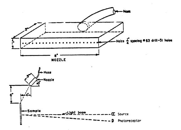
FIGURE 1. Test set up for rainfall test (source and photoreceptor in horizontal plane)
