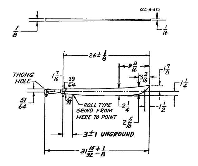
UNLESS OTHERWISE STATED TOLERANCES ARE: WHOLE NUMBERS AND FRACTIONS UP TO TWO INCHES  $\pm \frac{1}{64}$  WHOLE NUMBERS AND FRACTIONS OVER TWO INCHES  $\pm \frac{1}{4}$
