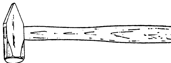
FIGURE 23.—Type X, class 2, blacksmiths', or engineers', cross peen.
