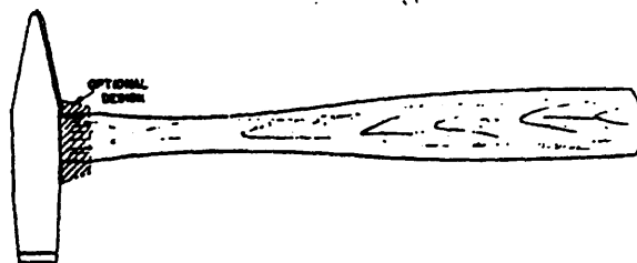
FIGURE 15.—Type VI, scaling (boiler pick).
