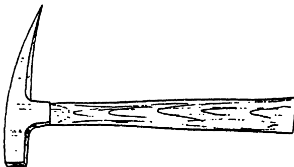
FIGURE 14.—Type V, geologists' (prospecting pick).
