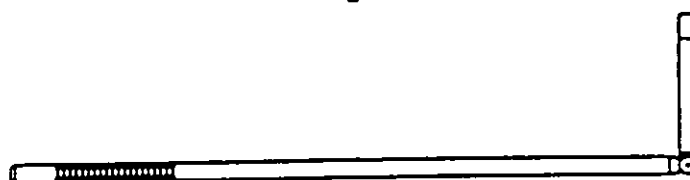
Figure 3. Type II, class 1, retrieving tool, magnetic, telescoping.
