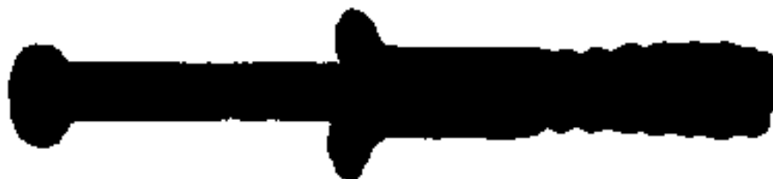
FIGURE 20.—Shield, expansion, nail anchor (steel).
