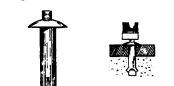
FIGURE 23—Shield, aluminum (aluminum hollow rivet shape nail (pin) anchors). Style 2. Anchor with a cross-slit stem.
