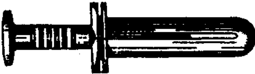
FIGURE 19.—Shield, expansion, nail anchor (aluminum).
