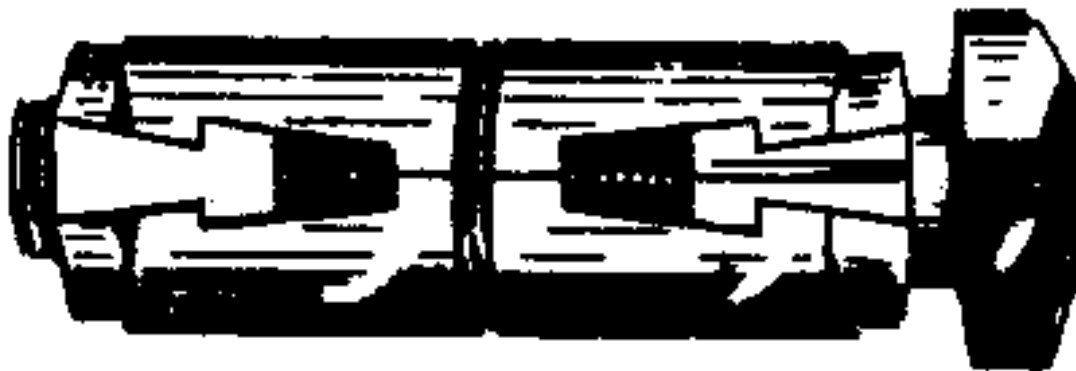
FIGURE 12.—Shield, expansion, anchor (machine bolt). Style 2. Double-end expansion shield anchor.
