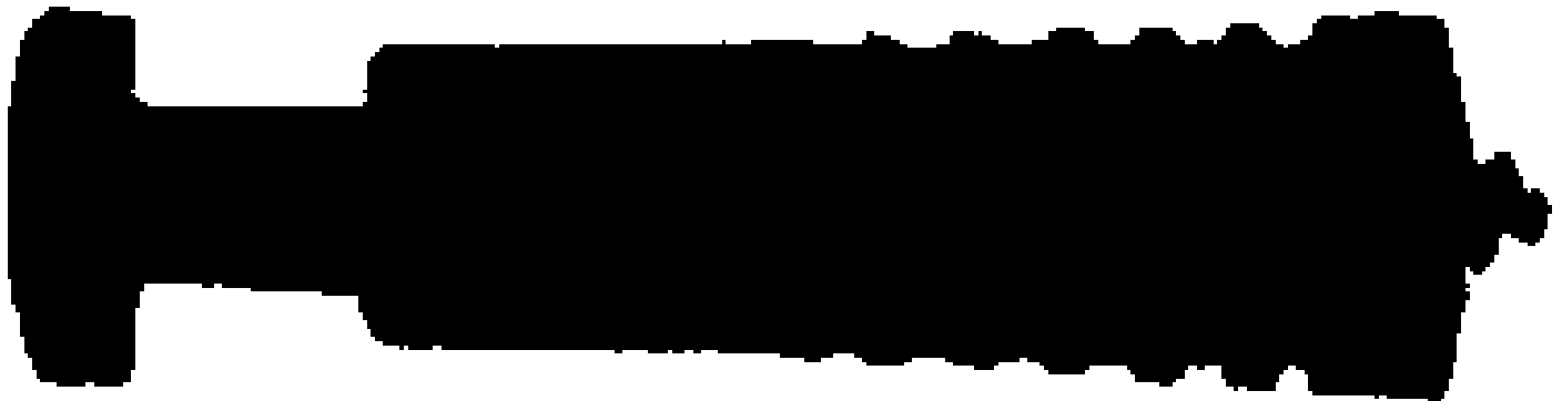
FIGURE 9.—Shield, expansion, anchor (lag bolt).
