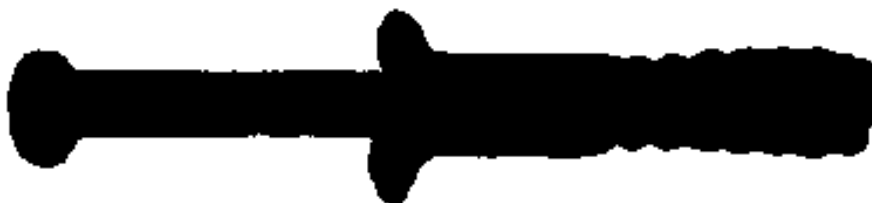
FIGURE 20.—Shield, expansion, nail anchor (steel).
