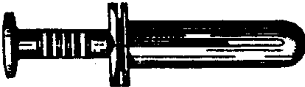
FIGURE 19.—Shield, expansion, nail anchor (aluminum).
