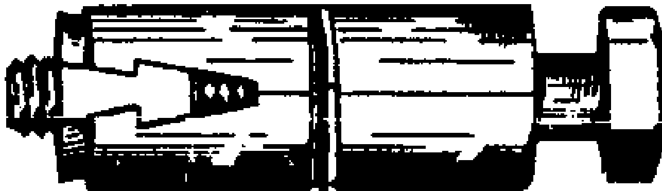
FIGURE 11.—Shield, expansion, anchor (machine bolt). Style 1. Single-end expansion shield anchor.
