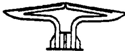
FIGURE 11 TYPE IV PLASTIC SCREW ANCHOR
