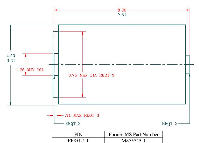
Figure 1. Oil filter element.
