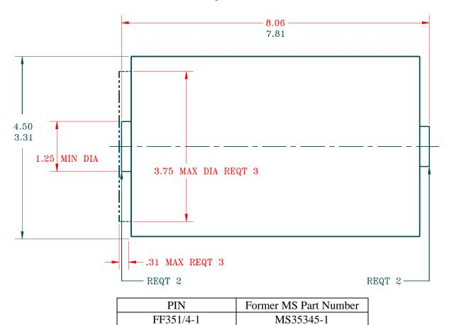
Figure 1. Oil filter element.
