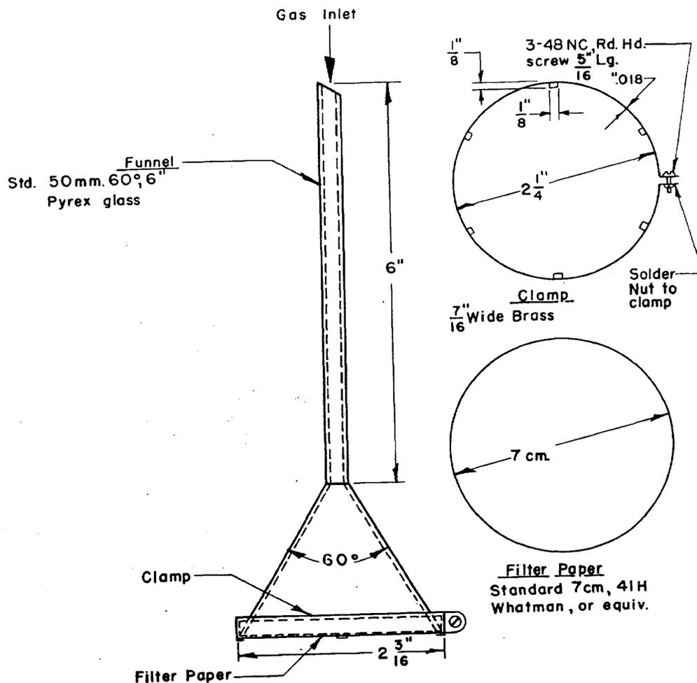
FIGURE 1 - Filter assembly.
