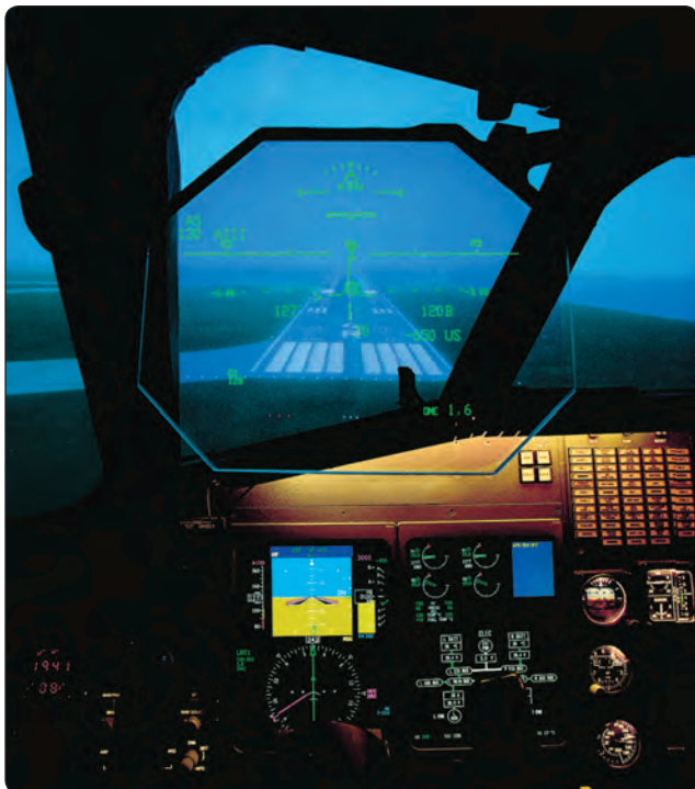
Figure 5-12. Head-up guidance system (HGS).
