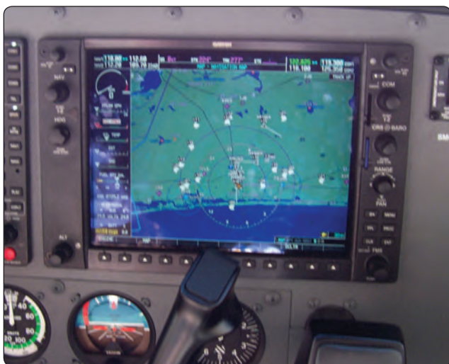
Figure 5-3. Automatic Dependent Surveillance-Broadcast (ADS-B) systems.
