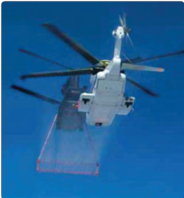
Figure 7-1. Icing tests. To safely provide an all-weather capability and flight into known icing conditions that would otherwise delay or cancel winter flight operations, the digital control of the S-92 Rotor Ice Protection System (RIPS) determines the temperature and moisture content of the air and removes any ice buildup by heating the main and tail rotor blades. The system is shown here during testing.
