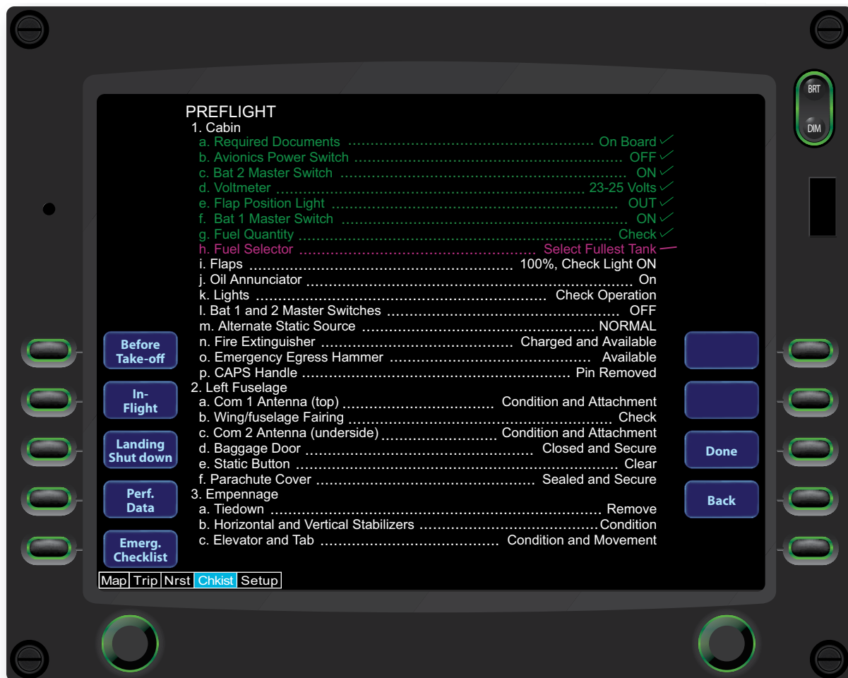
Figure 5-23. A pretakeoff checklist shown on an MFD.
