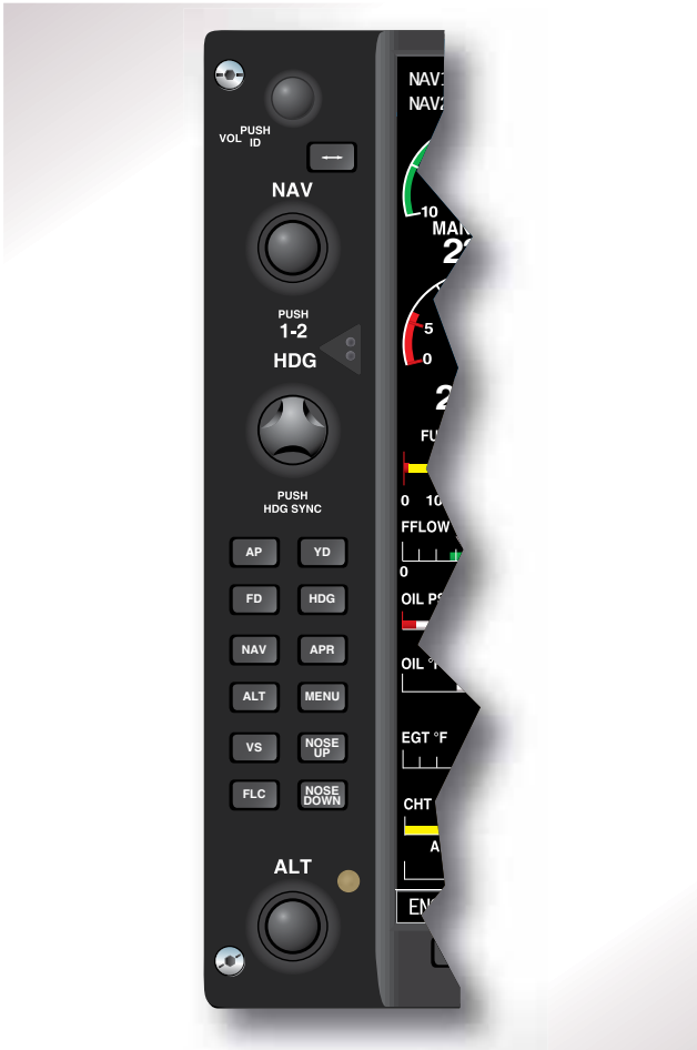
Figure 4-3. An integrated avionics system with an autopilot.
