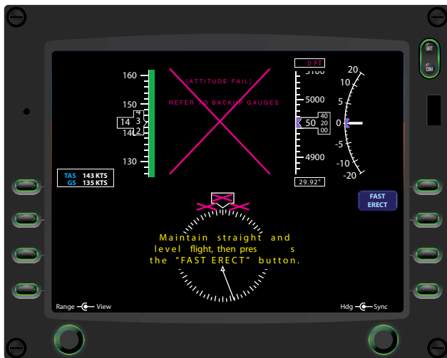
Figure 2-8. A PFD indicating a failed AHRS.
