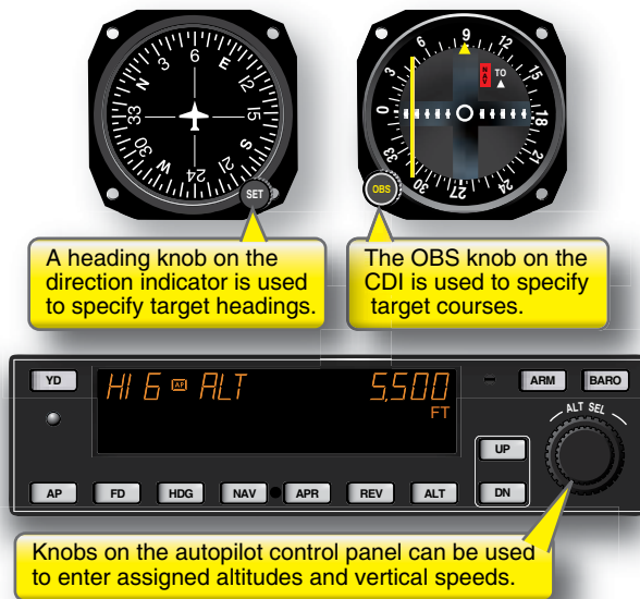
Figure 4-1. A simple autopilot.
