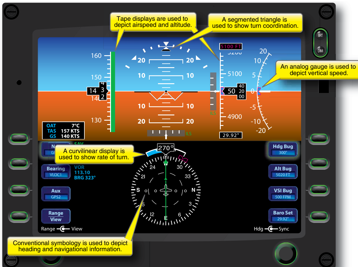
Figure 2-1. A typical primary flight display (PFD).
