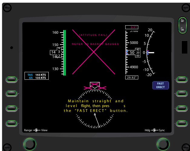
Figure 2-8. A PFD indicating a failed AHRS.
