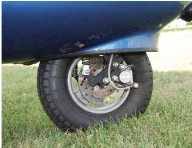
Figure 3-31. Hydraulic disk brake system.
