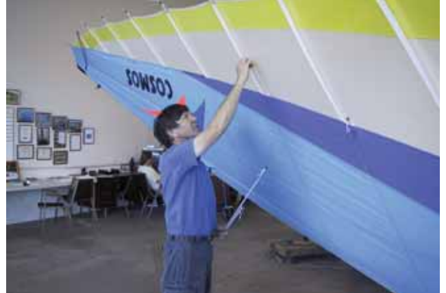
Figure 5-28. Installing the lower surface battens.
