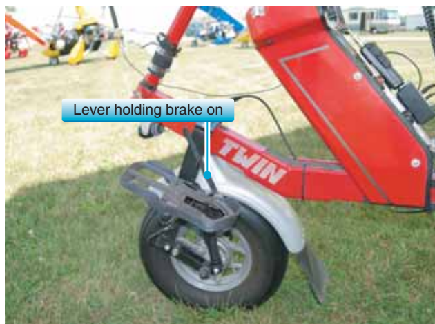
Figure 3-32. Mechanical parking brake system.
