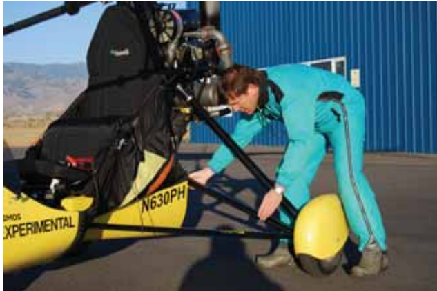
Figure 5-51. Checking the rear landing gear struts.
