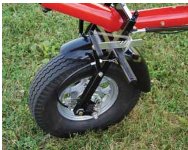
Figure 3-30. Mechanical drum brake system.
