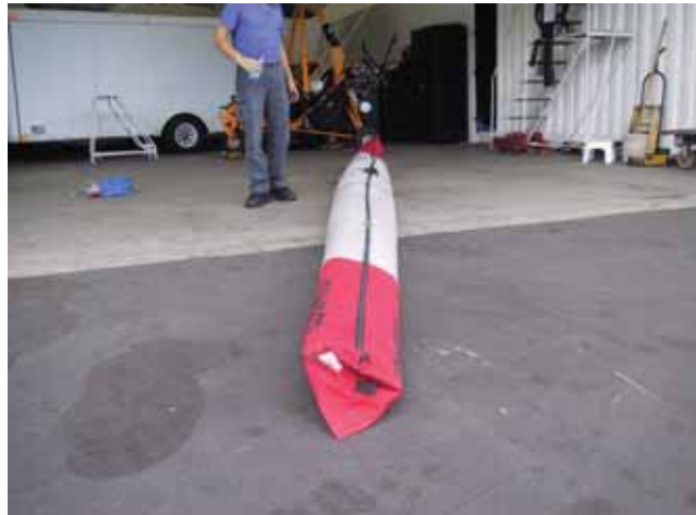
Figure 5-11. Wing positioned for setup.
