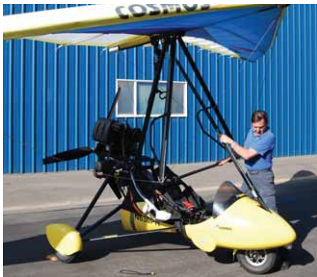
Figure 5-32. Attaching the front tube.
