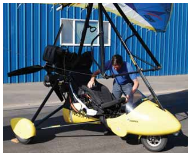
Figure 5-33. Installing the seats.
