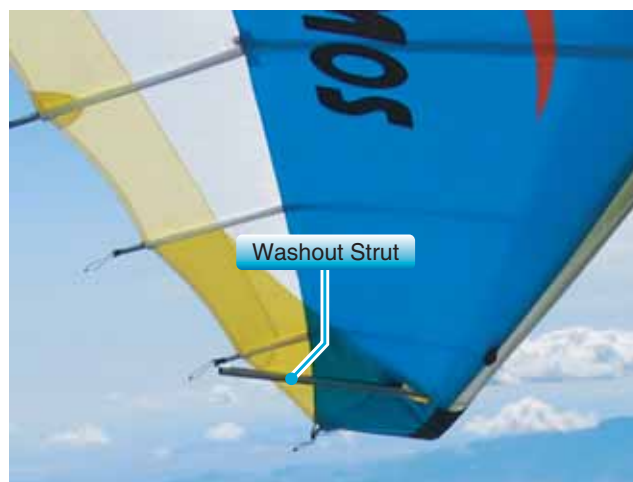
Figure 3-17. Washout struts.
