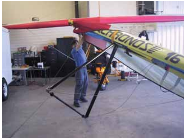
Figure 5-14. Rotating the wing onto its control frame.
