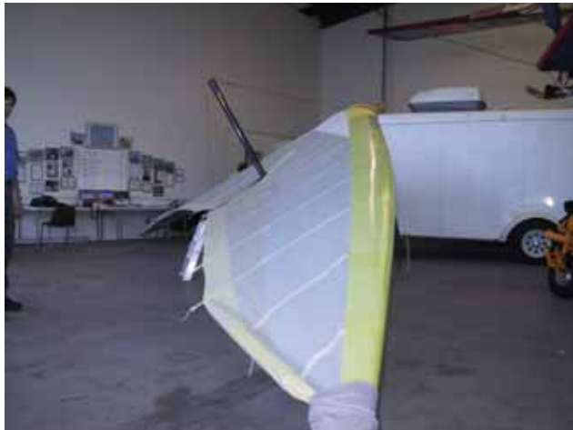
Figure 5-25. The wing tensioned.
