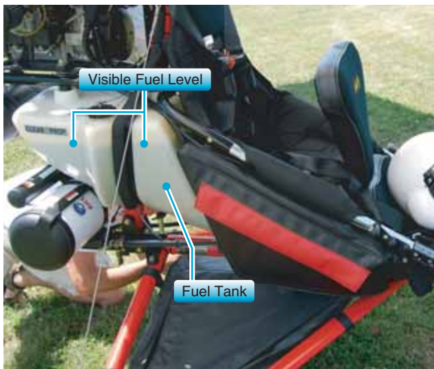
Figure 3-50. Fuel tank with visible fuel quantity.
