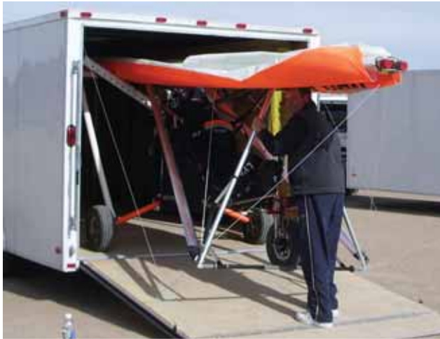
Figure 3-10. Clean upper surface of strutted wing.
