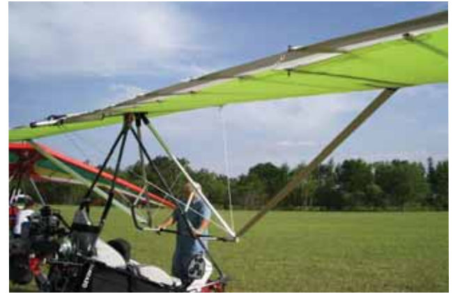
Figure 3-8. Strutted wing on WSC aircraft carriage.
