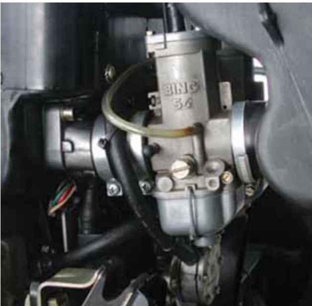
Figure 4-13. Typical two-stroke carburetor.
