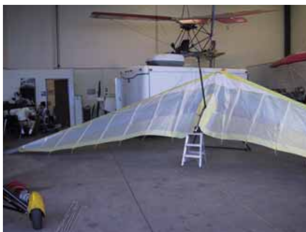
Figure 5-23. Wing ready to tension.
