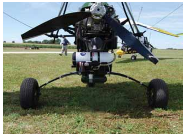
Figure 3-35. Solid flexible main gear.
