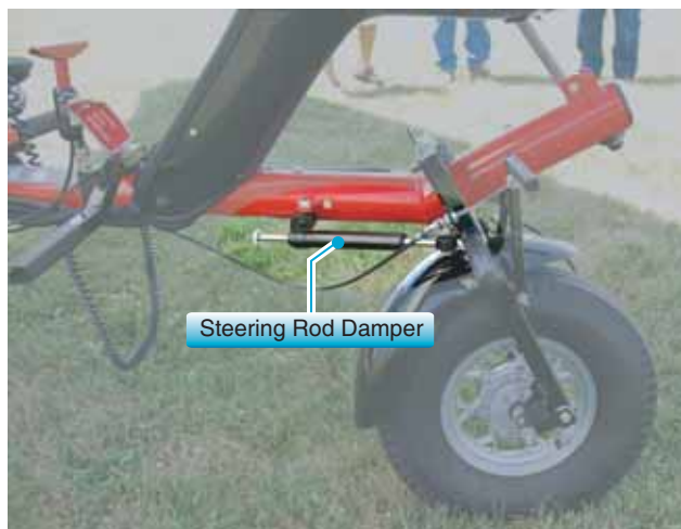
Figure 3-29. Steering rod damper.
