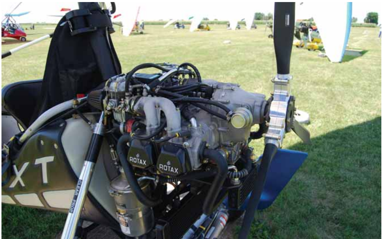
Figure 4-3. Four-stroke water- and oil-cooled engine.
