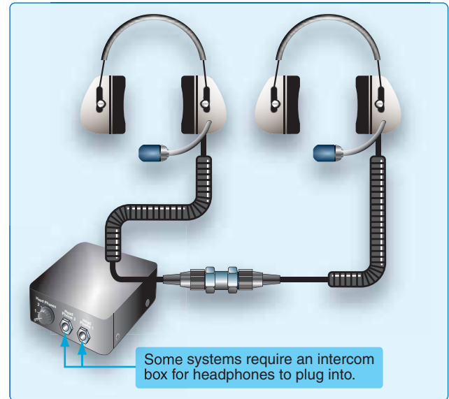
Figure 3-48. Basic pilot-to-passenger communication system.
