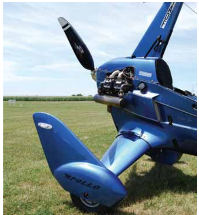
Figure 12-3. Modern LED position lights on carriage wheel pants simplify the installation with no wires running from the carriage to the wing tips.
