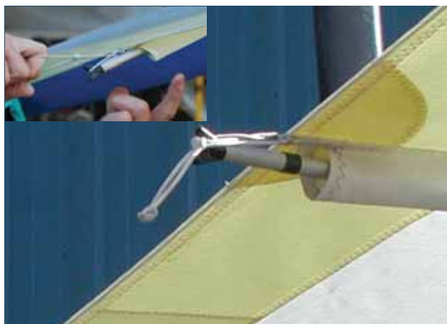
Figure 5-22. Attaching double pull batten (inset). Batten secured into batten pocket.
