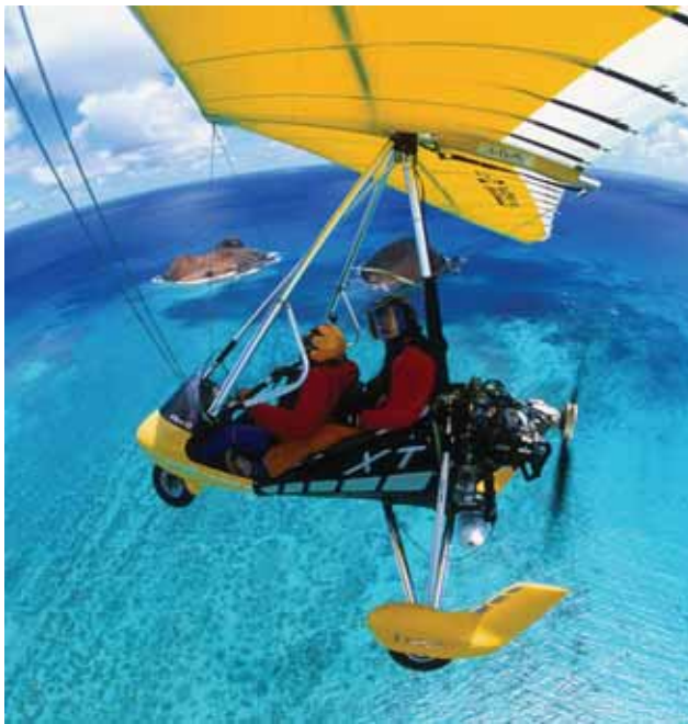
Figure 2-34. Wheel fins for carriage yaw stability.
