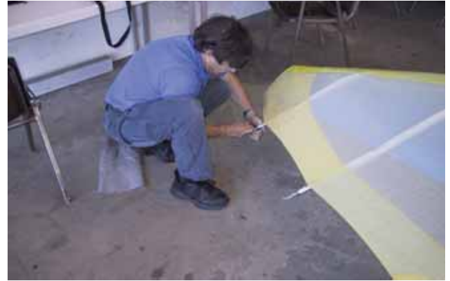
Figure 5-27. Installing the wing tip battens.
