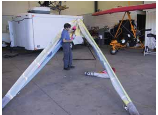
Figure 5-17. Wings spread slightly to raise the kingpost.
