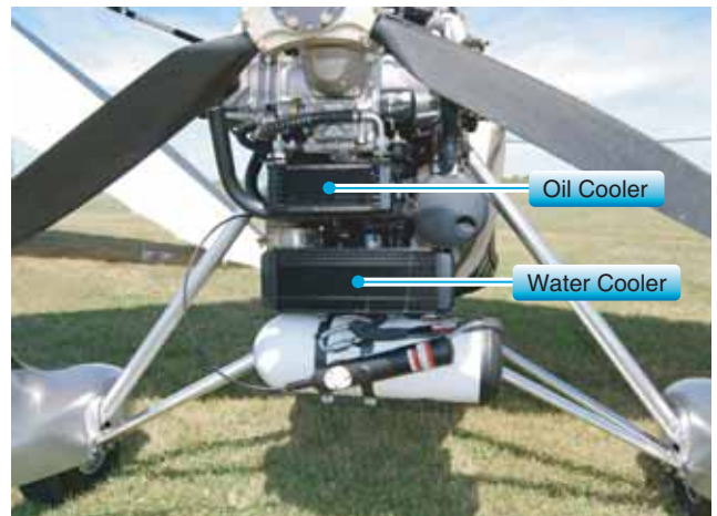
Figure 4-21. Cooling radiators—oil cooler is on top and water cooler is on bottom.
