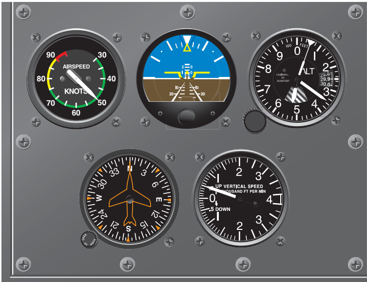
Figure 12-9. Classic instrument gauges for WSC aircraft.
