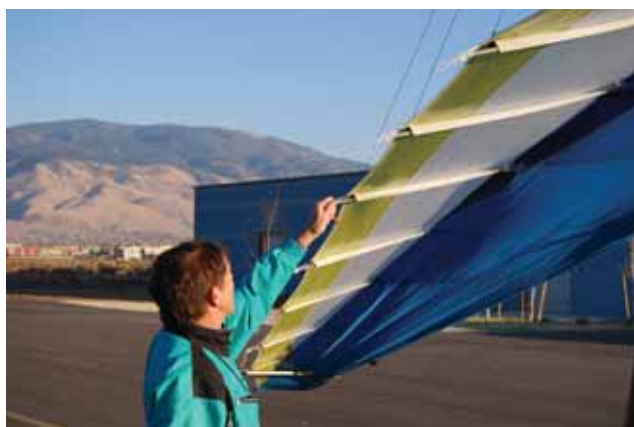
Figure 5-46. Inspecting the trailing edge of the wing.
