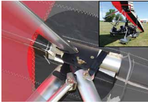
Figure 3-19. Hang point wing attachment.
