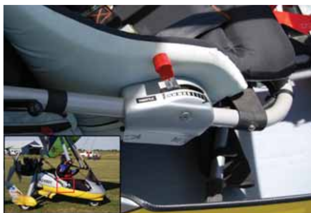
Figure 3-43. Cruise throttle control and ignition switches.
