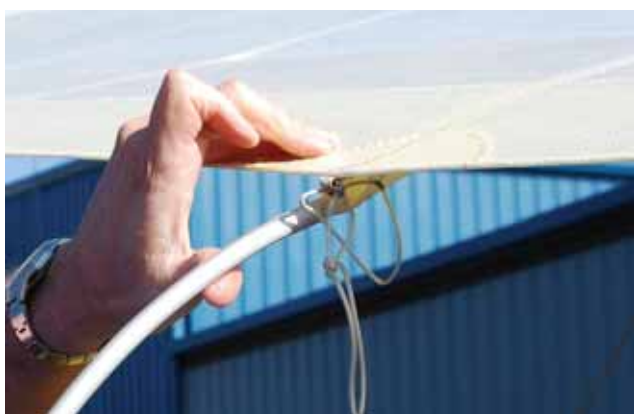
Figure 5-21. Inserting batten into batten pocket.
