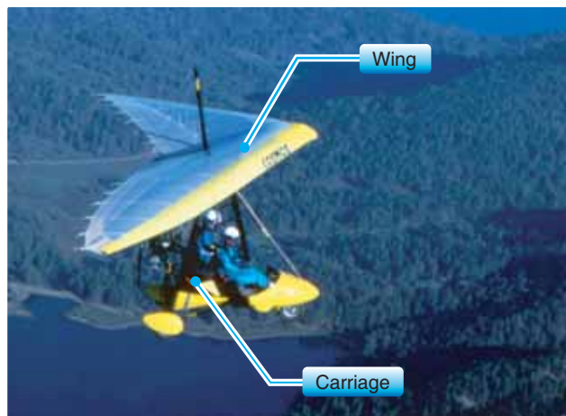
Figure 1-13. Carriage and wing of a WSC aircraft.
