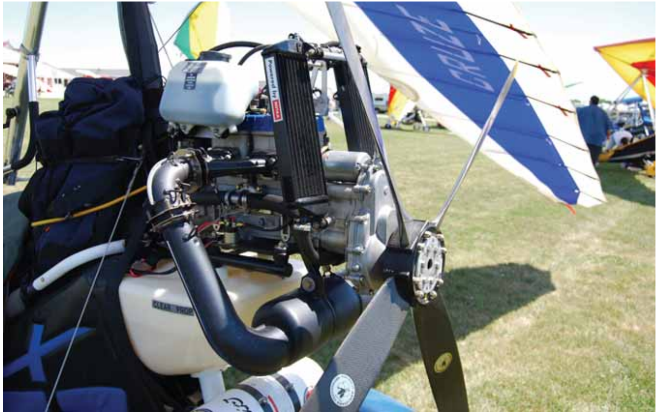
Figure 4-2. Two-stroke water-cooled engine.
