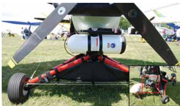
Figure 3-42. Canister mounted under engine.
