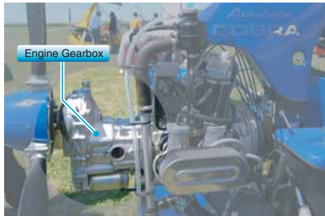
Figure 3-52. Engine gearbox.
