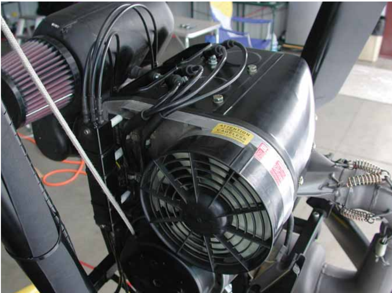
Figure 4-1. Two-stroke air-cooled engine.
