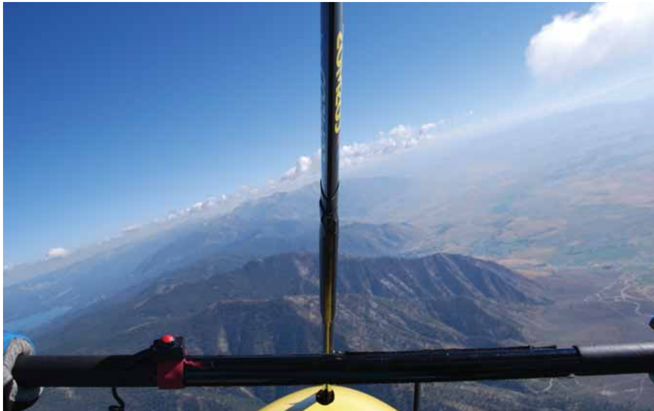
Figure 6-17. Pilot's visual reference of pitch and roll—descending in a shallow bank.
