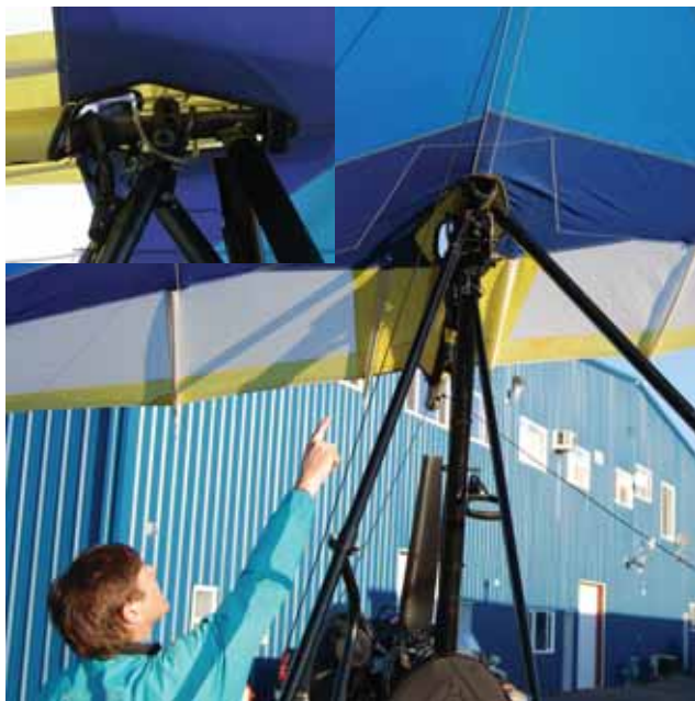
Figure 5-48. Inspecting the wing attachment to the carriage.
