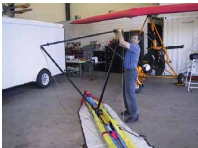
Figure 5-13. Assembling control frame.
