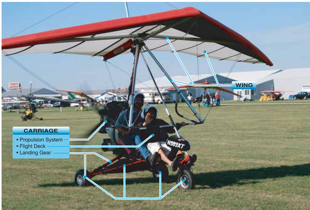
Figure 3-1. Wing and carriage of WSC aircraft.
