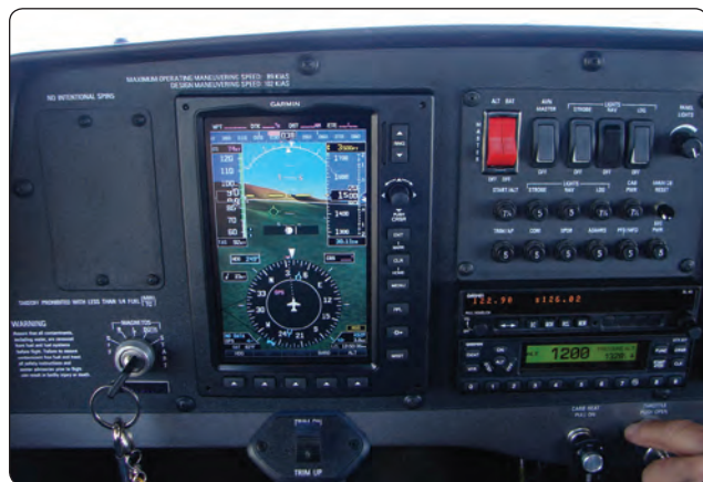
Figure 16-15. EFIS indication of level cruise flight.
