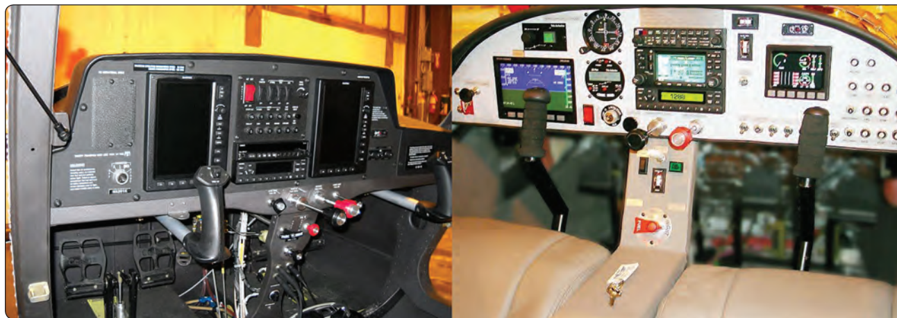
Figure 16-5. An electronic flight instrumentation system provides attitude, airspeed, altimeter, vertical speed, direction, moving map, navigation, terrain awareness, traffic, weather, and engine data all on one or two liquid crystal displays.
