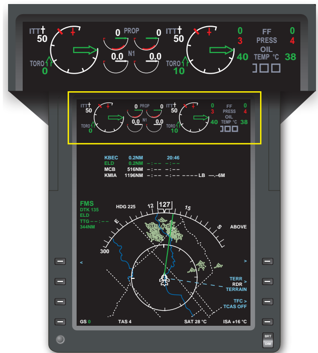
Figure 14-7. Engine instruments—split shaft/free turbine engine.
