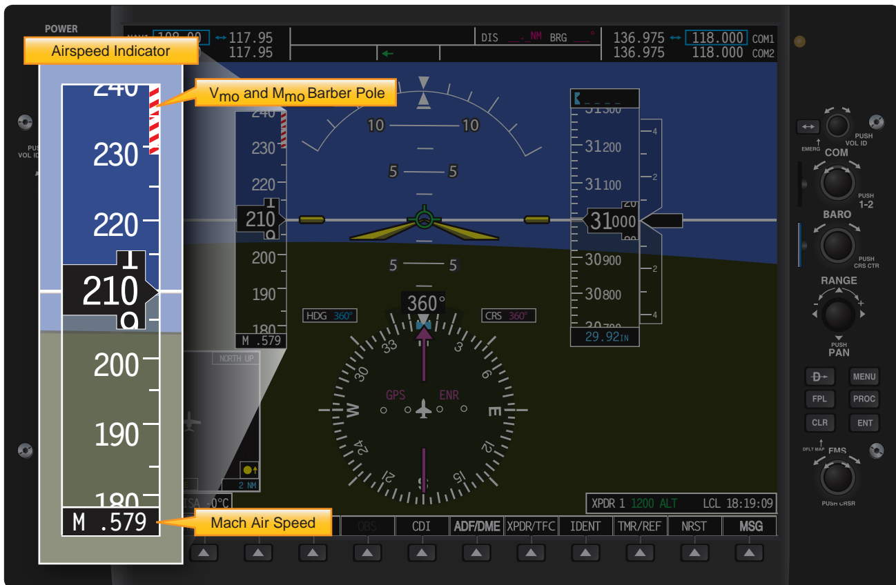
Figure 15-8. Jet airspeed indicator.
