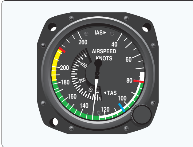
Figure 12-1. Airspeed indicator markings for a multiengine airplane.
