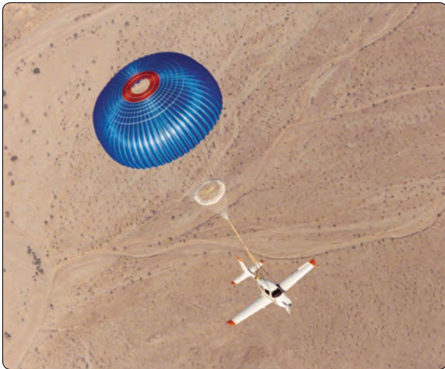
Figure 16-13. A ballistic recovery parachute is a popular safety feature available on some LSA.
