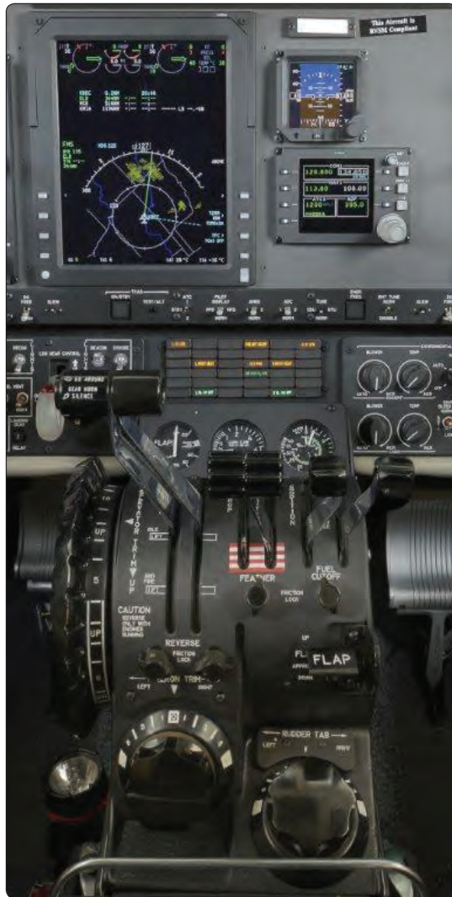
Figure 14-6. Powerplant controls—split shaft/free turbine engine.
