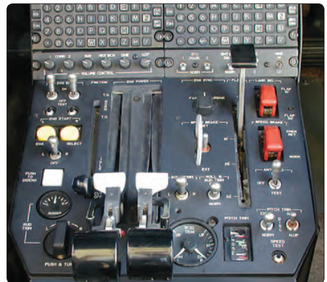
Figure 15-3. Jet engine power controls.
