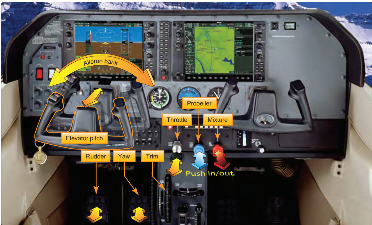
Figure 3-1. Basic flight controls and instrument panel.
