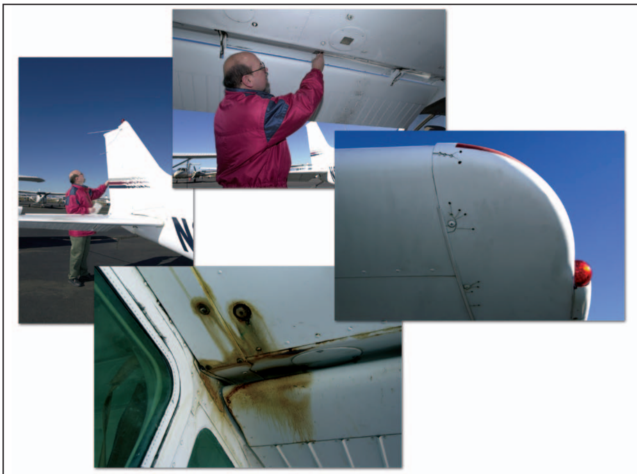
Figure 2-6. Wing and tail section inspection.
