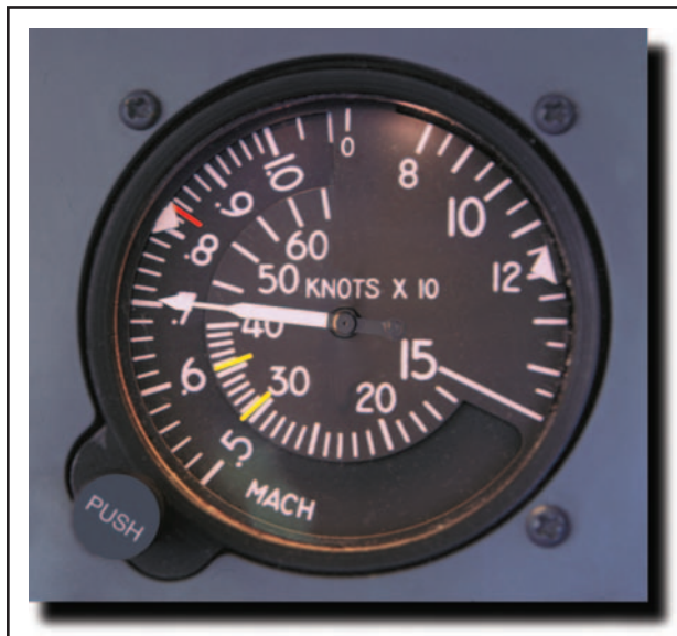
Figure 15-8. Jet airspeed indicator.
