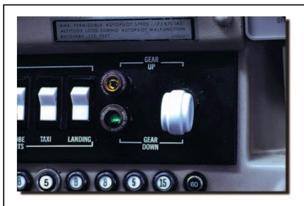
Figure 11-7. Typical landing gear switches and position indicators.
