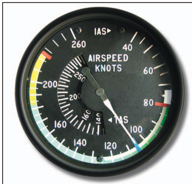
Figure 12-1. Airspeed indicator markings for a multiengine airplane.
