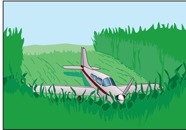
Figure 16-1. Using vegetation to absorb energy.
