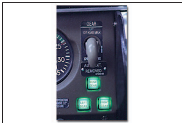
Figure 11-6. Typical landing gear switches and position indicators.
