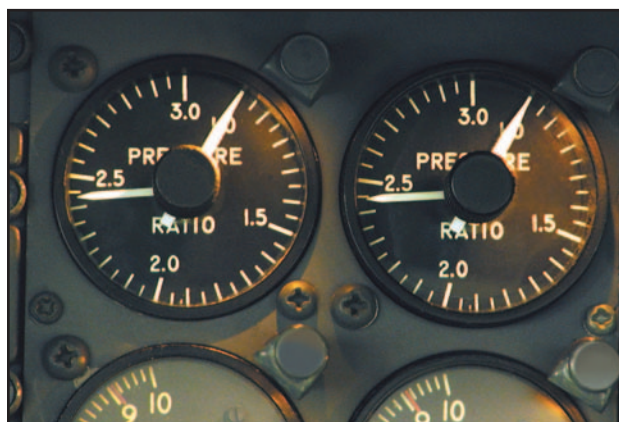
Figure 15-5. EPR gauge.
