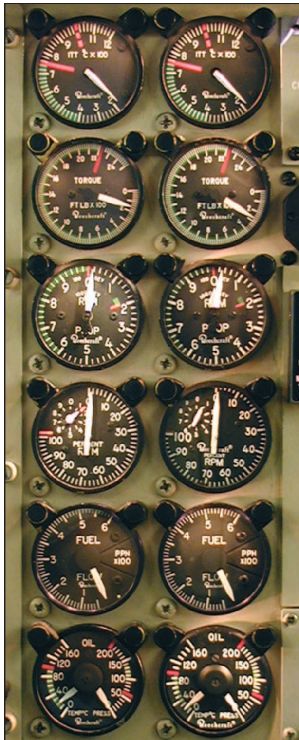
Figure 14-7. Engine instruments—split shaft/free turbine engine.
