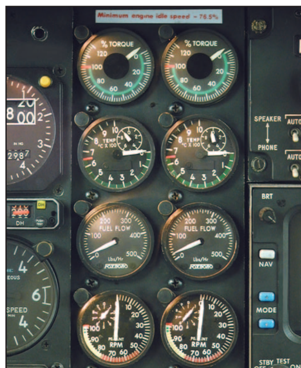
Figure 14-4. Powerplant instrumentation—fixed shaft turboprop engine.
