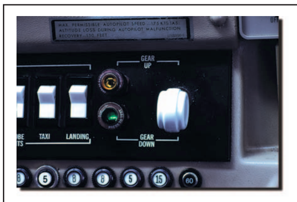
Figure 11-7. Typical landing gear switches and position indicators.
