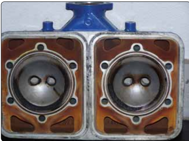
Figure 11-8. Water-cooled heads.
