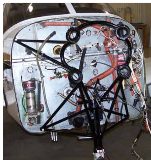
Figure 8-25. Engine mounting ring.
