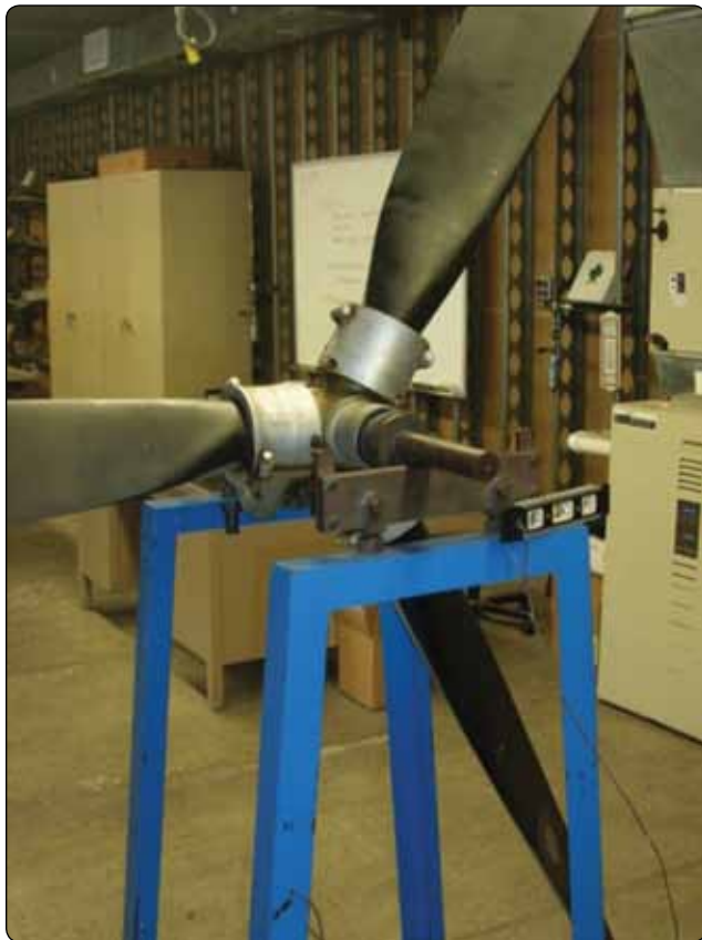
Figure 7-40. Static propeller balancing.
