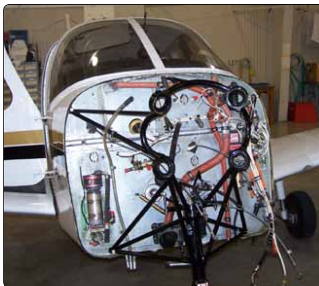
Figure 8-2. Typical firewall with components mounted on it.
