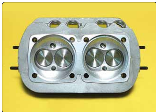
Figure 11-22. Hemispherical combustion chamber within the Revmaster R-2300 Heads.
