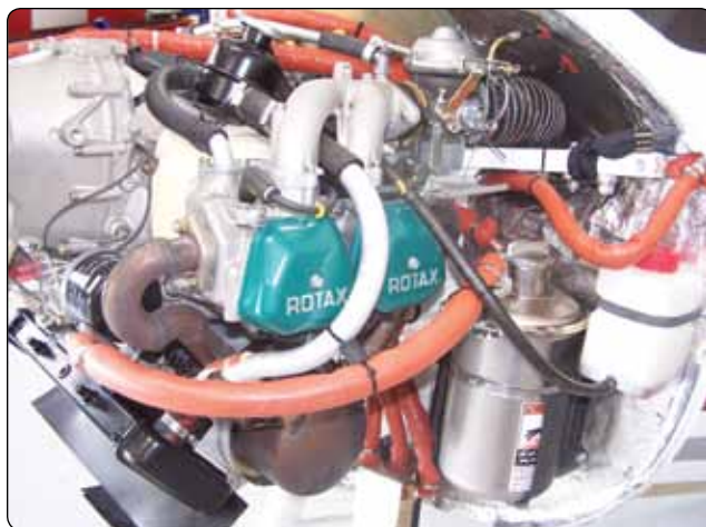
Figure 11-6. Typical four cylinder, four-stroke horizontally opposed engine.
