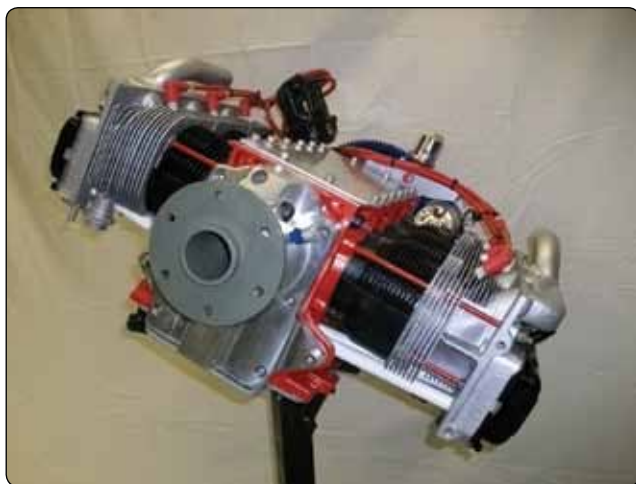
Figure 11-18. Aeromax direct drive, air-cooled, six-cylinder engine.
