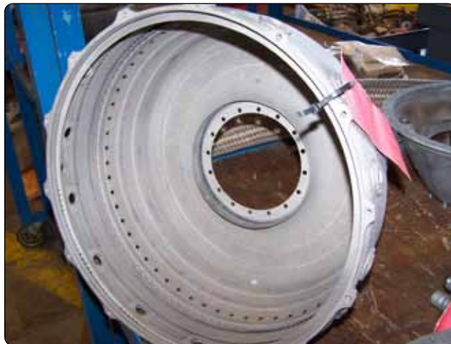
Figure 10-63. Combustion case inspection.
