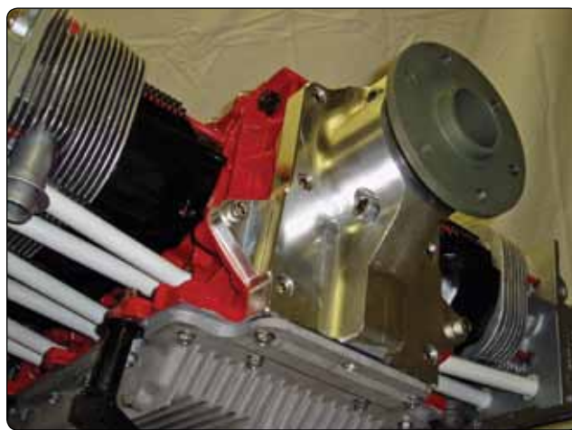
Figure 11-19. Front-end bearing on the 1000 IFB engine.
