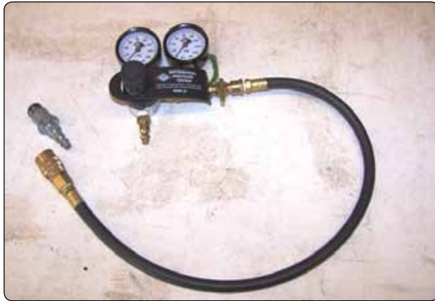
Figure 10-54. Compression tester and adapter.
