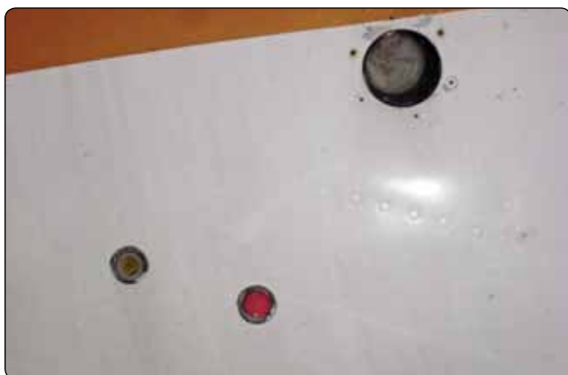
Figure 9-11. Discharge indicators.
