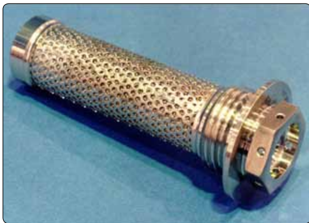
Figure 6-36. Last-chance filter before spray nozzle.
