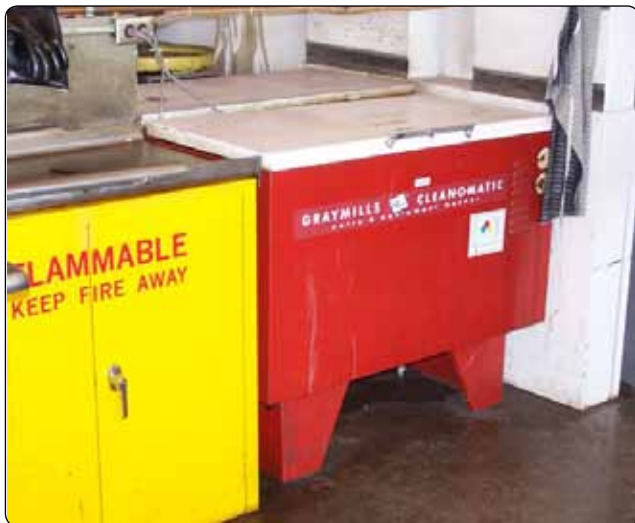
Figure 10-3. Typical solvent degreasing tank.
