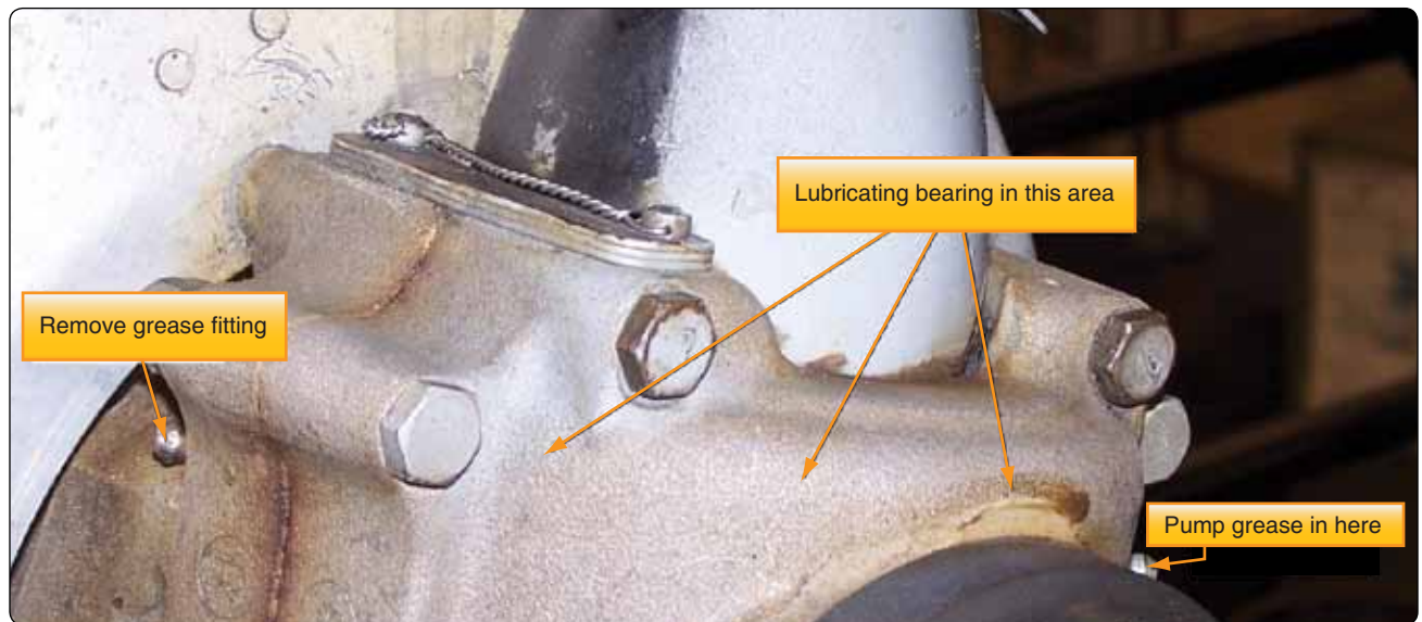
Figure 7-42. Lubricating propeller bearings.
