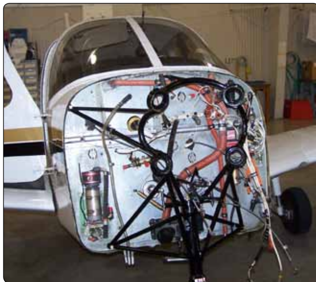
Figure 8-2. Typical firewall with components mounted on it.
