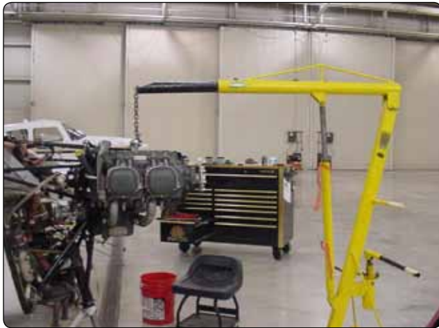
Figure 8-14. Relieve tension on engine mounts.
