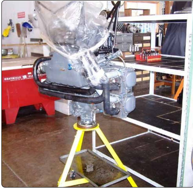
Figure 10-1. Engine mounted on an overhaul stand.
