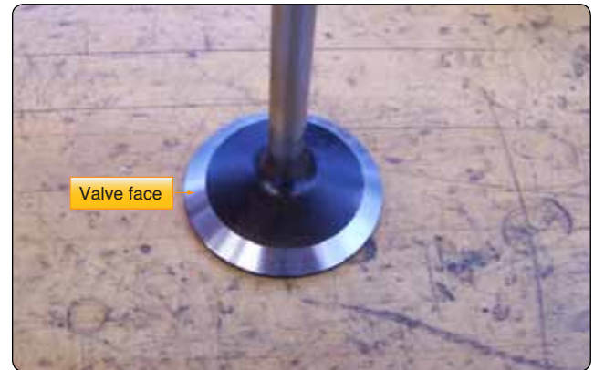
Figure 10-15. Valve face surface.
