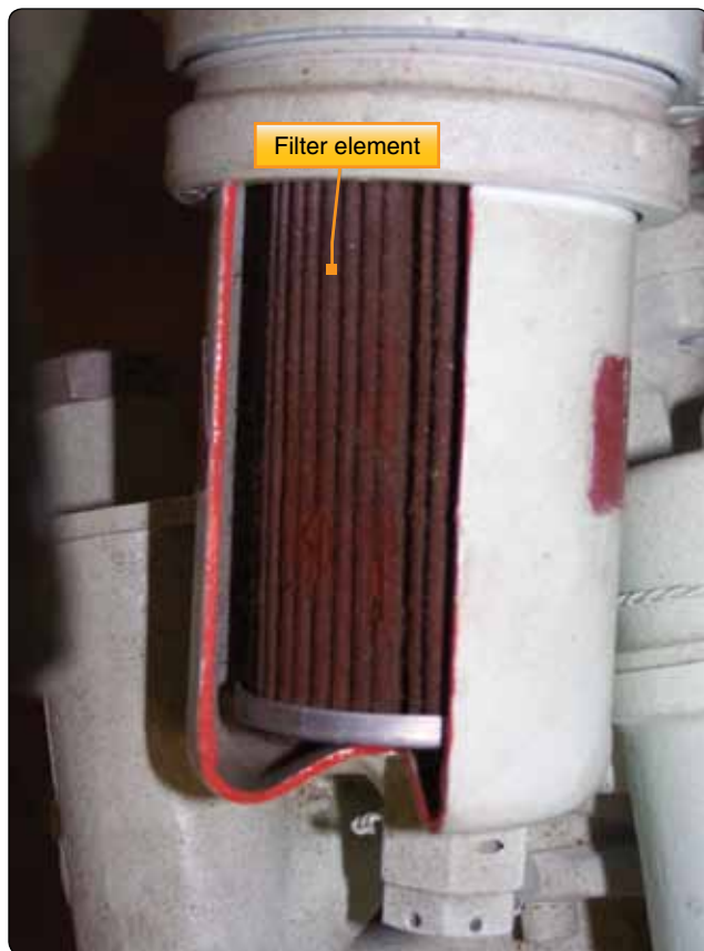
Figure 6-35. Turbine oil filter paper element.
