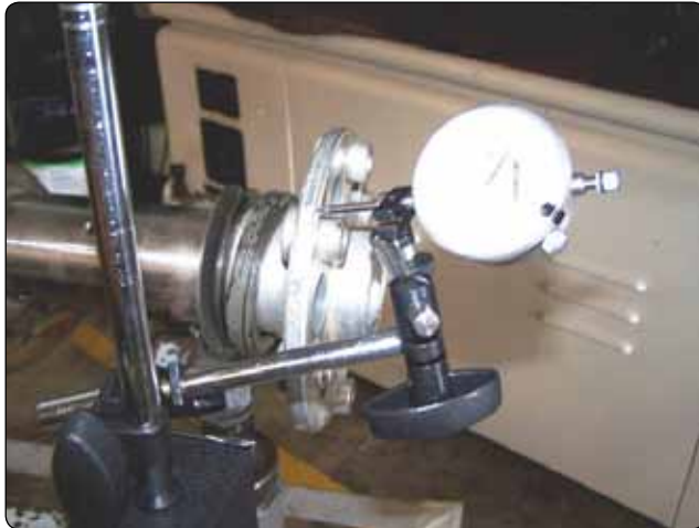
Figure 10-10. Checking crankshaft runout.
