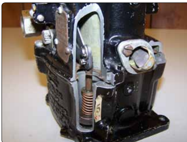
Figure 2-19. Accelerating pump shown in cutaway.
