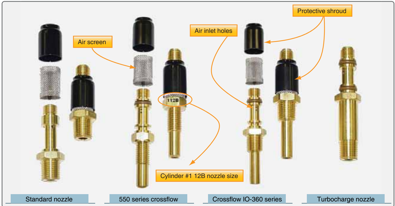
Figure 2-45. Fuel discharge nozzles.
