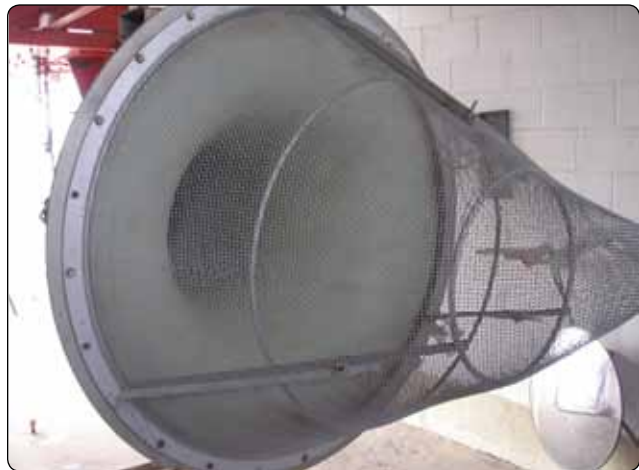
Figure 3-30. A bellmouth inlet used during system tests.
