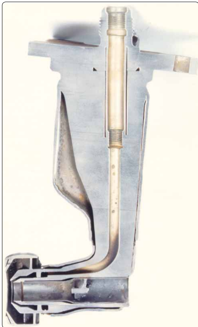
Figure 2-64. Simplex airblast nozzle cutaway.
