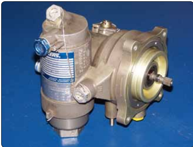
Figure 2-50. Fuel pump and filter.
