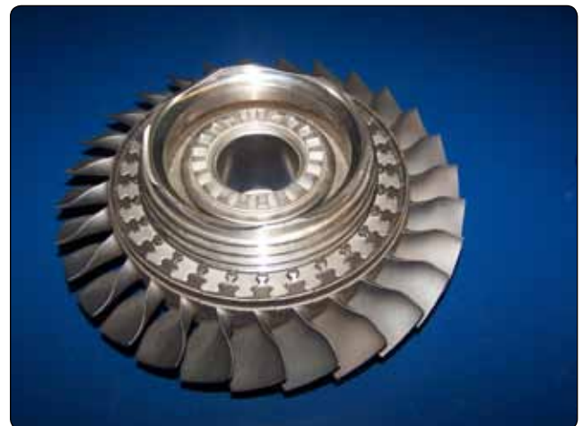
Figure 1-61. Turbine blades.
