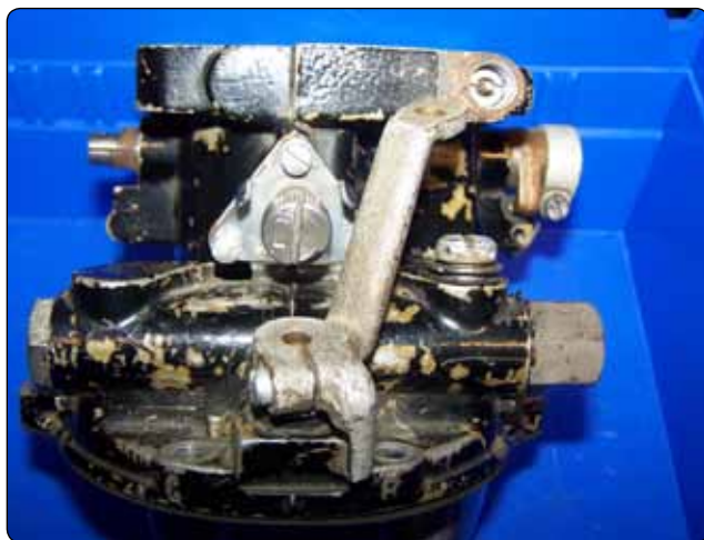
Figure 2-46. Idle mixture adjustment for carburetor.
