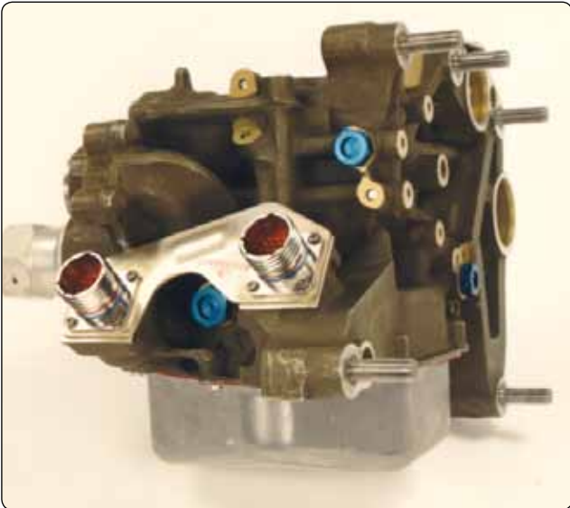
Figure 2-54. Fuel metering unit.
