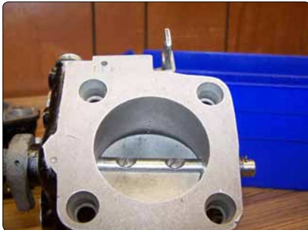
Figure 2-14. Throttle action in idle position.
