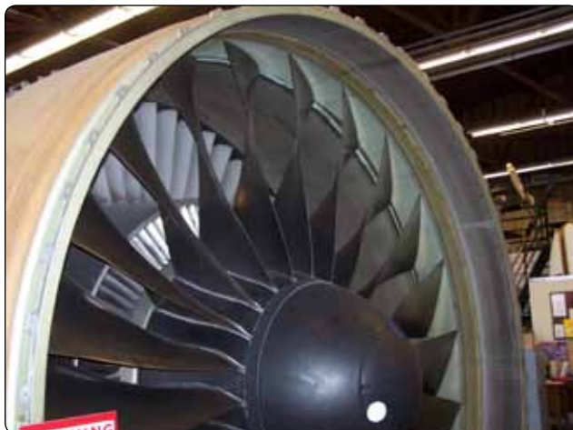
Figure 3-36. The air that passes through the inner part of the fan blades becomes the primary airstream.
