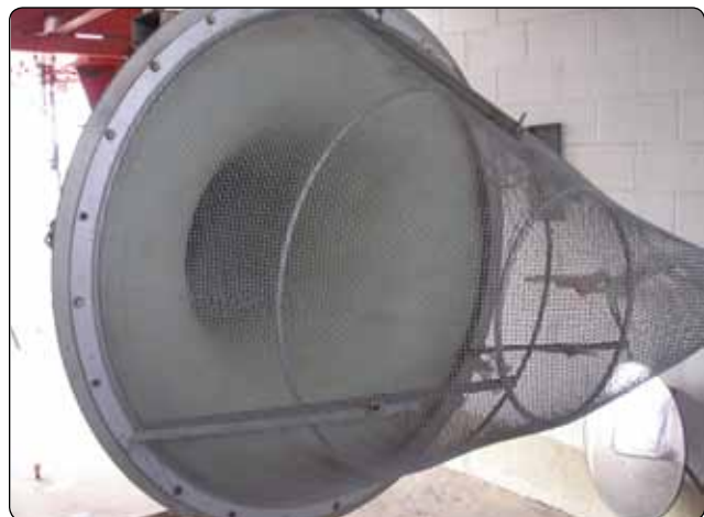
Figure 3-30. A bellmouth inlet used during system tests.
