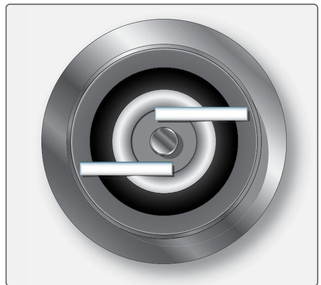
Figure 4-34. Fine wire electrodes.
