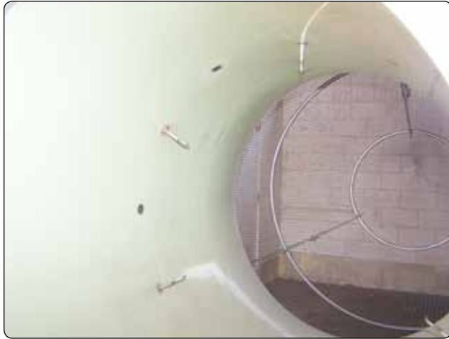
Figure 3-31. Probes within a bellmouth inlet used to measure intake temperature and pressure.
