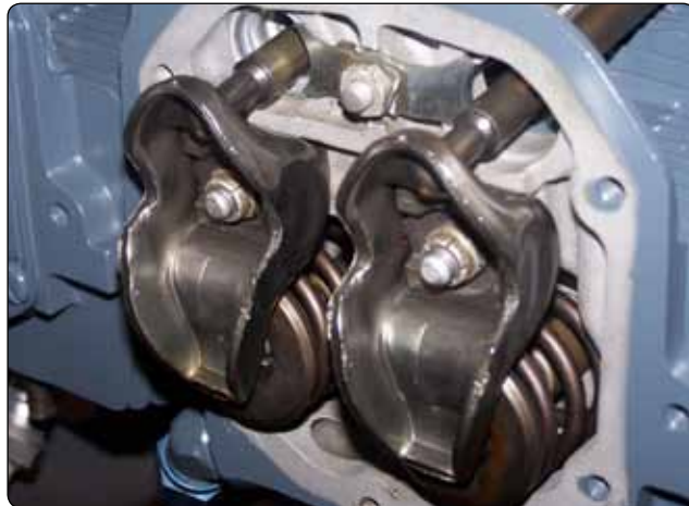
Figure 1-31. Rocker opposed engine arms.
