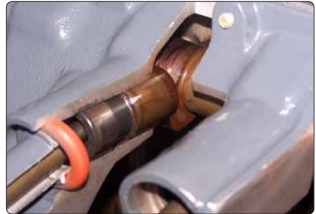
Figure 1-29. Cam load on lifter body.
