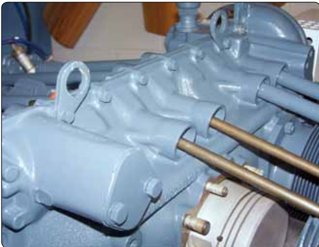
Figure 1-5. The crankcase.
