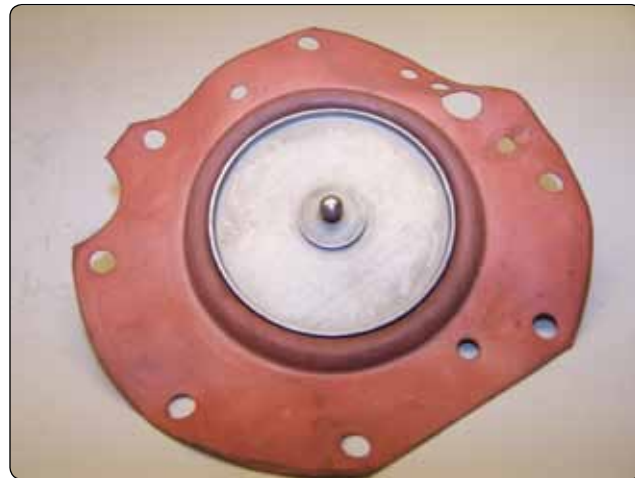
Figure 2-33. Fuel diaphragm with ball valve attached.
