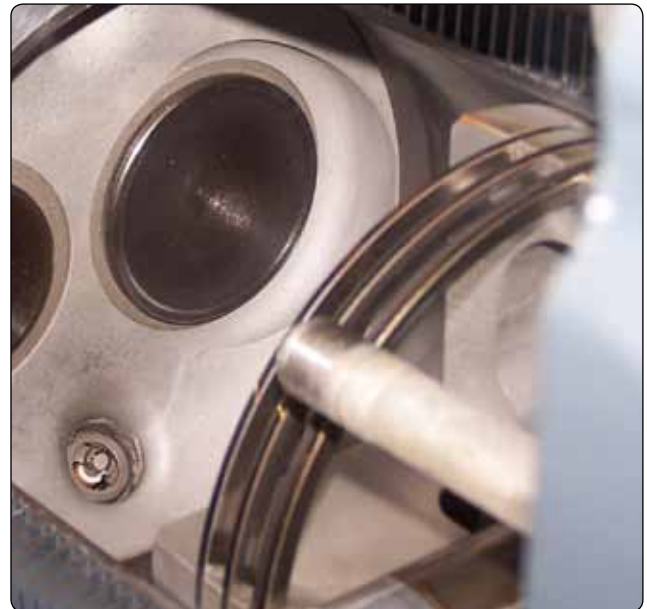
Figure 1-15. Machined rings around a piston.
