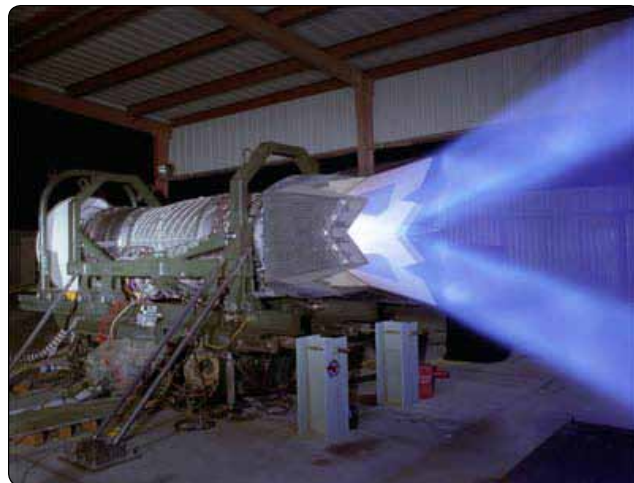
Figure 3-51. A pilot can direct thrust via the vectoring nozzle 20^\circ up or down to increase flight maneuverability.
