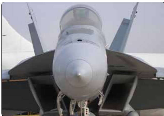
Figure 3-25. An example of a divided-entrance duct.
