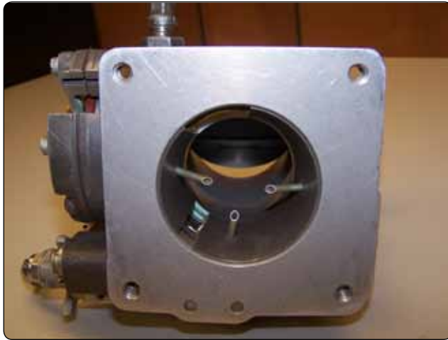
Figure 2-32. Impact tubes for inlet air pressure.
