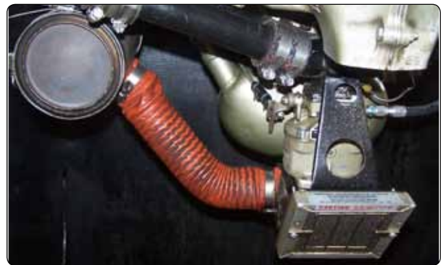
Figure 3-5. Location of a carburetor heat air valve.
