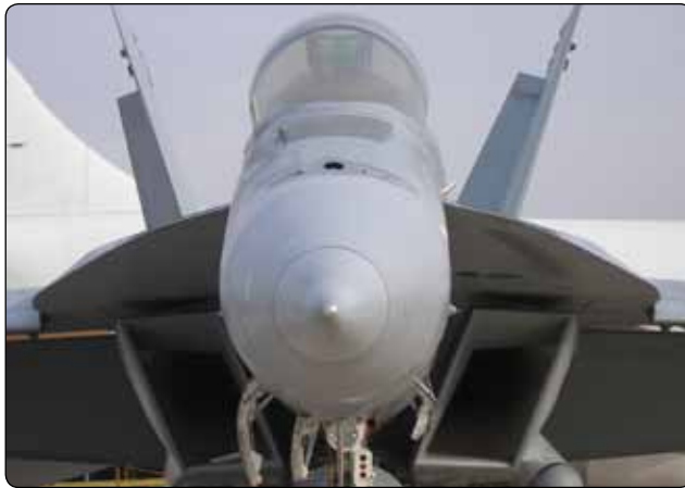
Figure 3-25. An example of a divided-entrance duct.
