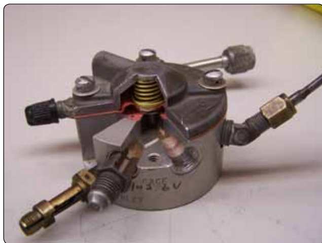
Figure 2-37. Flow divider cutaway.
