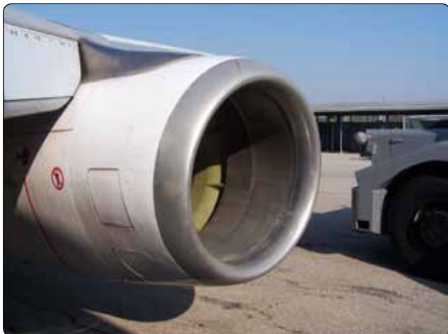
Figure 3-34. A typical turbofan intake section.
