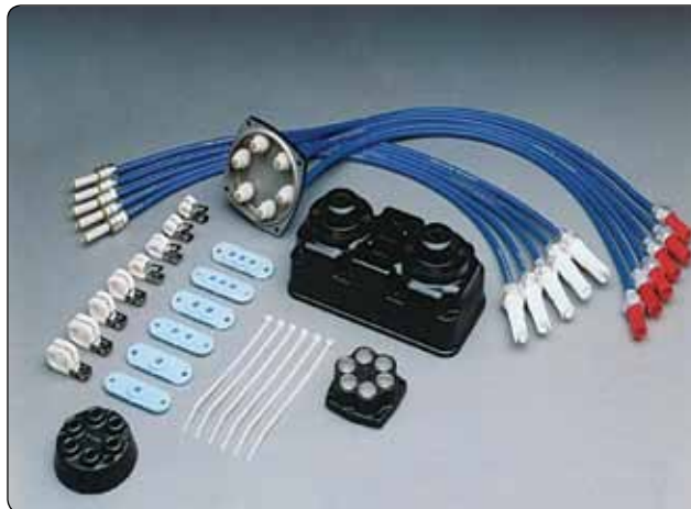
Figure 4-11. A high-tension ignition harness.
