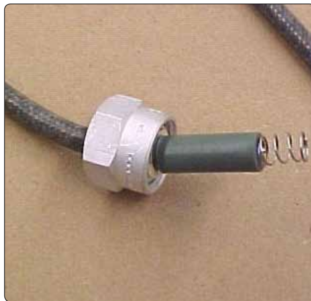
Figure 4-13. Ignition lead spark plug end.
