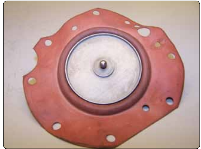
Figure 2-33. Fuel diaphragm with ball valve attached.
