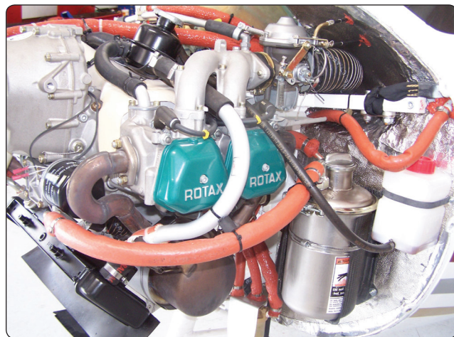
Figure 11-6. Typical four cylinder, four-stroke horizontally opposed engine.
