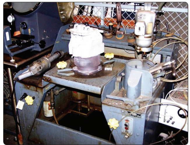
Figure 10-16. Valve seat grinding equipment.
