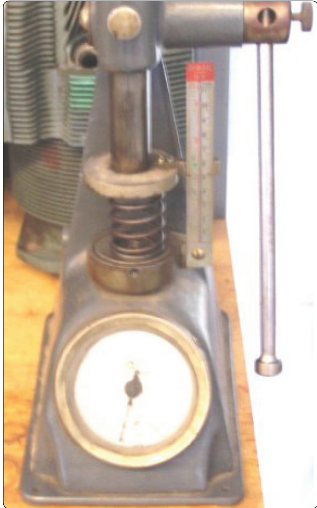
Figure 10-9. Valve spring compression tester.
