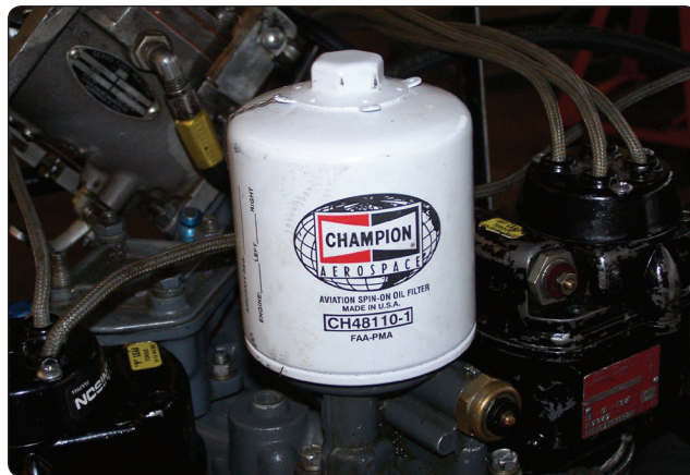
Figure 6-8. Full flow spin-on filter.
