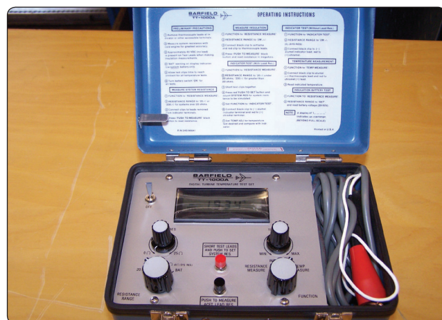
Figure 10-78. EGT analyzer.
