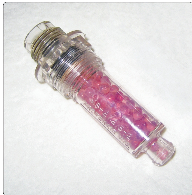
Figure 8-18. Dehydrator plug “pink” showing high humidity (Sacramento Sky Ranch).
