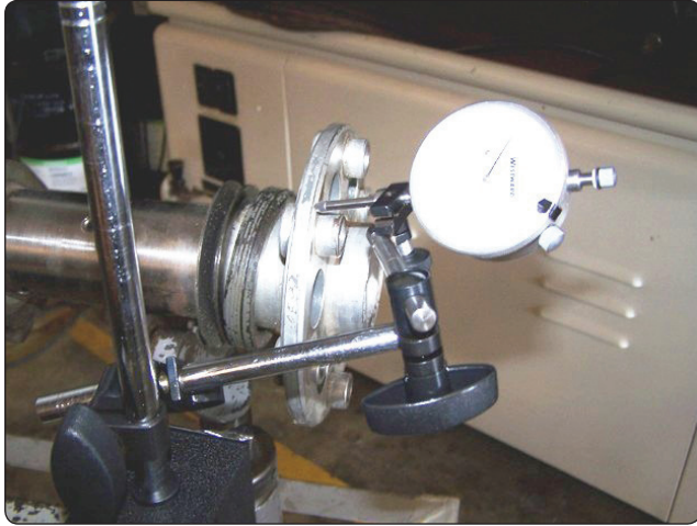
Figure 10-10. Checking crankshaft runout.
