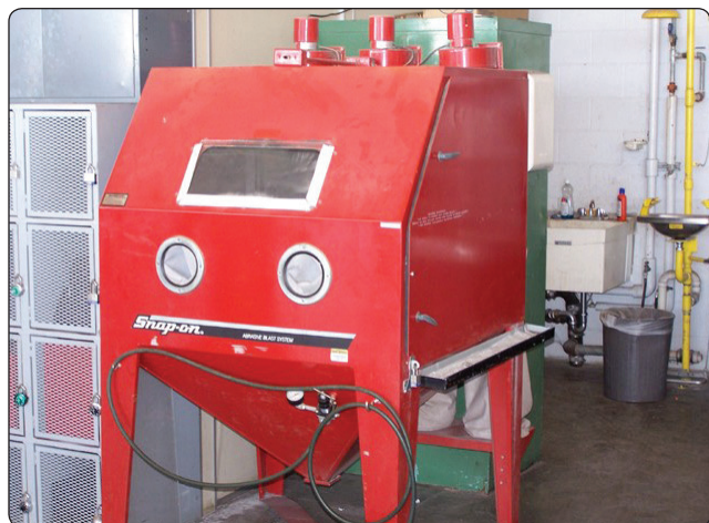
Figure 10-4. Grit-blasting machine.
