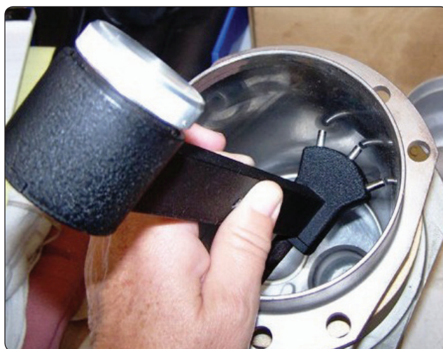
Figure 10-5. A cylinder bore gauge.
