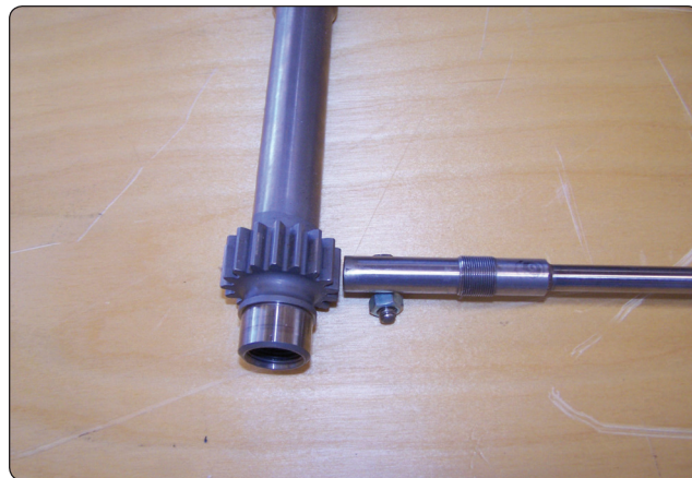
Figure 10-79. Magnetic pickup and gear.
