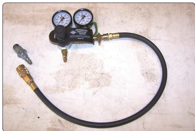
Figure 10-54. Compression tester and adapter.
