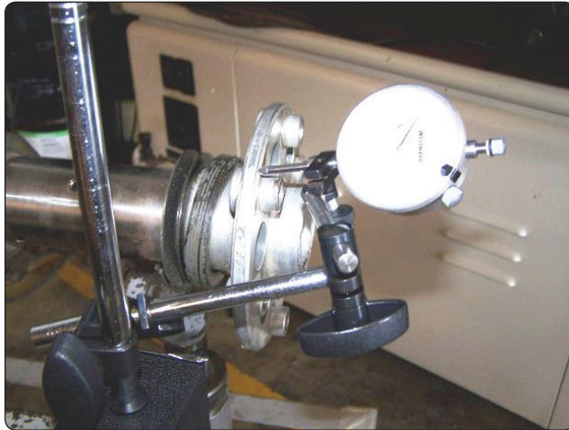
Figure 10-10. Checking crankshaft runout.
