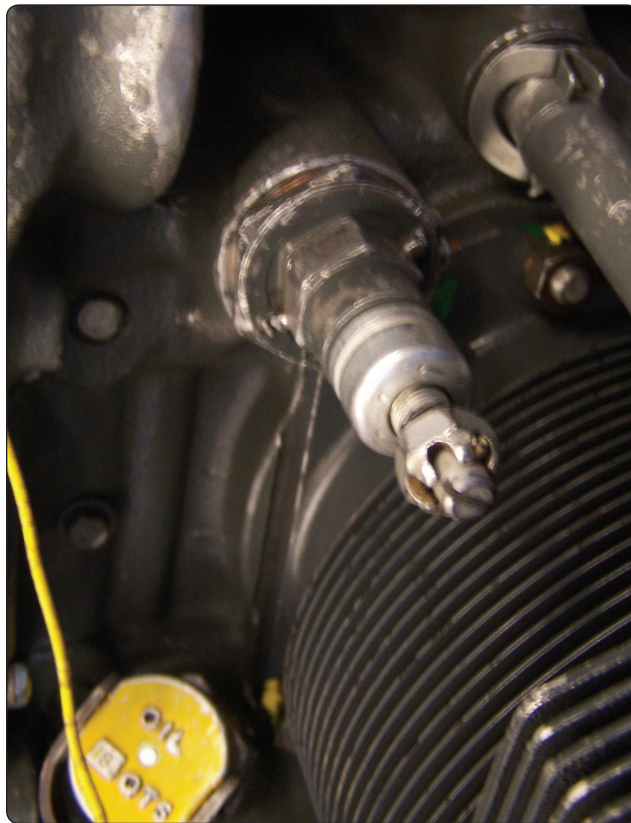
Figure 6-10. Oil pressure adjustment screw.
