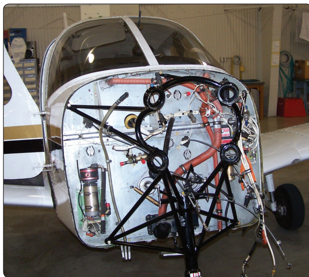
Figure 8-2. Typical firewall with components mounted on it.
