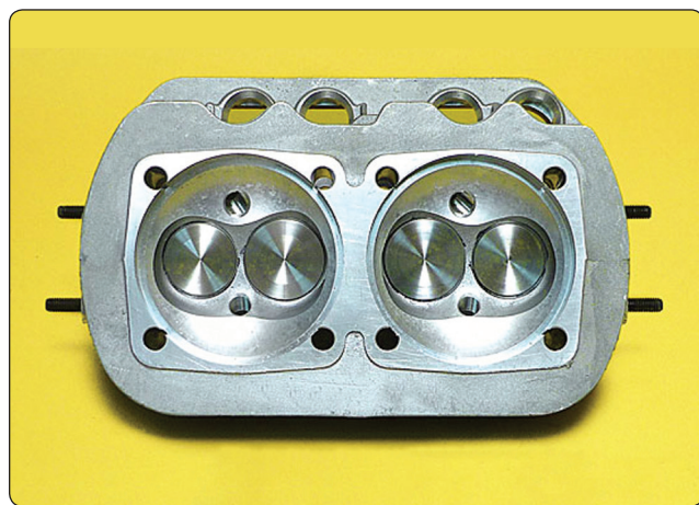
Figure 11-22. Hemispherical combustion chamber within the Revmaster R-2300 Heads.
