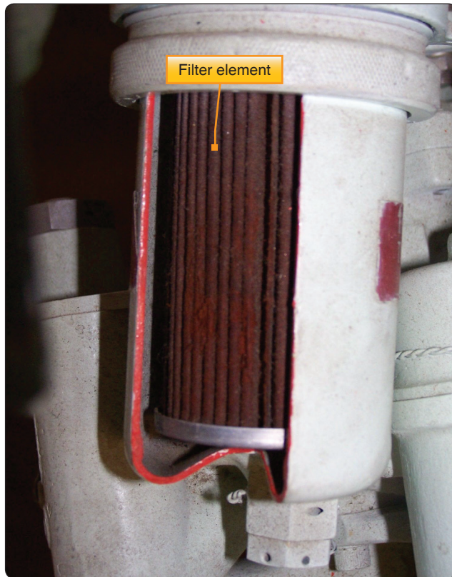
Figure 6-35. Turbine oil filter paper element.
