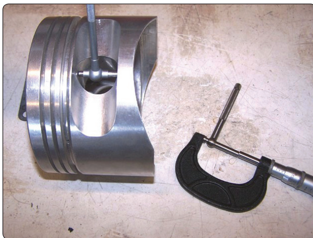
Figure 10-12. Telescoping gauges and micrometer combination.
