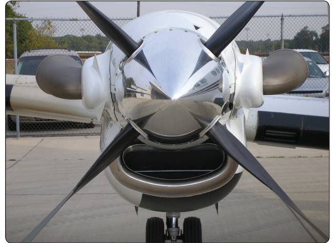
Figure 3-32. An example of a ducted arrangement on a turboprop engine.
