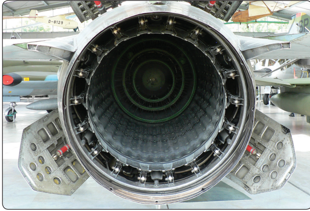
Figure 3-50. An example of a variable area exhaust nozzle used to increase or decrease exhaust flow during afterburn.
