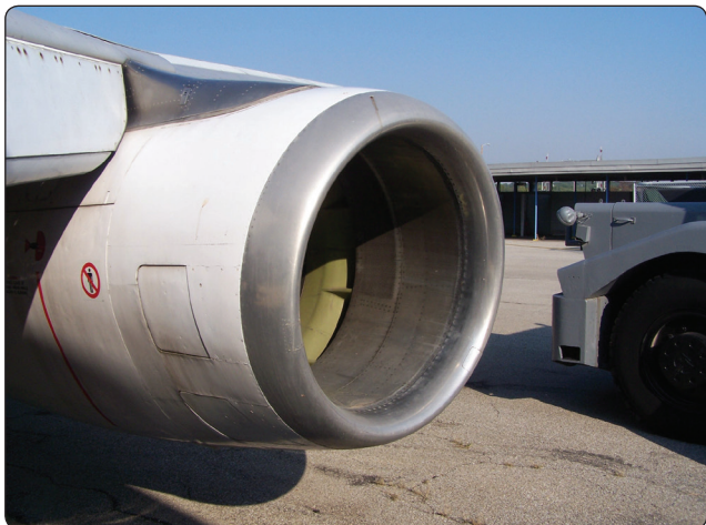
Figure 3-34. A typical turbofan intake section.
