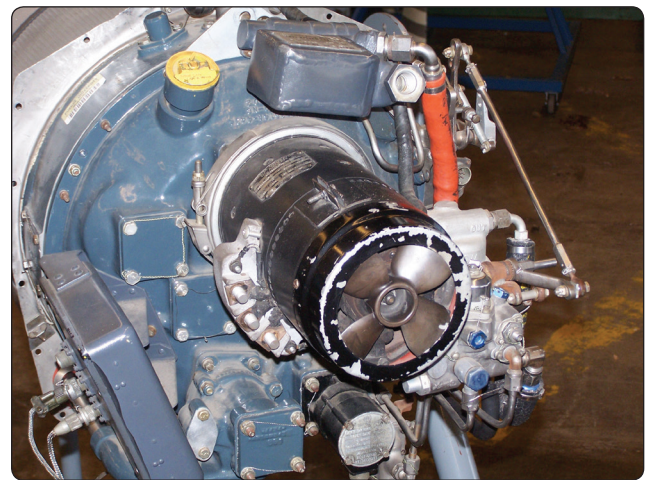
Figure 1-45. Typical turboprop accessory case.
