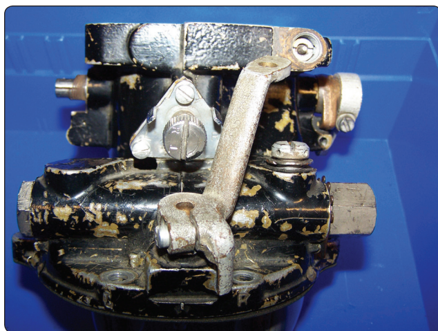
Figure 2-46. Idle mixture adjustment for carburetor.
