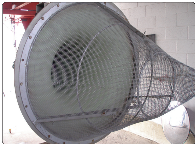
Figure 3-30. A bellmouth inlet used during system tests.
