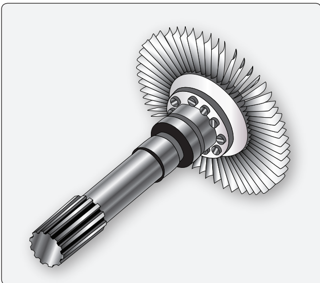
Figure 1-64. Rotor elements of the turbine assembly.
