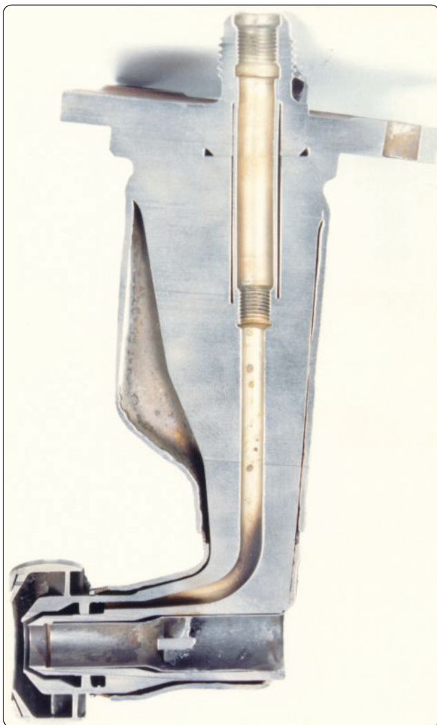
Figure 2-64. Simplex airblast nozzle cutaway.
