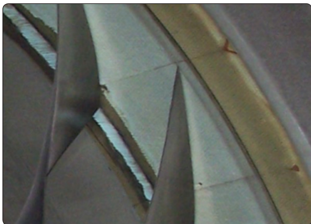
Figure 3-35. Rubber stripping inside a turbofan engine inlet allows for friction for short periods of time during changes in the flightpath.
