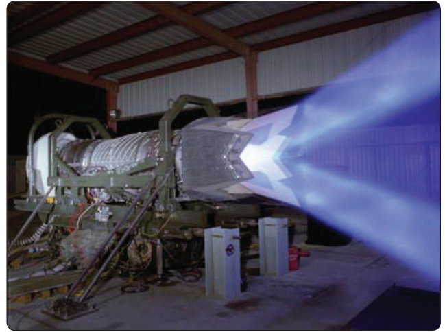
Figure 3-51. A pilot can direct thrust via the vectoring nozzle 20° up or down to increase flight maneuverability.
