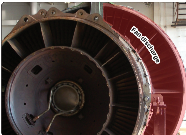
Figure 3-37. Air from the fan exhaust can be discharged overboard through short ducts directly behind the fan.
