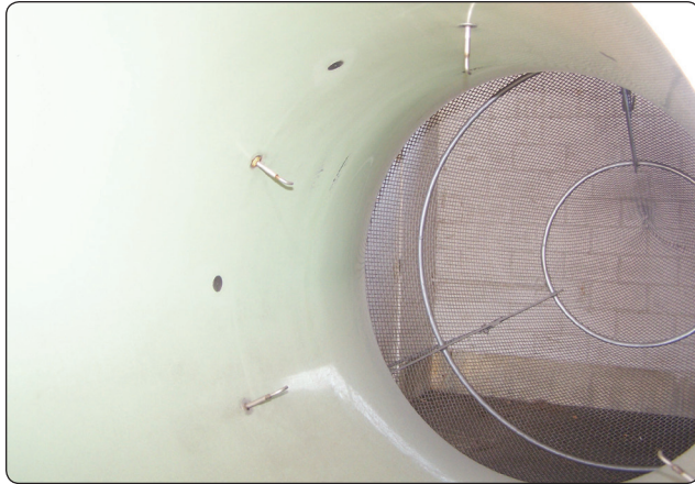
Figure 3-31. Probes within a bellmouth inlet used to measure intake temperature and pressure.
