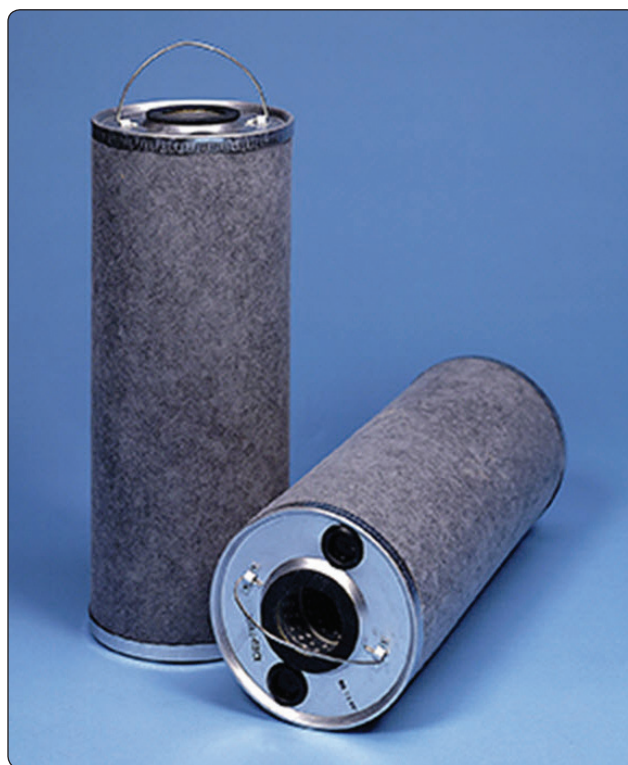
Figure 14-95. Clay filter elements remove surfactants. They are used in the fuel dispensing system before fuel enters the aircraft.
