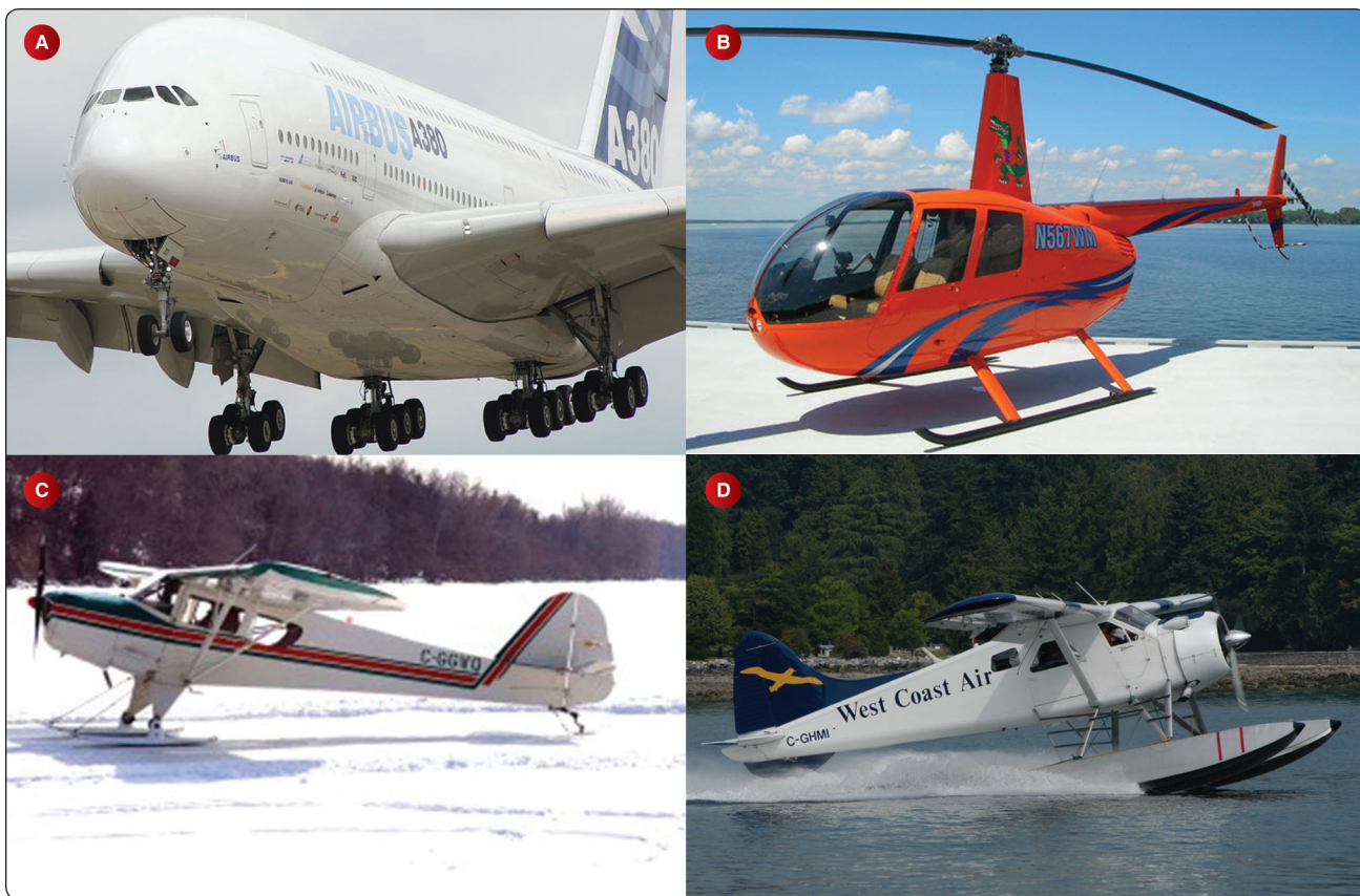
Figure 13-1. Basic landing gear types include those with wheels (a), skids (b), skis (c), and floats or pontoons (d).
