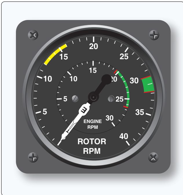
Figure 10-57. A helicopter tachometer with engine rpm, rotor rpm, and slippage indications.
