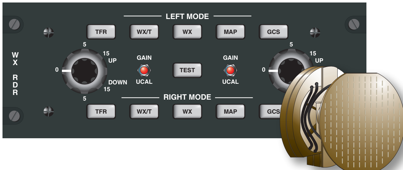
Figure 11-143. A typical on-board weather radar system for a high performance aircraft uses a nose-mounted antenna that gimbals. It is usually controlled by the inertial reference system (IRS) to automatically adjust for attitude changes during maneuvers so that the radar remains aimed at the desired weather target. The pilot may also adjust the angle and sweep manually as well as the gain. A dual mode control panel allows separate control and display on the left or right HSI or navigational display.
