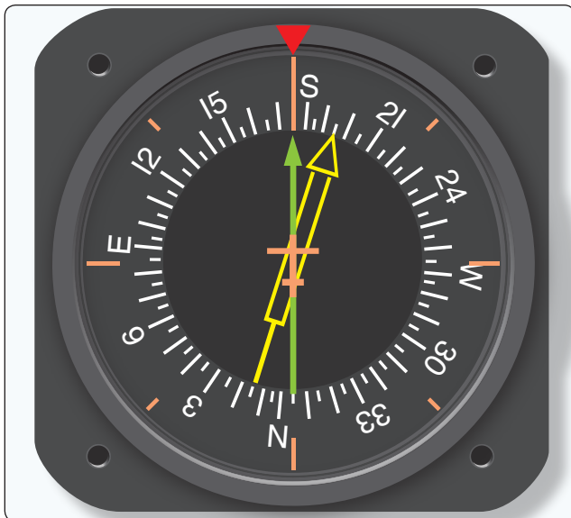
Figure 10-85. A radio magnetic indicator (RMI) combines a slaved gyro heading indication (red triangle at top of gauge) with magnetic bearing information to a VOR station (solid pointer) and an ADF station (hollow pointer).
