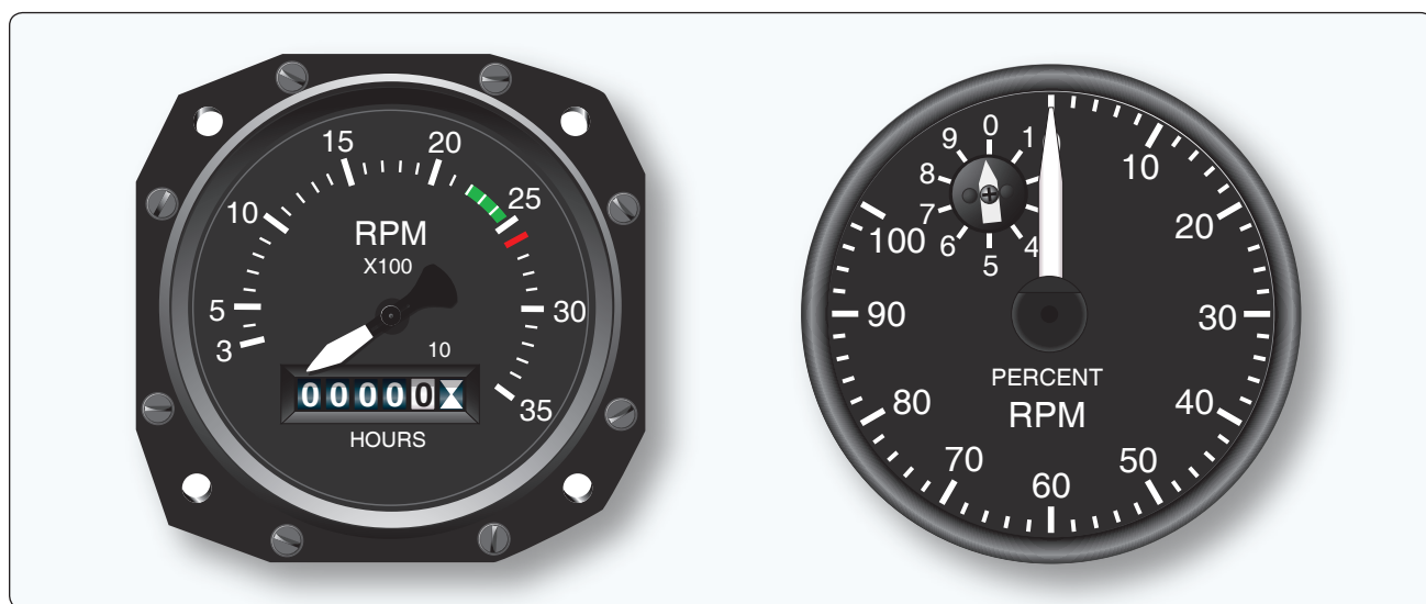
Figure 10-52. A tachometer for a reciprocating engine is calibrated in rpm. A tachometer for a turbine engine is calculated in percent of rpm.
