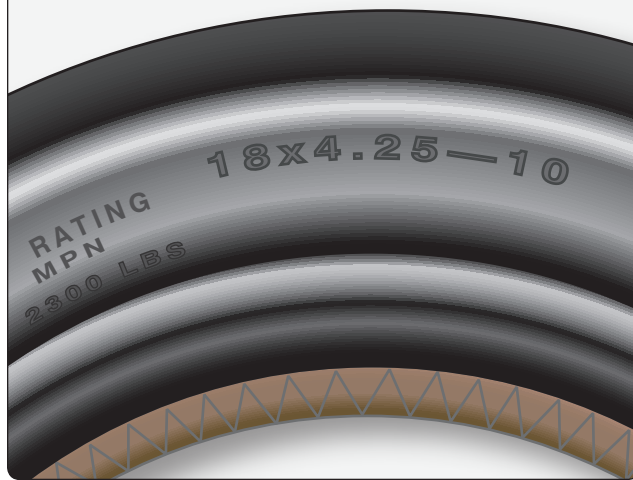
Figure 13-127. A Type VIII or three-part nomenclature tire is identified by 3 parameters: overall diameter, section width, and rim diameter. They are arranged in that order with the first two separated by an "X" and the second two separated by a "-." For example: 18 X 4.25-10 designates a tire that is 18 inches in diameter with a 4.25-inch section width to be mounted on a 10-inch wheel rim.
