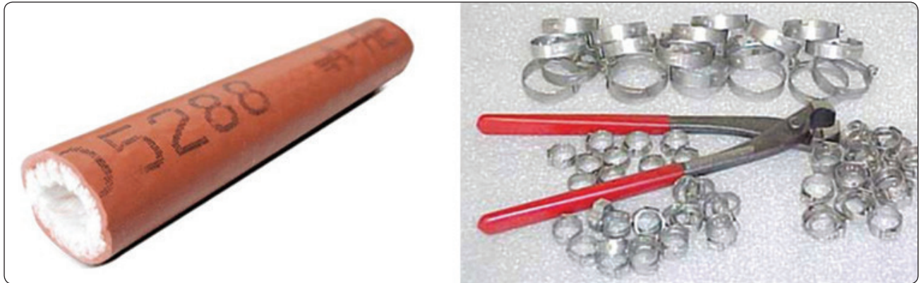
Figure 14-36. Exterior fuel hose wrap that protects from fire, as well as abrasion, shown with the clamps and pliers used to install it.
