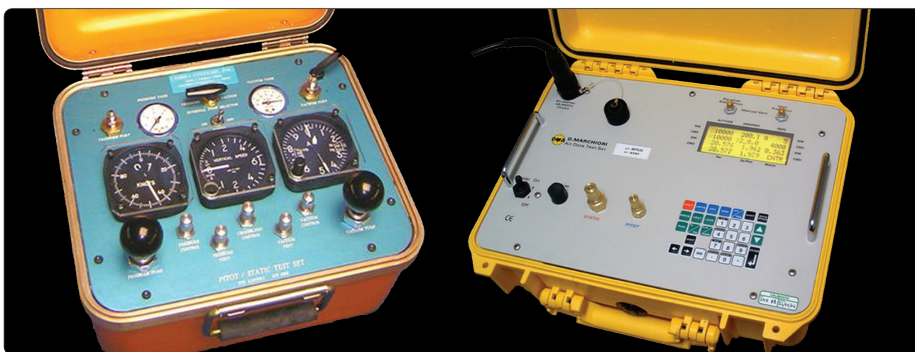
Figure 10-138. An analog pitot-static system test unit (left) and a digital pitot static test unit (right).
