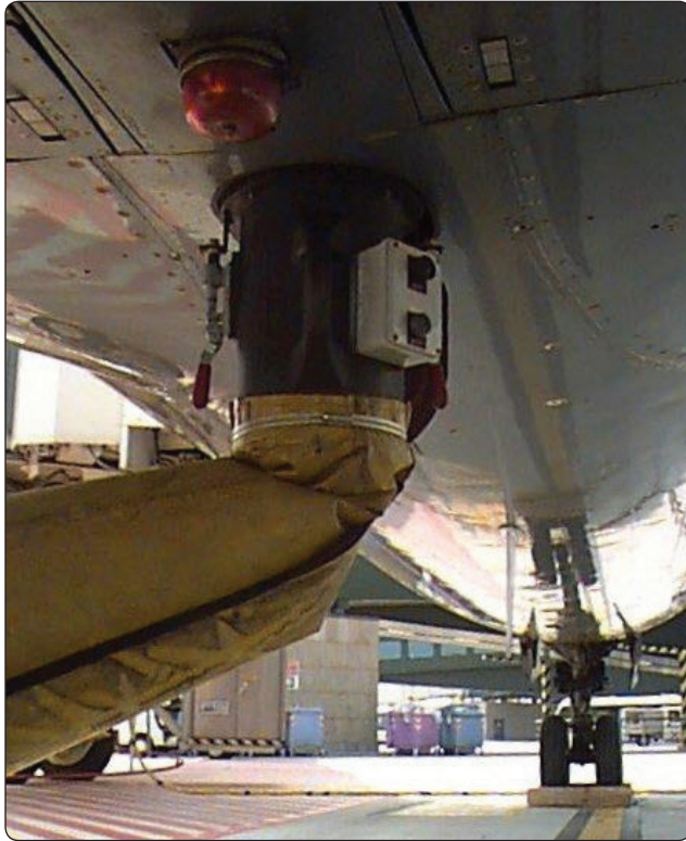
Figure 16-61. A duct hose installed on this airliner distributes hot or cold air from a ground-based source throughout the cabin using the aircraft's own air distribution system ducting.
