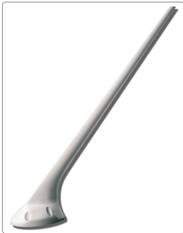
Figure 11-90. Many antenna are canted for better reception.
