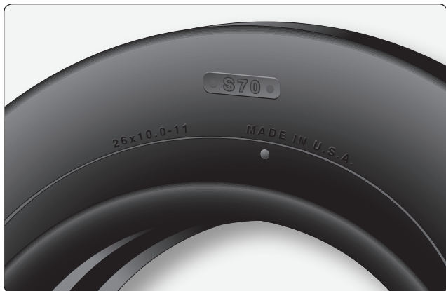
Figure 13-132. A sidewall vent marked by a colored dot must be kept free from obstruction to allow trapped air or nitrogen to escape from the carcass plies of the tire.
