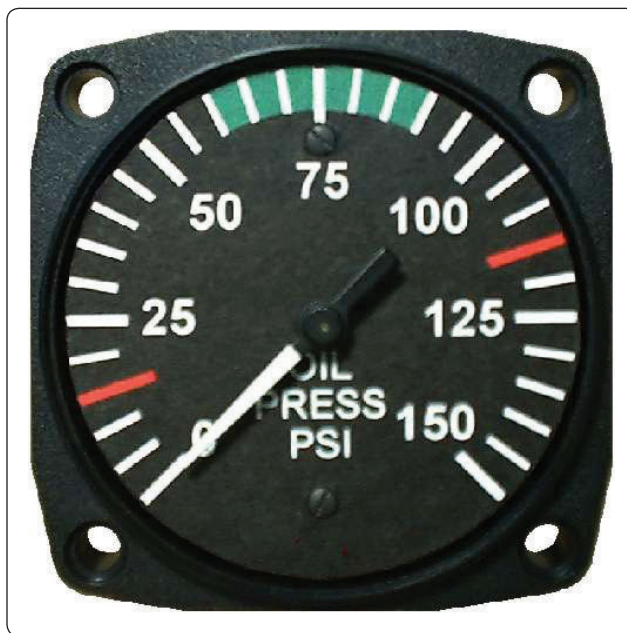
Figure 10-13. An analog oil pressure gauge is driven by a Bourdon tube. Oil pressure is vital to engine health and must be monitored by the pilot.
