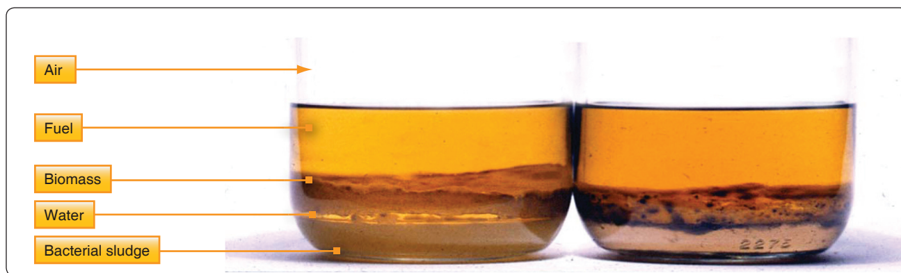
Figure 14-96. This fuel-water sample has microbial growth at the interface of the two liquids.
