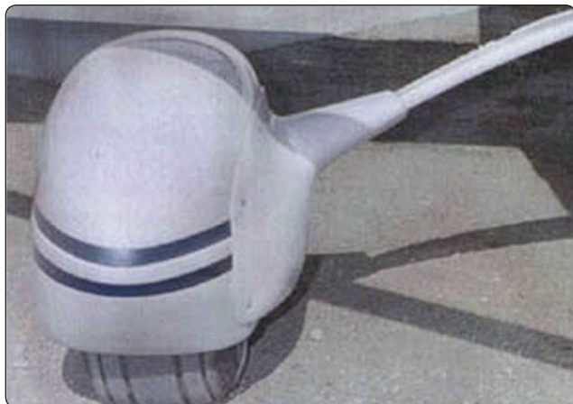
Figure 13-11. Wheel fairings, or pants, and low profile struts reduce parasite drag on fixed gear aircraft.
