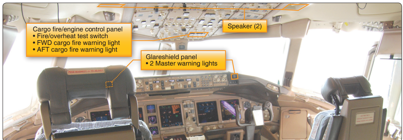
Figure 17-18. Cargo fire detection warning.
