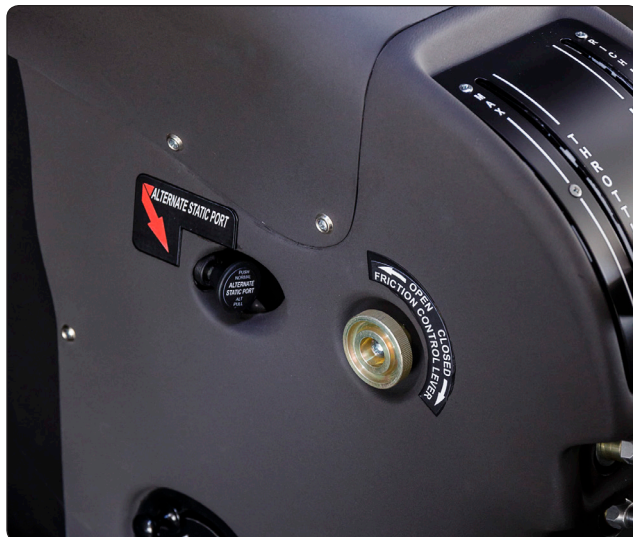
Figure 10-25. On unpressurized aircraft, an alternate source of static air is cabin air.
