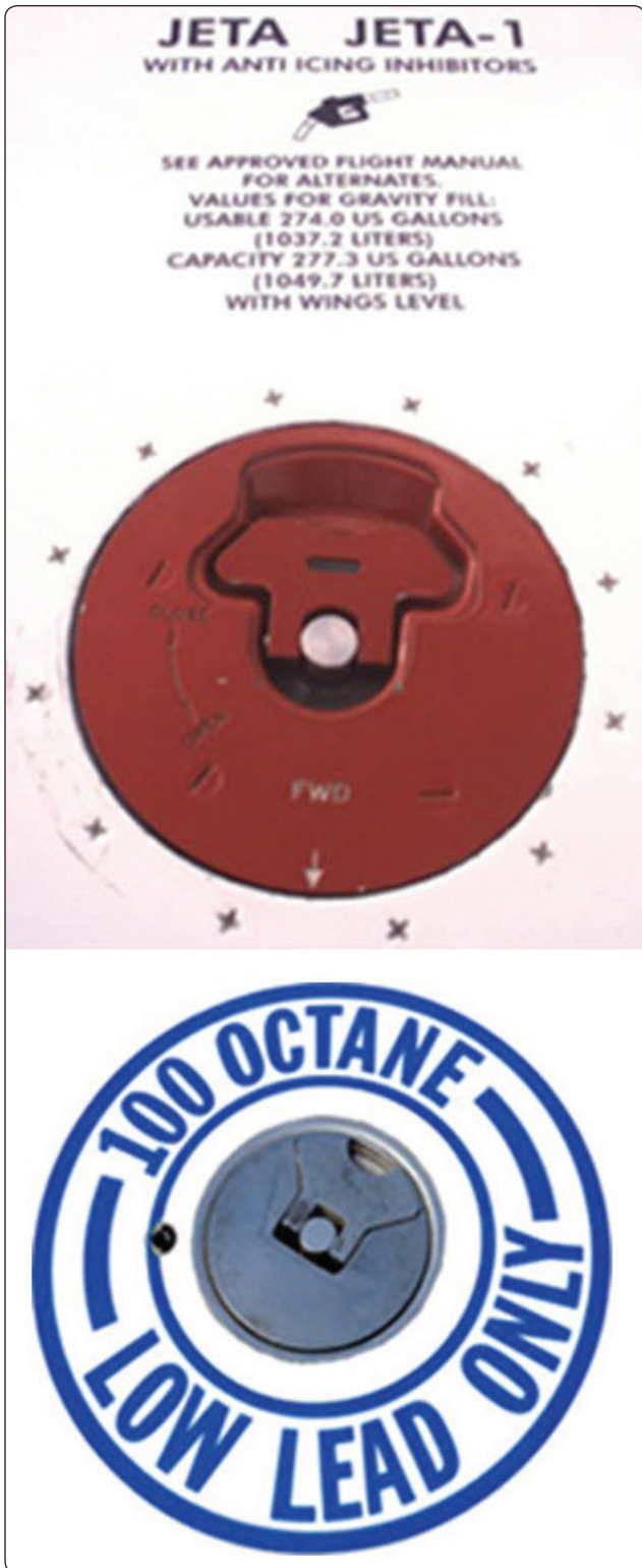
Figure 14-97. All entry points of fuel into the aircraft are marked with the type of fuel to be used. Never introduce any other fuel into the aircraft other than that which is specified.
