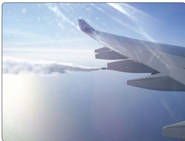
Figure 14-3. Fuel being jettisoned free of the airframe on a transport category aircraft.
