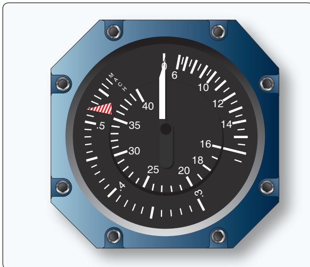
Figure 10-46. A combination Mach/airspeed indicator shows airspeed with a white pointer and Mach number with a red and white striped pointer. Each pointer is driven by separate internal mechanisms.
