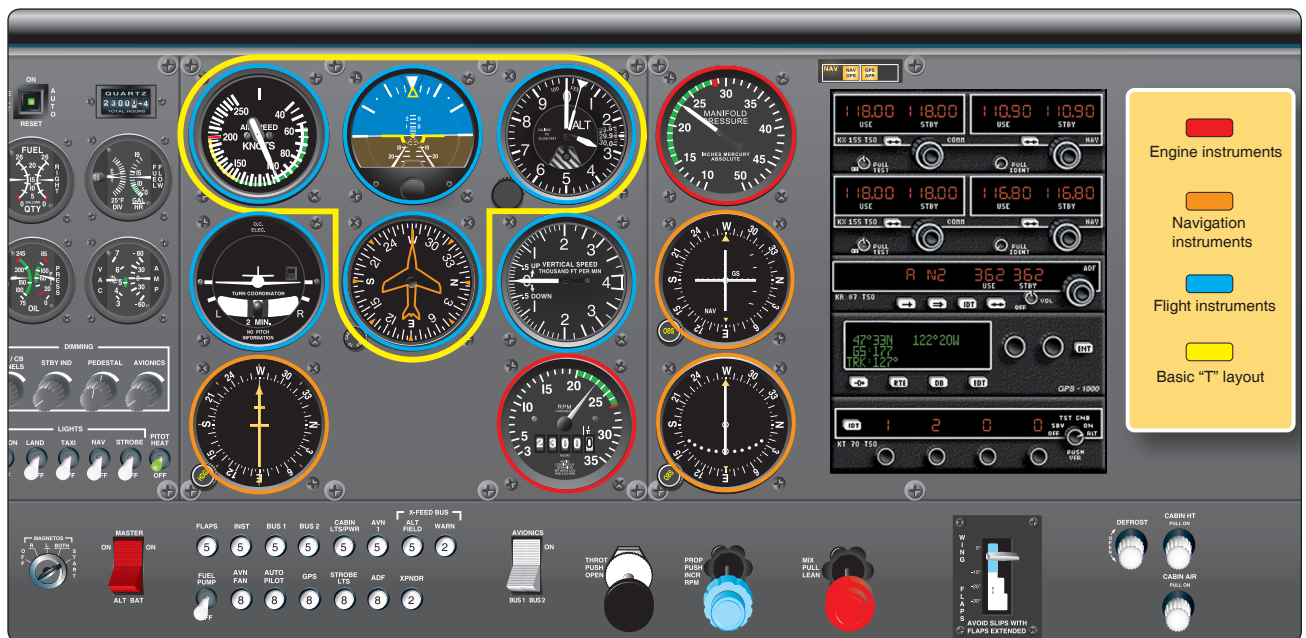
Figure 10-134. Flight instruments directly in front of the pilot, engine instruments to the left and right, and navigation instruments and radios primarily to the right, which is the center of the instrument panel. This arrangement is commonly on light aircraft to be flown by a single pilot.
