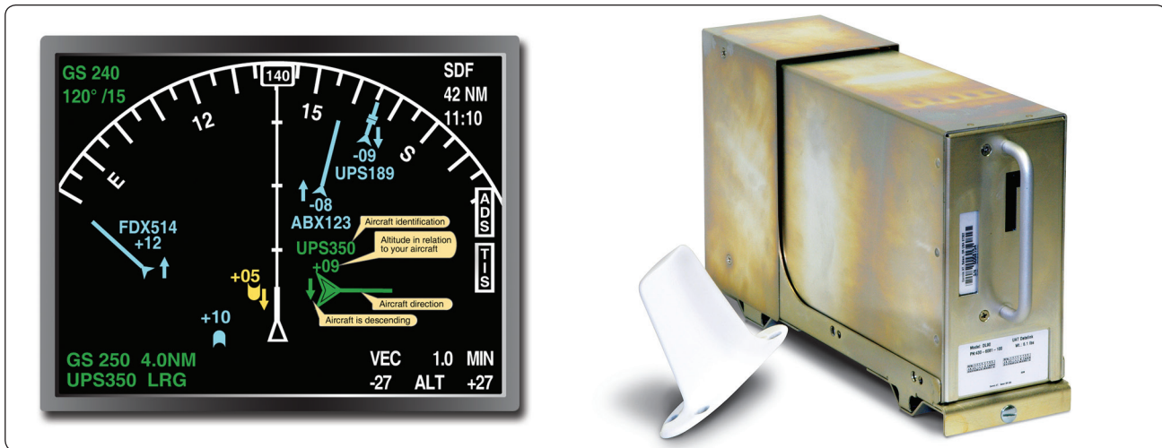
Figure 11-137. A cockpit display of ADS-B generated targets (left) and an ADS-B airborne receiver with antenna (right).
