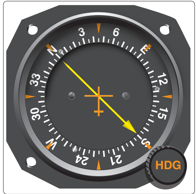
Figure 11-104. A movable card ADF indicator can be rotated to put the aircraft's heading at the top of the scale. The pointer then points to the magnetic bearing the ADF broadcast antenna.
