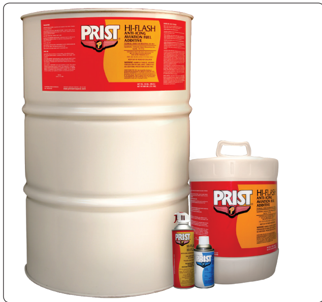
Figure 14-9. Fuel anti-icing products, such as Prist®, act as antifreeze for any free water in aircraft fuel. They dissolve in the water and lower its freezing point to prevent ice crystals from disrupting fuel flow.
