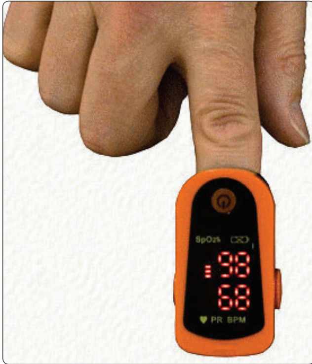
Figure 16-5. A portable pulse-type oximeter displays percentage of oxygen saturation of the blood and heart rate. Pilots can adjust oxygen supply levels to maintain saturation and avoid hypoxia.
