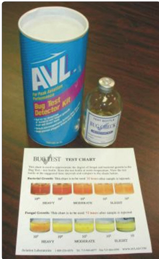
Figure 14-100. Fuel bug test kits identify the level of bacteria and fungus present in a fuel load by comparing the color of a treated sample with a color chart.
