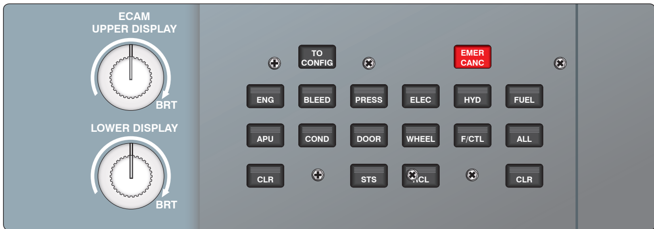
Figure 10-121. An ECAM display control panel.
