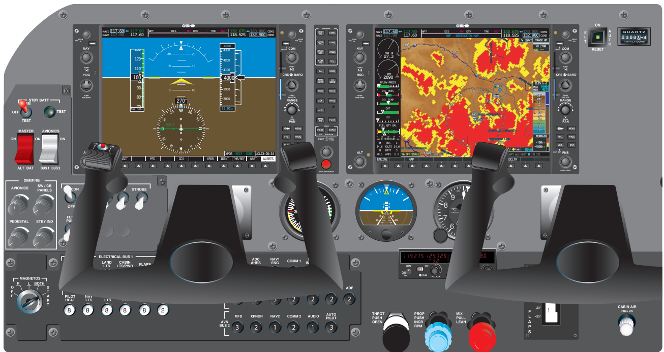
Figure 10-99. Instrumentation displayed within a glass cockpit using an attitude heading and reference system (AHRS) computer.
