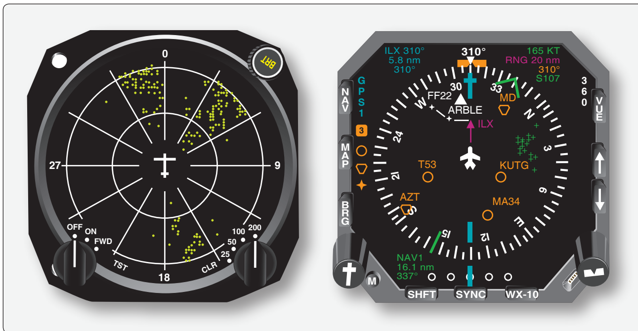
Figure 11-145. A dedicated stormscope lightning detector display (left), and an electronic navigational display with lightning strikes overlaid in the form of green “plus” signs (right).
