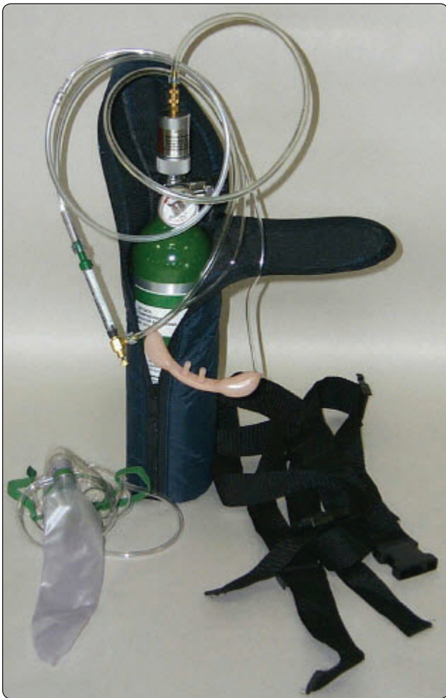
Figure 16-11. A typical portable gaseous oxygen cylinder complete with valve, pressure gauge, regulator/reducer, hose, adjustable flow indicator, and rebreather cannula. A padded carrying case/bag can be strapped to the back of a seat in the cabin to meet certification and testing specifications.
