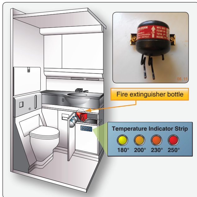
Figure 17-24. Lavatory fire extinguishing bottle.
