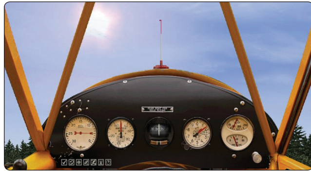
Figure 14-66. The fuel quantity indicator on this Piper Cub is a float attached to a rod that protrudes through the fuel cap.
