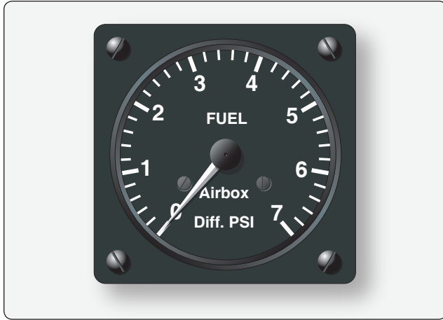
Figure 14-84. A differential fuel pressure gauge used on complex and high-performance reciprocating-engine aircraft compares the fuel inlet pressure to the air inlet pressure at the fuel metering device.
