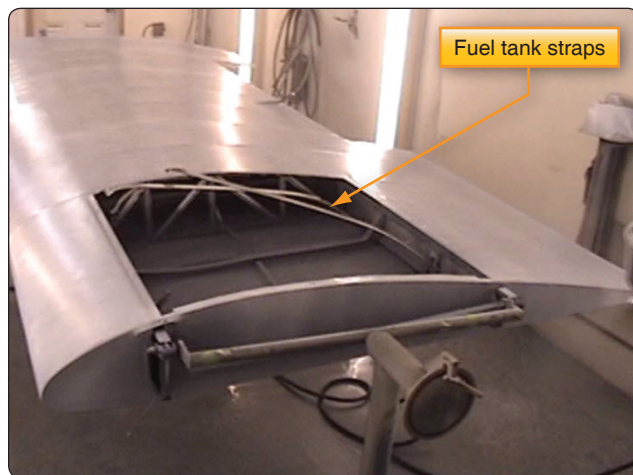
Figure 14-28. A fuel tank bay in the root of a light aircraft wing on a stand in a paint booth. Padded straps hold the fuel tank securely in the structure.
