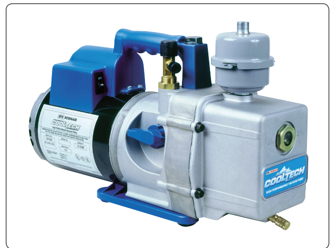
Figure 16-91. A vacuum pump is used to lower the pressure in the vapor cycle air conditioning system. This reduces the boiling point of water in the system, which vaporizes and is drawn out by the pump.
