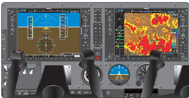
Figure 10-5. This electrically operated flat screen display instrument panel, or glass cockpit, retains an analog airspeed indicator, a gyroscope-driven artificial horizon, and an analog altimeter as a backup should electric power be lost, or a display unit fails.
