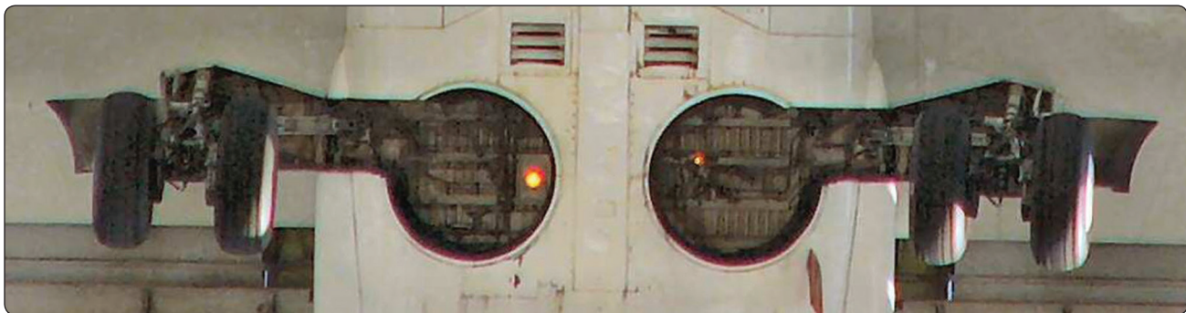
Figure 13-12. The retractable gear of a Boeing 737 fair into recesses in the fuselage. Panels attached to the landing gear provide smooth airflow over the struts. The wheel assemblies mate with seals to provide aerodynamic flow without doors.
