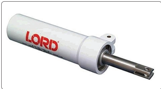
Figure 13-56. A non-hydraulic shimmy damper uses a rubber piston with lubricant that dampens via motion against the inner diameter of the unit housing.
