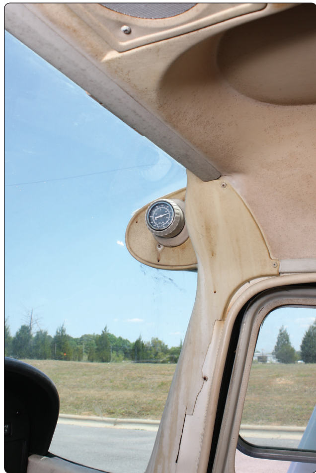
Figure 10-67. A bimetallic outside air temperature gauge and its installation on a light aircraft.
