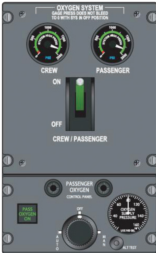
Figure 16-16. The crew can deploy passenger emergency continuous-flow oxygen masks and supply with a switch in the cockpit.
