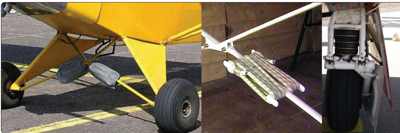
Figure 13-15. Piper Cub bungee cord landing gear transfer landing loads to the airframe (left and center). Rubber, donut-type shock transfer is used on some Mooney aircraft (right).
