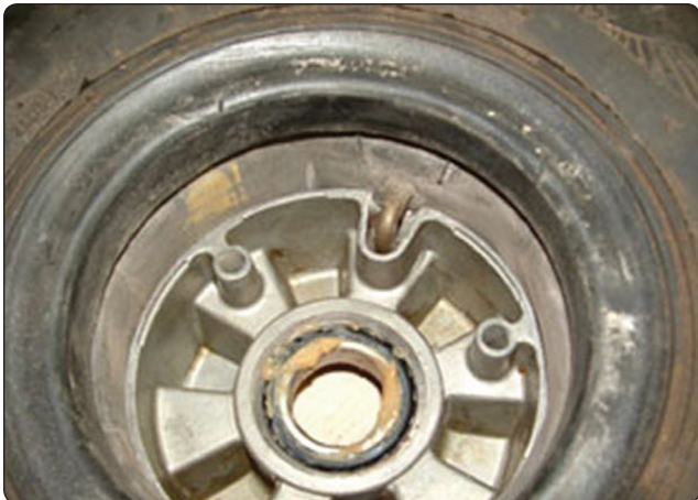
Figure 13-157. Mounting a tube type tire with the tube valve stem positioned to pass through the outboard wheel half.
