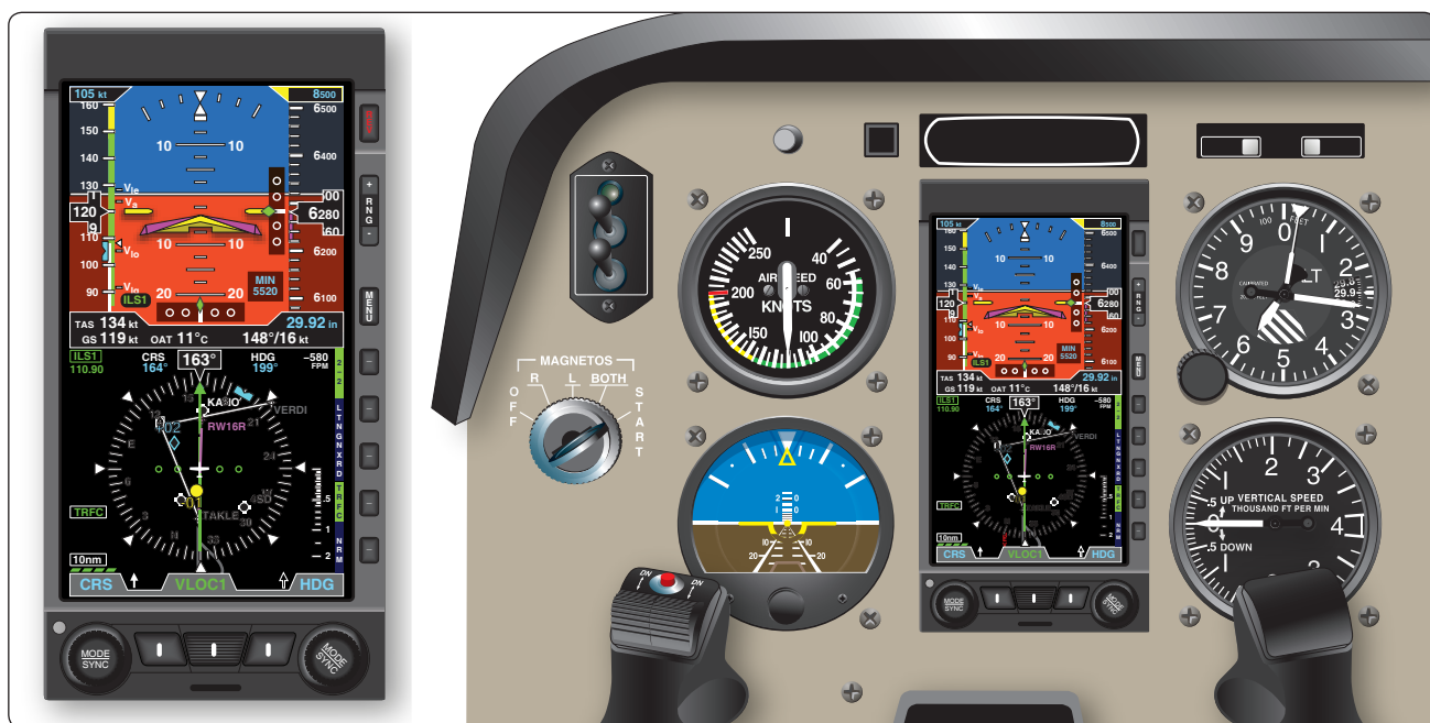
Figure 11-71. A retrofit digital data display.
