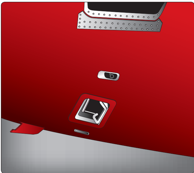
Figure 16-55. This outflow valve on a transport category aircraft is normally operated by an ac motor controlled by a pressure controller in the electronics equipment bay. A second ac motor on the valve is used when in standby mode. A dc motor also on the valve is used for manual operation.
