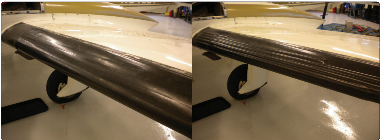
Figure 15-31. Deicing boots inflated (left) and deflated (right).
