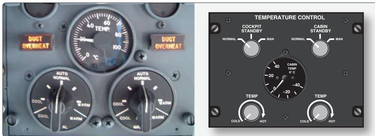
Figure 16-70. Typical temperature selectors on a transport category aircraft temperature control panel in the cockpit (left) and a business jet (right). On large aircraft, temperature selectors may be located on control panels located in a particular cabin air distribution zone.
