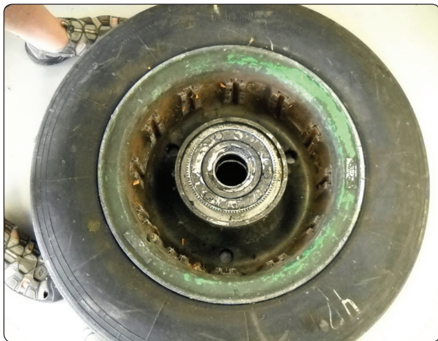
Figure 13-60. Keys on the inner wheel half of an aircraft wheel used to engage and rotate the rotors of a disc brake.
