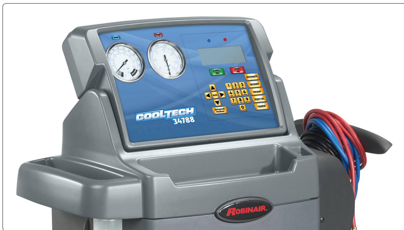
Figure 16-88. A modern refrigerant recovery/recycle/charging service unit. Electronic control of solenoid activated valves combine with a built-in system for recovering, recycling, and recharging. A built-in vacuum pump and heated refrigerant reservoir are also included.
