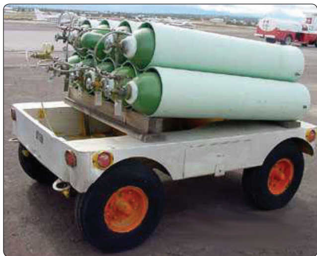
Figure 16-31. Typical oxygen servicing cart used to fill an aircraft system.
