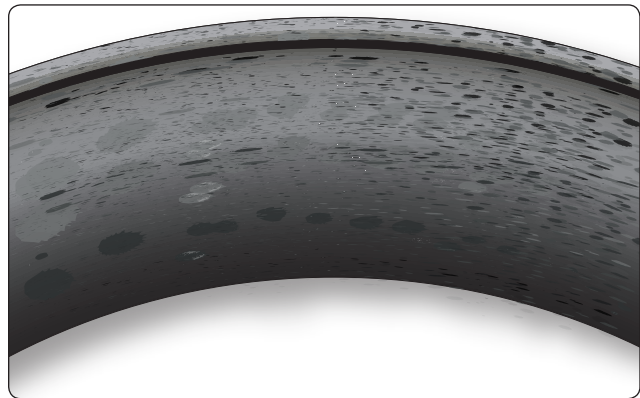
Figure 13-71. Bruising is caused by fine particle contamination possibly from a bad seal or improper maintenance of bearing cleanliness. It leaves a less than smooth surface on the bearing cup.
