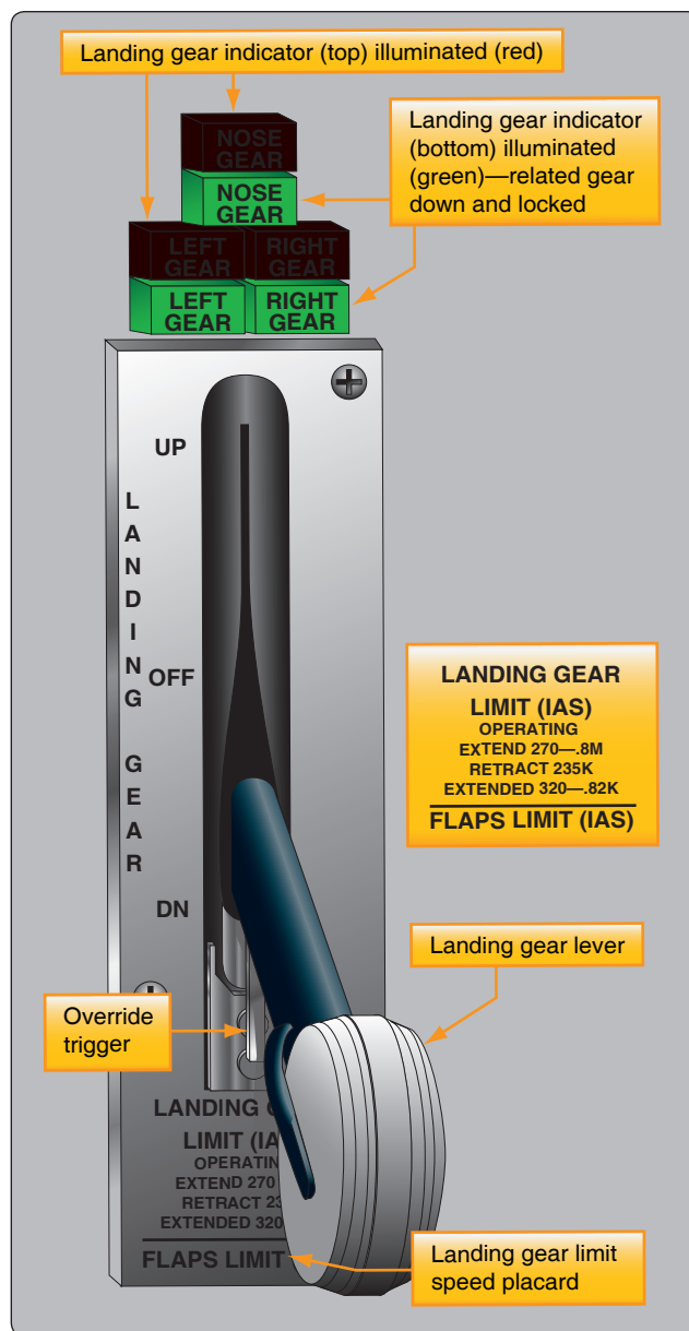
Figure 13-43. Landing gear selector panels with position indicator lights. The Boeing 737 panel illuminates red lights above the green lights when the gear is in transit.
