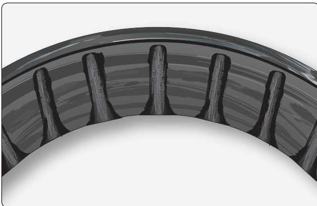
Figure 13-69. Staining and surface marks on the bearing cup that are grayish black streaks with the same spacing as the rollers are caused by water that has gotten into the bearing. It is the first stage of deeper corrosion that will follow.
