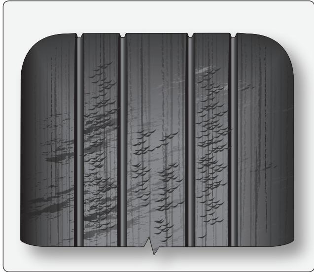
Figure 13-142. Chevron cuts in a tire are caused by operation on grooved runway surfaces. Shallow chevron cuts are permitted on aircraft tires.
