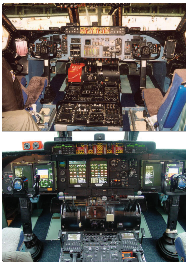
Figure 10-2. A conventional instrument panel of the C-5A Galaxy (top) and the glass cockpit of the C-5B Galaxy (bottom).
