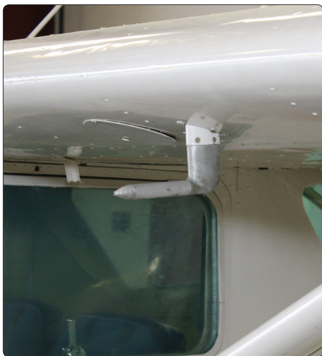
Figure 10-24. Pitot-static system heads, or pitot tubes, can be of various designs and locations on airplanes.
