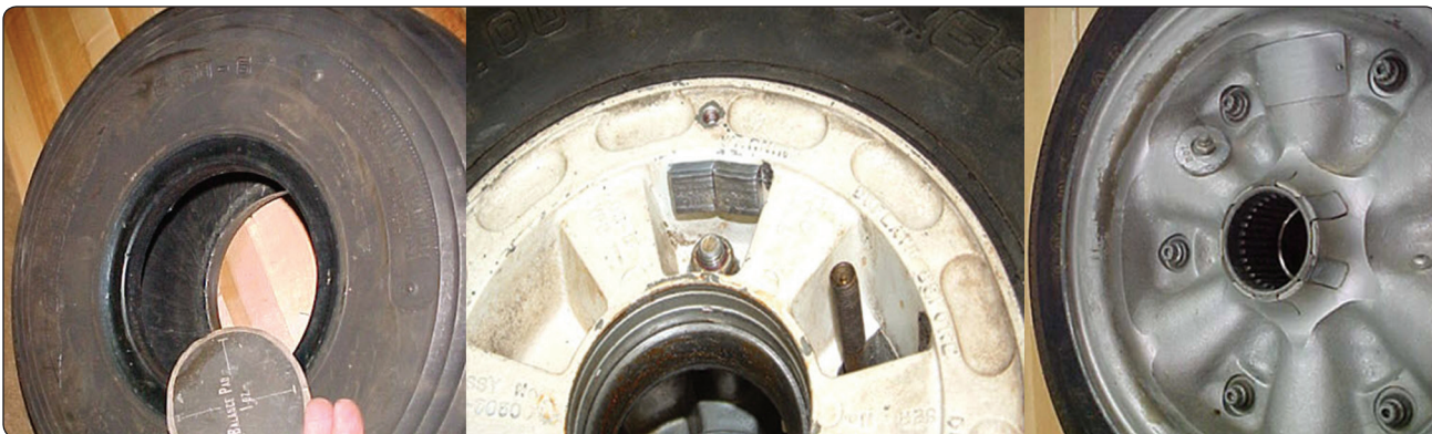
Figure 13-159. A tire balancing patch (left), adhesive wheel weights (center), and a bolted wheel weight (right) are all used to balance aircraft tire and wheel assemblies per the manufacturer's instructions.
