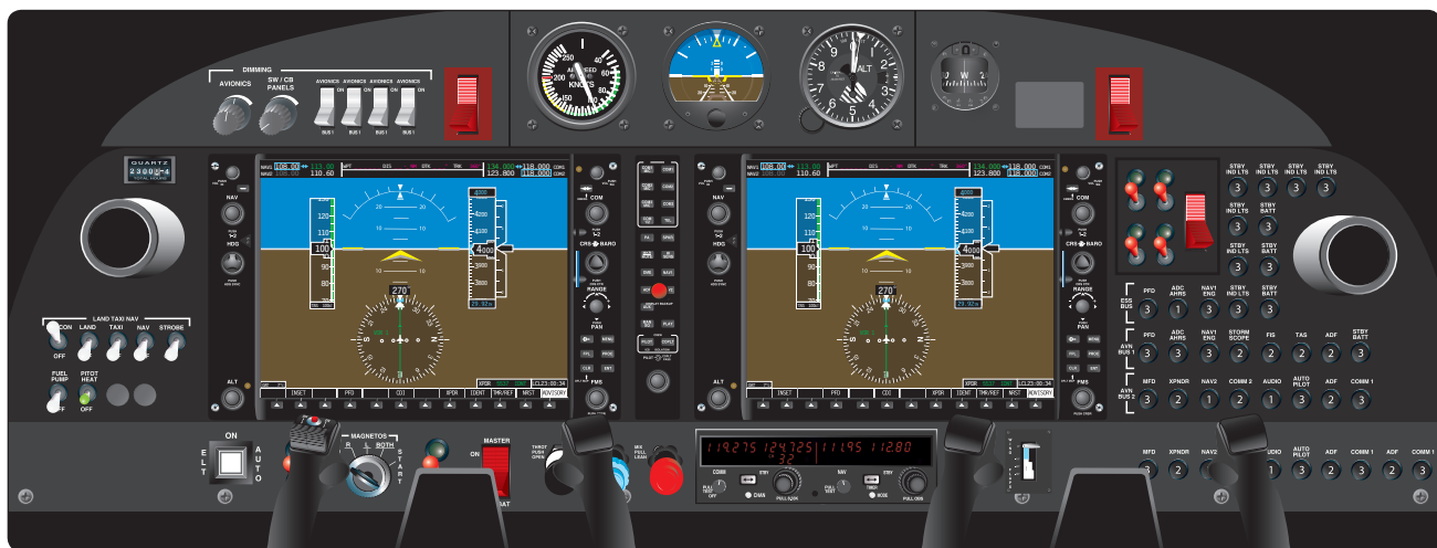
Figure 11-70. A modern glass cockpit on a general aviation aircraft. Digital data displays replace many older instruments and indicators of the past.
