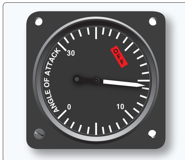
Figure 10-63. Angle of attack indicator.
