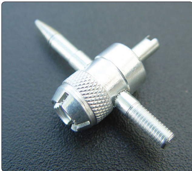
Figure 13-27. This valve tool features internal and external thread chasers, a notched valve core removal/installation tool, and a tapered end for depressing a valve core or clearing debris.
