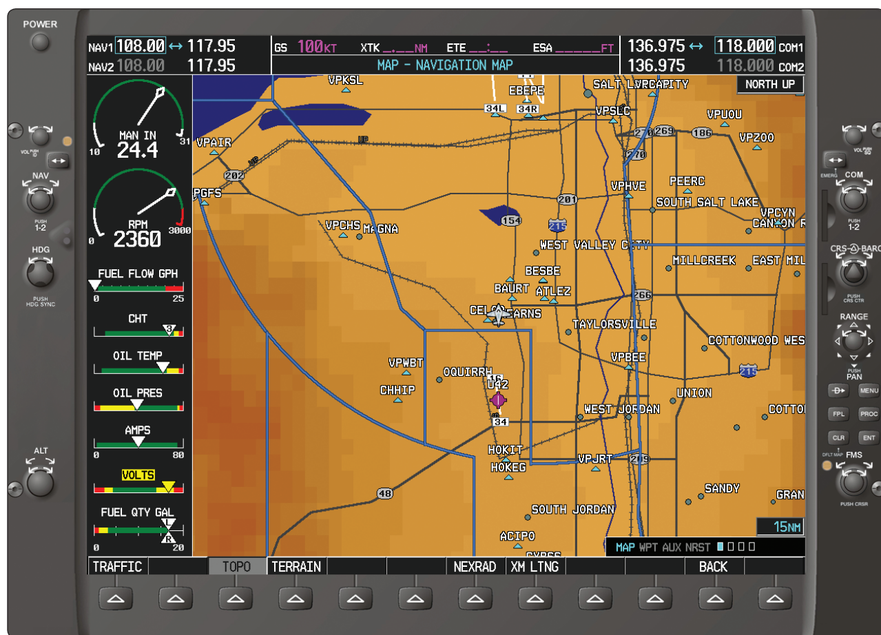
Figure 10-14. Oil pressure indication with other engine-related parameters shown in a column on the left side of this digital cockpit display panel.
