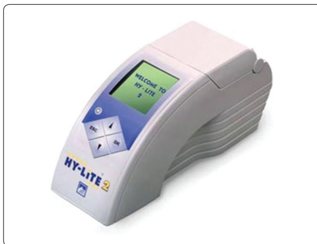
Figure 14-99. A capture solution is put into a 1 liter sample of fuel and shaken. The solution is then put into the analyzer shown to determine the level of microorganisms in the fuel.
