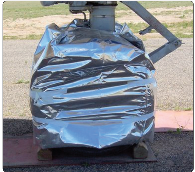
Figure 13-145. Cover tires to protect from harmful chemicals and from the elements when parked outside for long periods of time.
