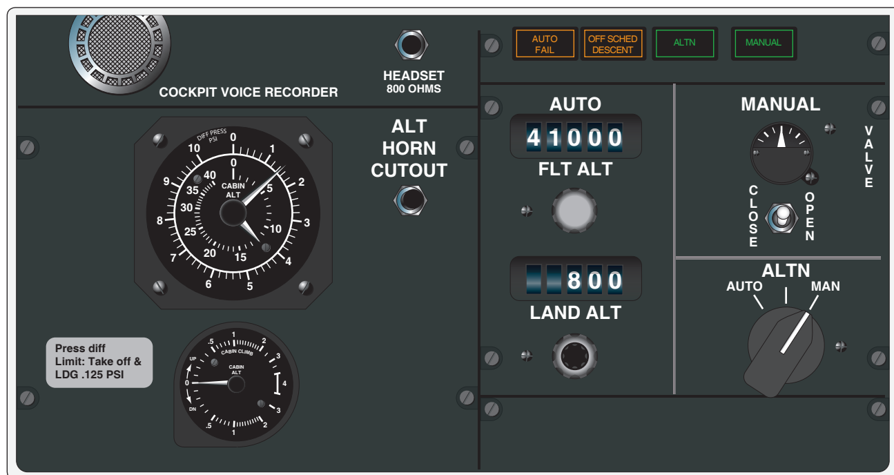
Figure 16-53. This pressurization panel from an 800 series Boeing 737 has input selections of flight altitude and landing altitude.
