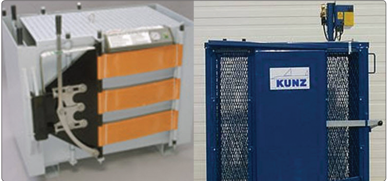
Figure 13-154. Modern tire inflation cages have been tested to withstand catastrophic failure of a tire and wheel assembly during inflation. All newly mounted tires should be inflated in such a cage.
