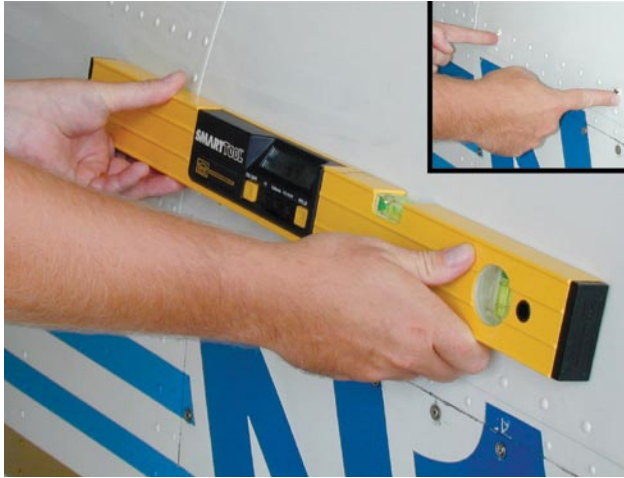
Figure 4-16. Spirit level being used on a Mooney M20.
