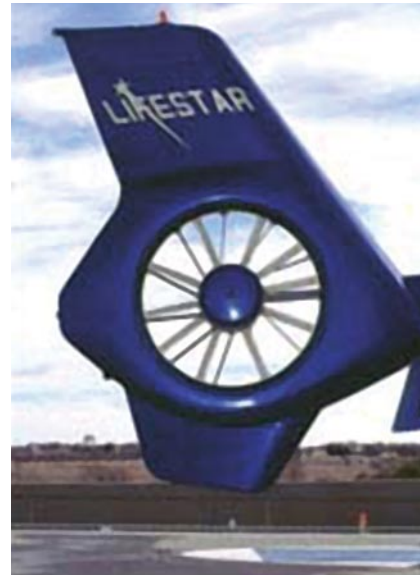
Figure 3-87. Fenestron on a Eurocopter Model 135.
