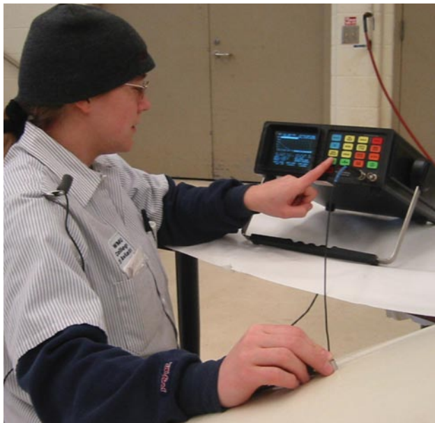
Figure 8-12. Ultrasonic inspection of a composite structure.
