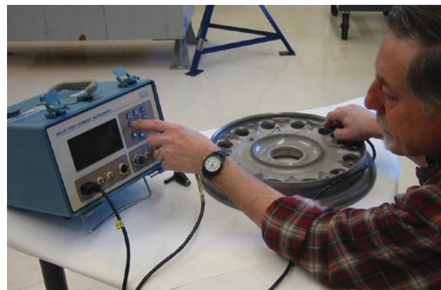
Figure 8-5. Eddy current inspection of wheel half.
