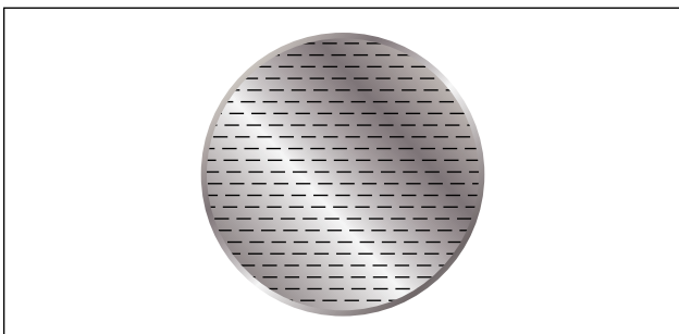
Figure 10-10. Even distribution of charge on metal disk.
