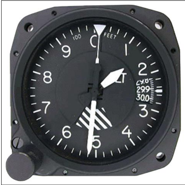
Figure 3-51. An airplane's altimeter is an aneroid barometer.
