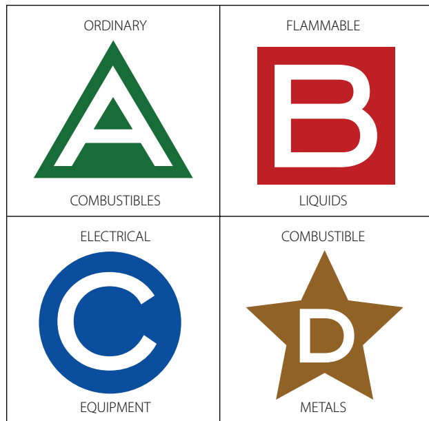
Figure 11-8. Identification of fire extinguisher type location.
