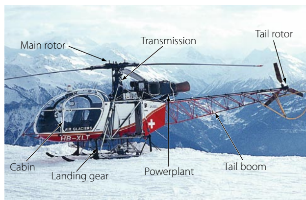
Figure 3-81. Main components of a helicopter.
