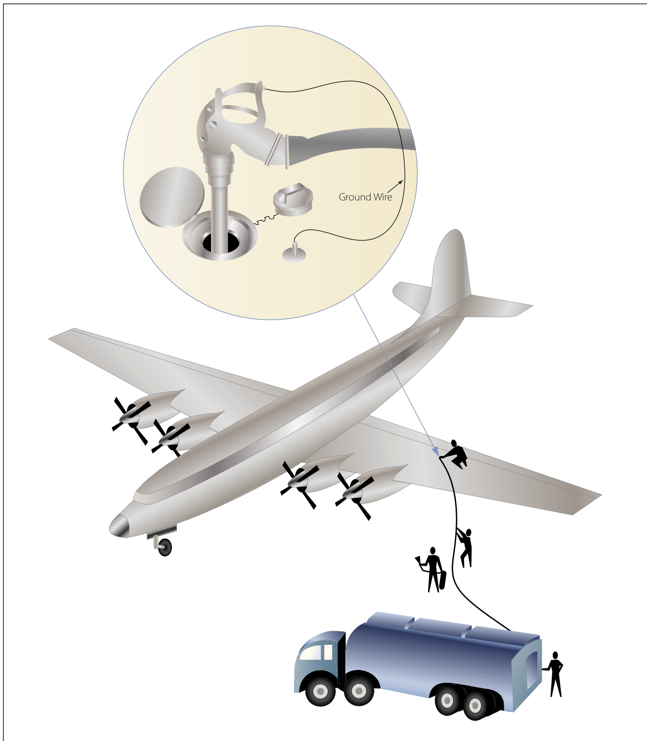
Figure 11-31. Refueling an aircraft by the over-the-wing method.
