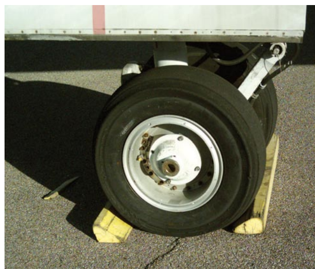
Figure 11-12. Wheels chocked fore and aft.
