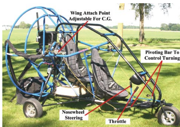
Figure 4-39. Powered parachute structure with wing attach points.
