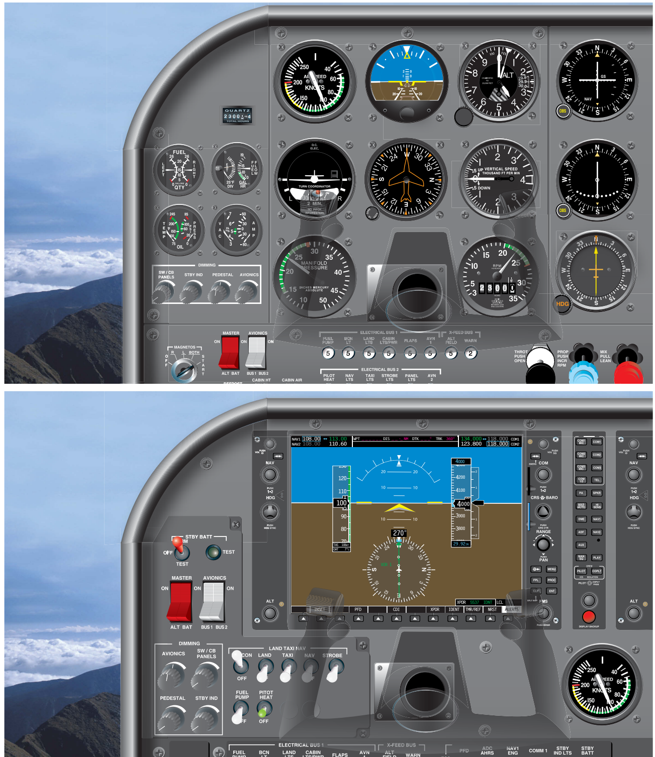
Figure 7-2. Two flight decks equipped with the same information but in two different formats: analog and digital. What are they indicating? Chances are that the analog pilot will review the top display before the bottom display. Conversely, the digitally trained pilot will review the instrument panel on the bottom first.
