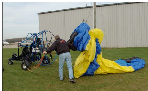
Figure 5-19. Undoing a line twist—beginning of the process.
