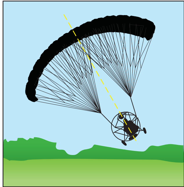
Figure 12-10. Side-to-side swinging on landing approach.
