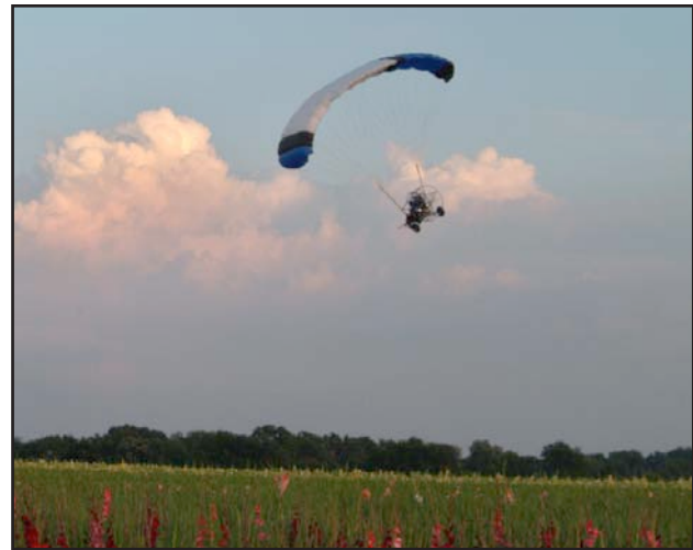
Figure 6-5. To turn, coordinate increased throttle with foot steering input.
