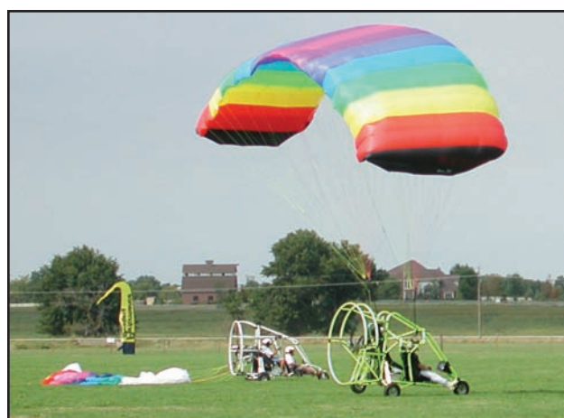
Figure 7-3. Pressurizing, or kiting, the wing.
