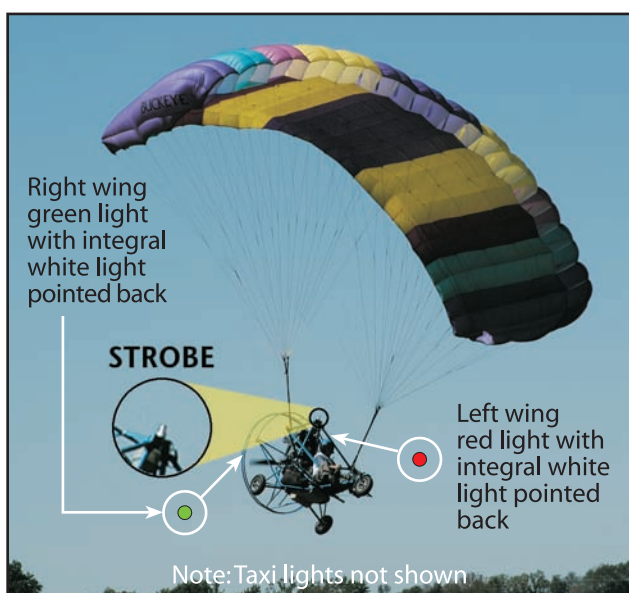
Figure 12-1. Powered parachutes must be specifically equipped for night flight.
