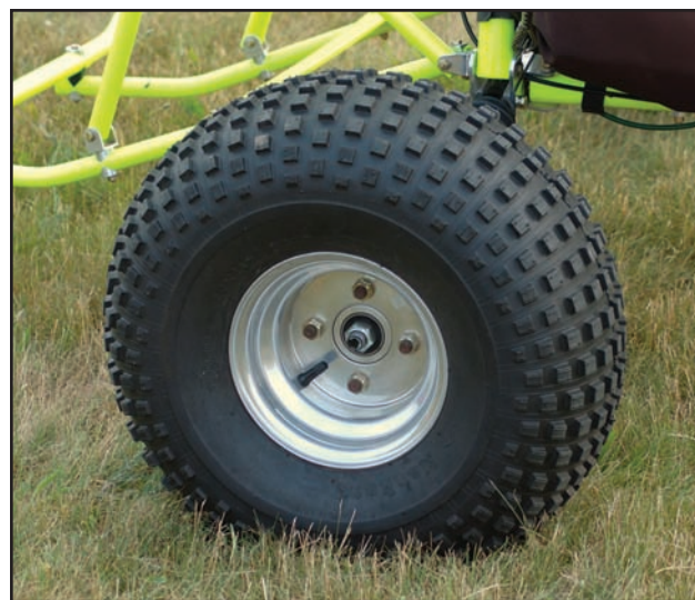
Figure 3-19. Some powered parachute tires are heavily treaded while others are smooth.
