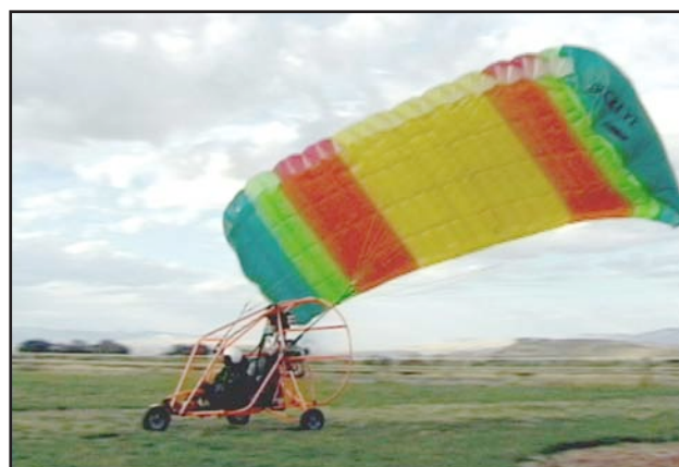
Figure 12-4. A wing lock-out.
