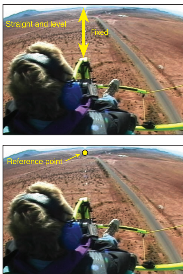
Figure 6-4. Nose reference for straight-and-level flight.
