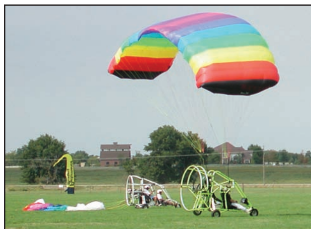
Figure 7-3. Pressurizing, or kiting, the wing.
