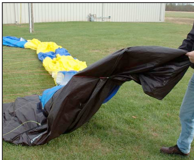
Figure 5-21. A simulated line-over.
