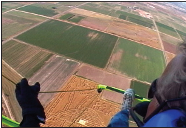
Figure 6-6. Push the foot control and pull the steering line smoothly and slowly.
