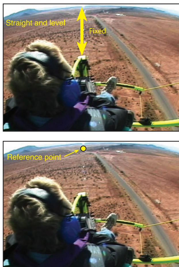
Figure 6-4. Nose reference for straight-and-level flight.
