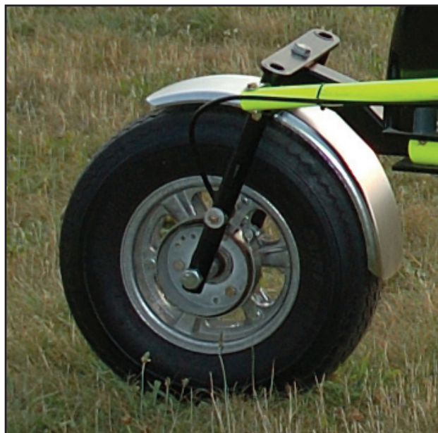
Figure 5-5. Check for proper tire inflation and that the axle bolt is secure.
