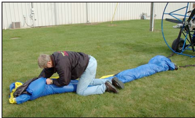
Figure 5-22. Squeeze out the air as you fold the wing for packing.
