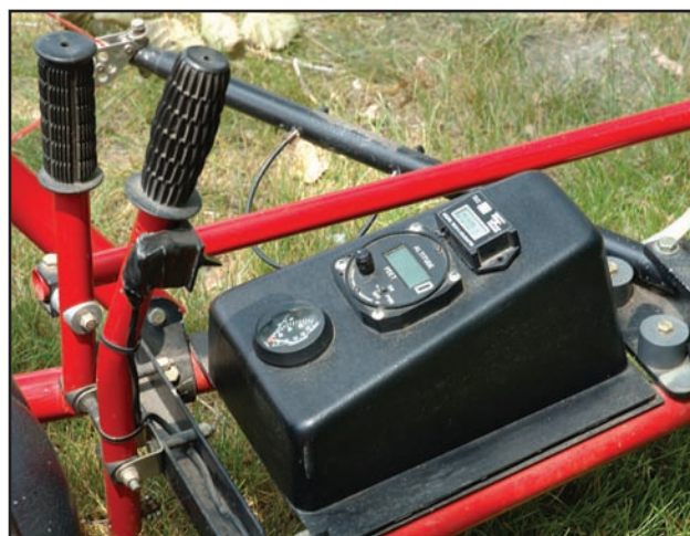
Figure 3-6. Some instrument panels will have just a few digital or analog gauges for EGT and RPM.
