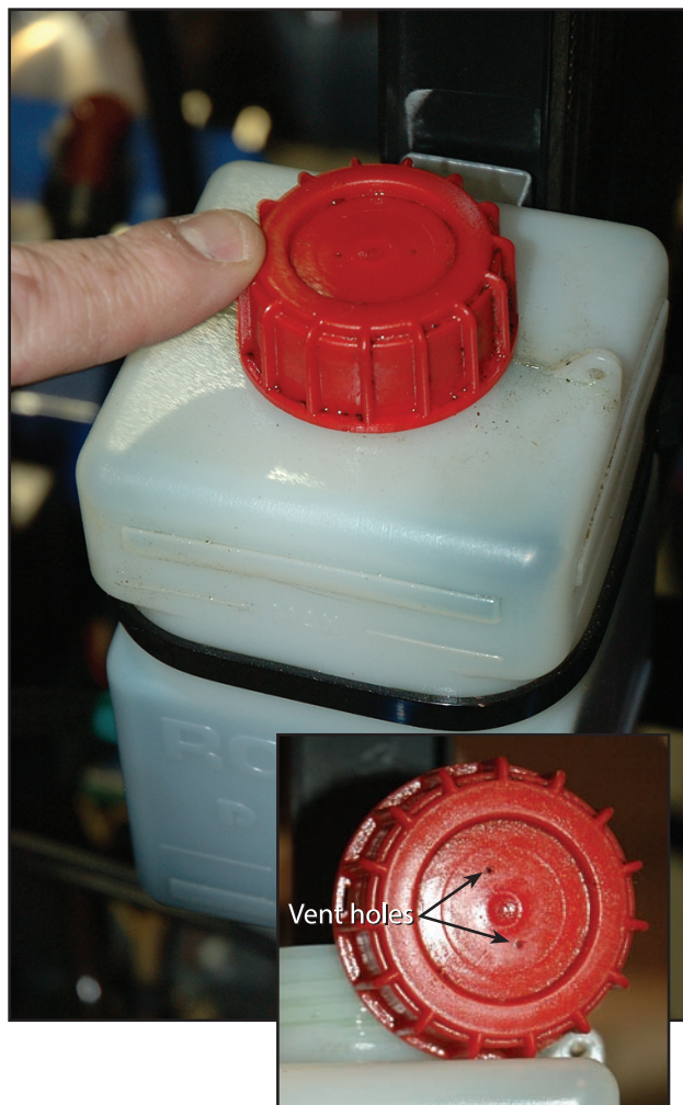
Figure 5-10. It is important to check the oil reservoir cap to make sure the vent holes are open and free of debris.
